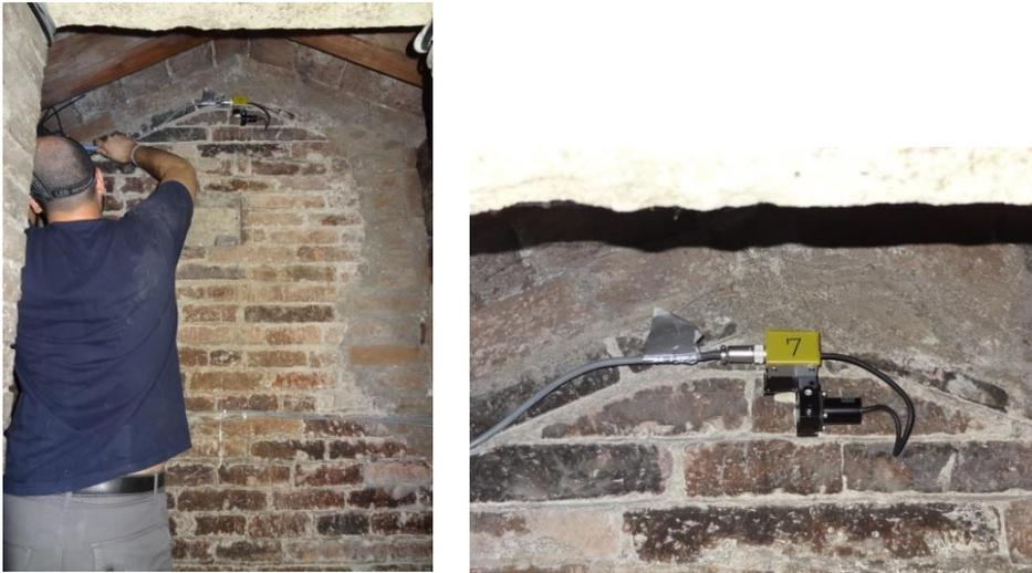
Figure 5.32 - Measurement point 7 - Recording channels and accelerometers 10 [27].
