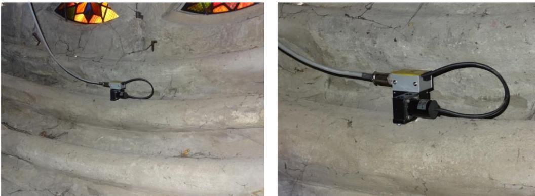
Figure 5.33 - Measurement point 8 - Recording channels and accelerometers 11 [27].
