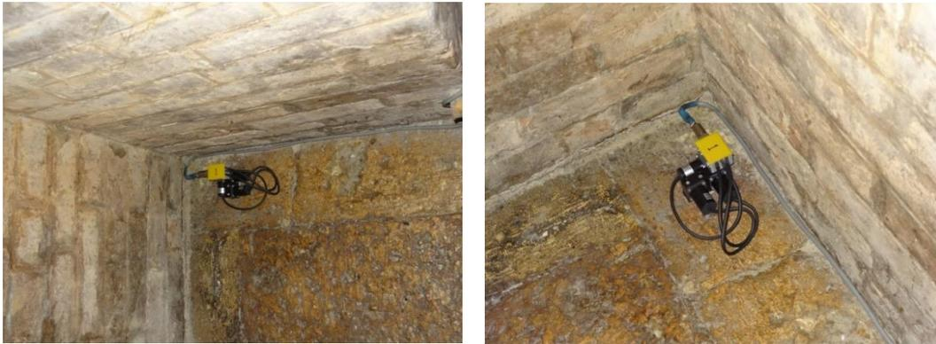
Figure 5.26 - Measurement point 1 - Recording channels and accelerometers 1, 2 and 3 [35].
