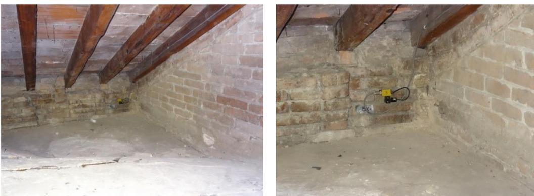
Figure 5.28 - Measurement point 3 - Recording channels and accelerometers 5 [35].
