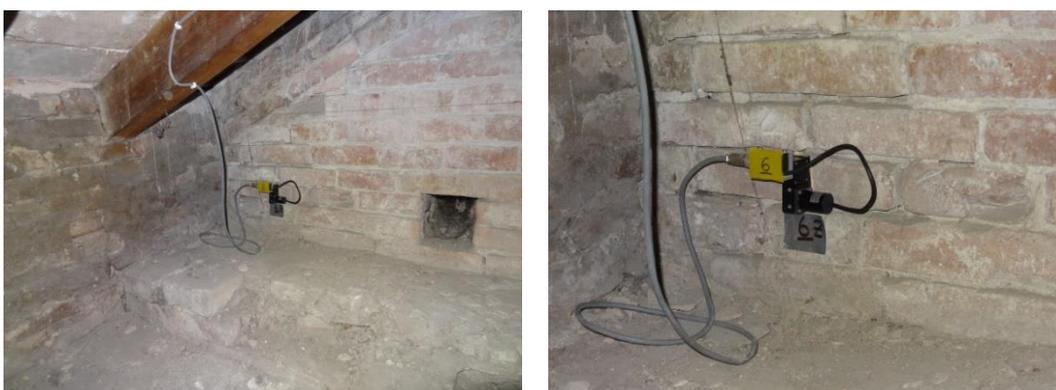
Figure 5.31 - Measurement point 6 - Recording channels and accelerometers 9 [27].
