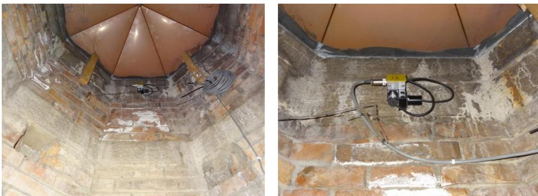
Figure 5.37 Measurement point 12 - Recording channels and accelerometers 15 and 16 [27].
