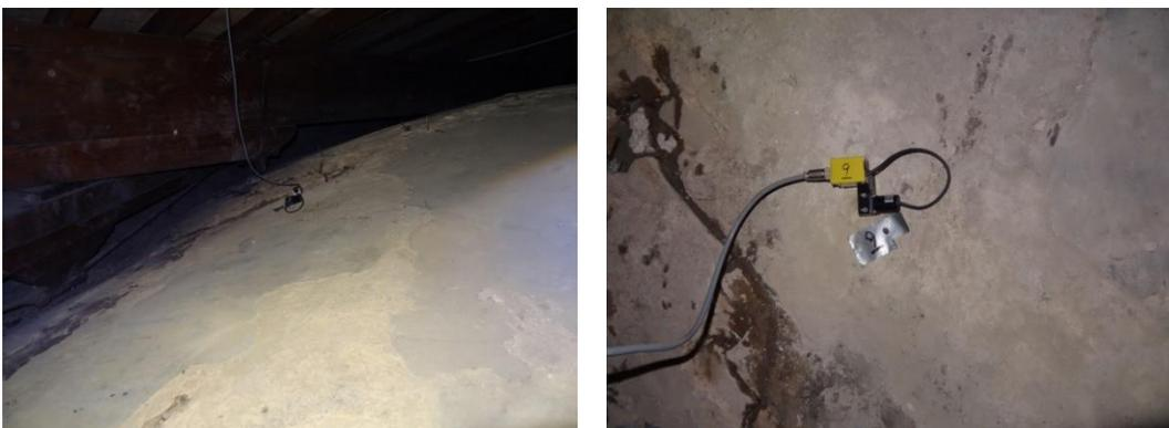
Figure 5.34 - Measurement point 9 - Recording channels and accelerometers 12 [27].
