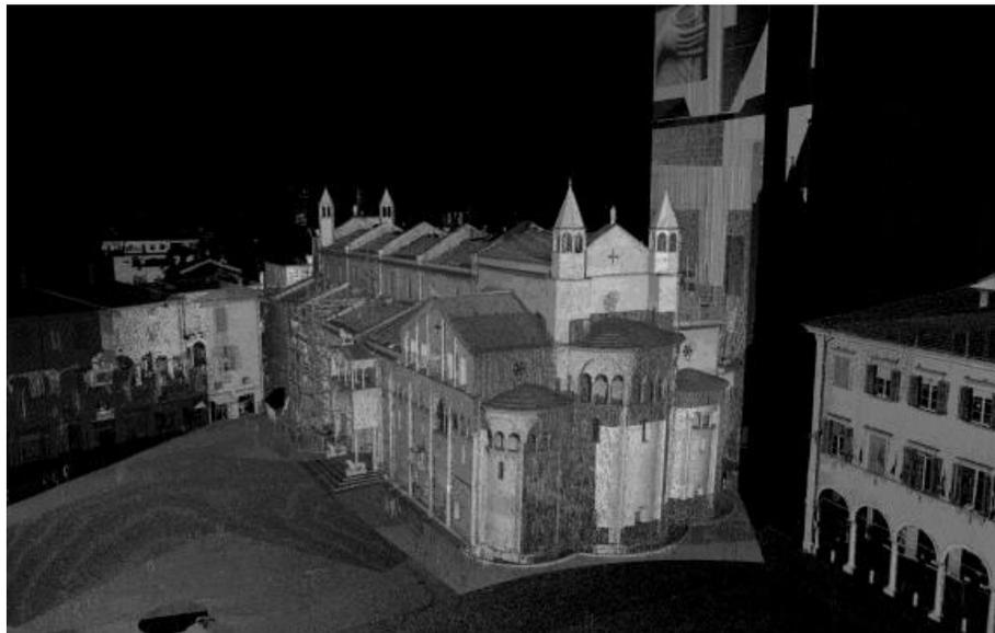
Figure 6.6 – Point cloud model: overall view of the Cathedral [51].
