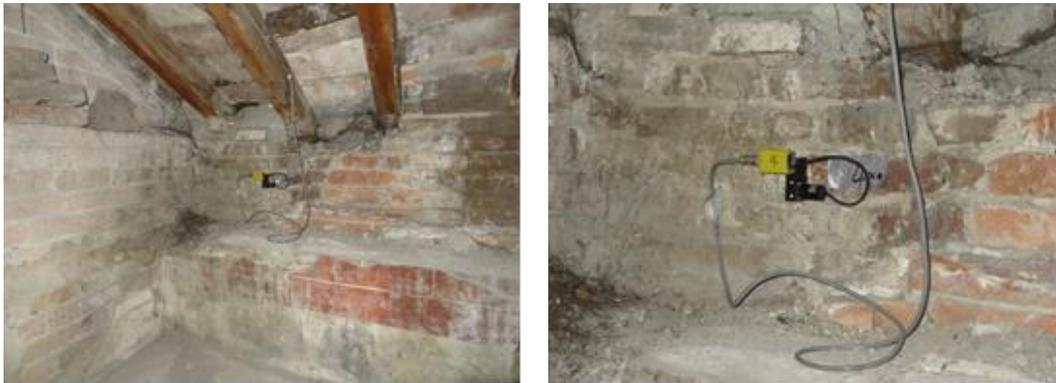
Figure 5.29 - Measurement point 4 - Recording channels and accelerometers 6 [35].
