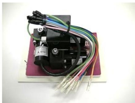
Figure 5.24 - Capacitive uniaxial accelerometer [35].
