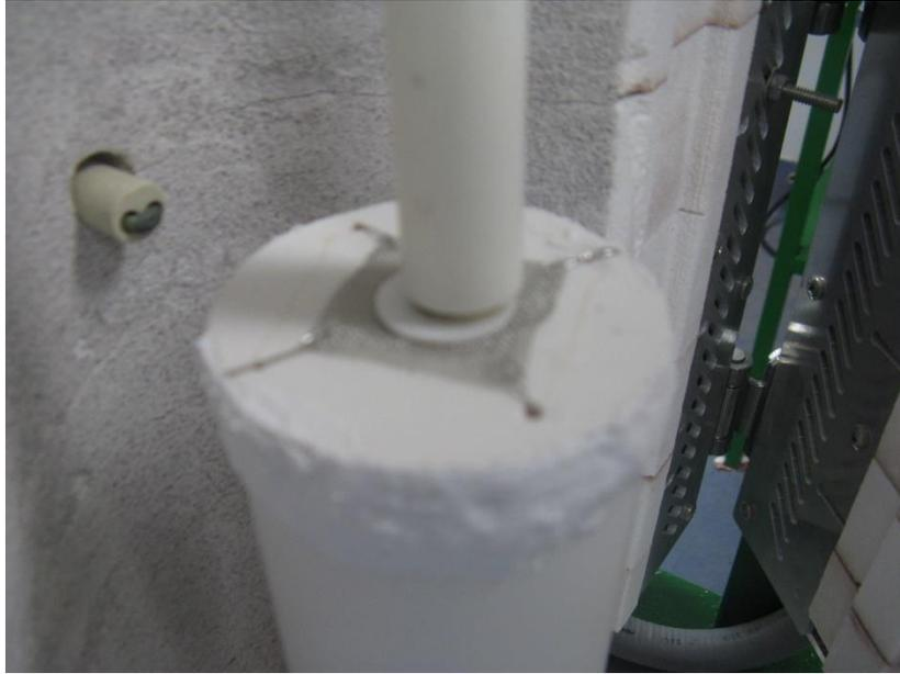
*Figure 17 Particular of the furnace with the cell pressed between the two tubes in order to increment the electrons transfer*
