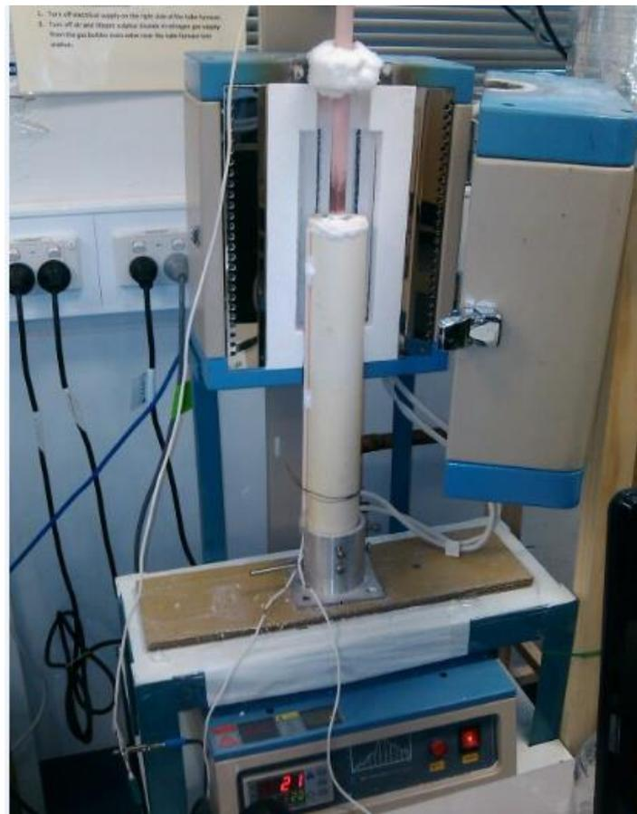
*Figure 16 Furnace and test station used to measure the electrochemical properties of the sintered cells at different temperature*
