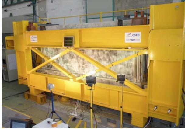
**Figure 3.2:** Steel frame of the specimen [7]
