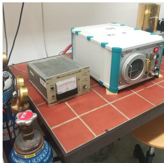
Figure 14-Femto Plasma chamber used in this project.
