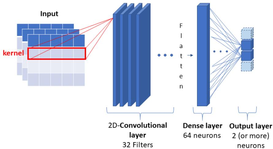
Figure 5.5. CNN architecture
