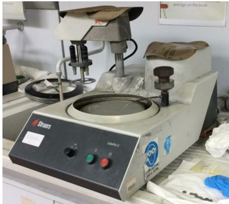
**Figure 2.44:** Grinding/polishing machine LaboPol-2, Struers.
