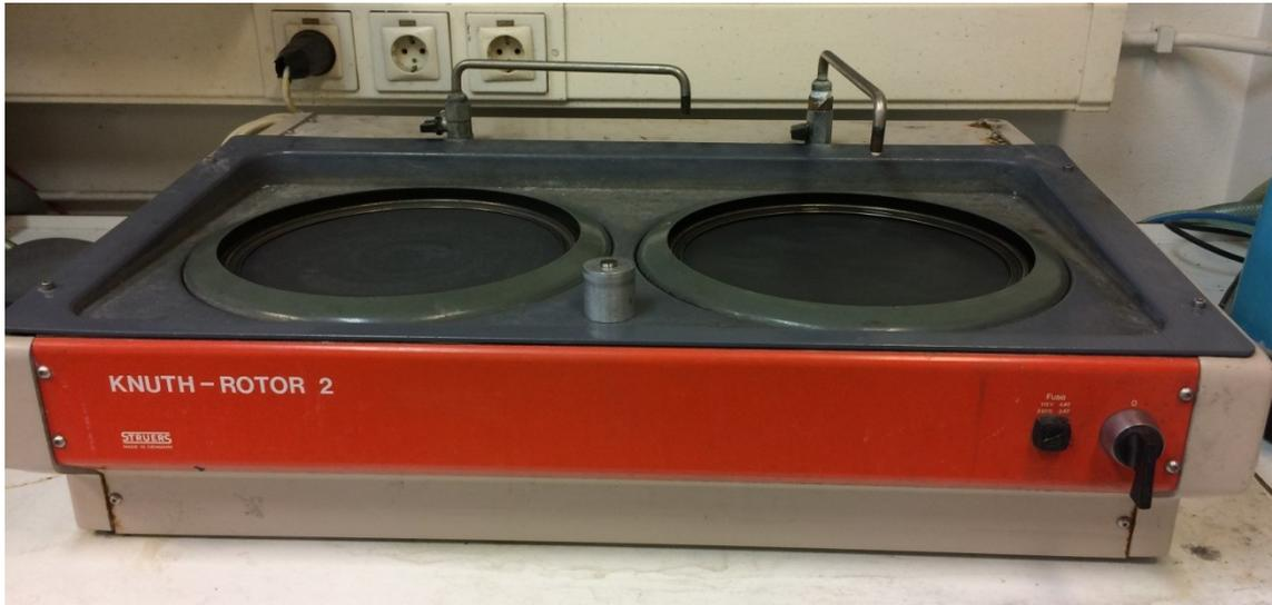
Figure 2.31: Polishing machine, Knuth-Rotor 2, Struers.
