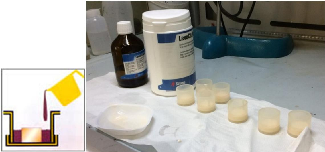
Figure 2.45: cold-embedded samples in the acrylic resin.
