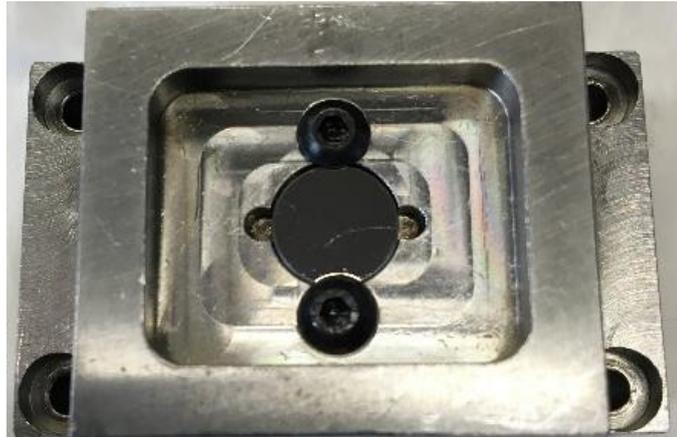
**Figure 2.36:** Bottom specimen holder.
