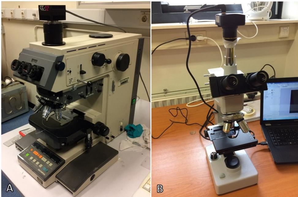
**Figure 2.40:** Optical microscopes, Olympus Vanox-T, Leica Microsystems B.V. (A) and AmScope, ME300 Series (B).
