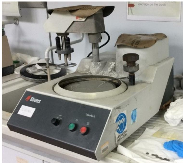
**Figure 2.44:** Grinding/polishing machine LaboPol-2, Struers.
