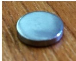
**Figure 2.1:** Commercially pure titanium (Ti cp) disk.
