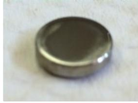
**Figure 2.2:** Titanium alloy (Ti6Al4V) disk.
