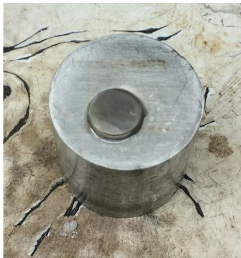
Figure 2.32: Support used to polish disks.
