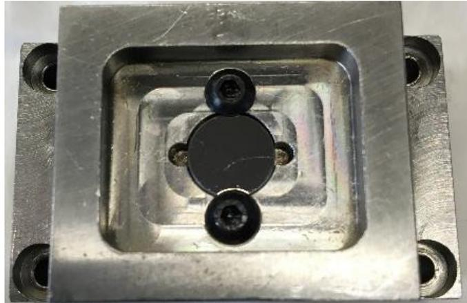
**Figure 2.36:** Bottom specimen holder.
