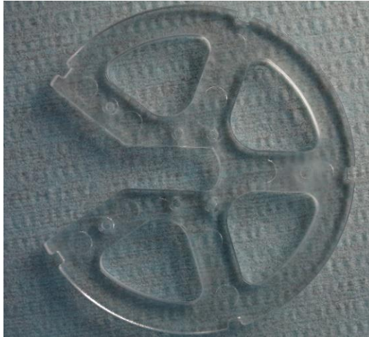
Figure 4.13. Visual inspection of retainer shelf, 1450 PSI
