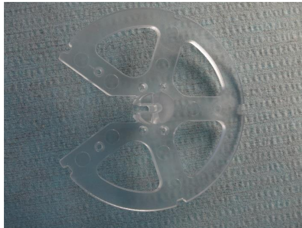
Figure 4.7. Visual inspection of Solo Smart retainer shelf, 2900 PSI
