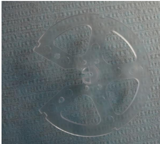
Figure 4.14. Visual inspection of Solo Smart retainer shelf, 1450 PSI
