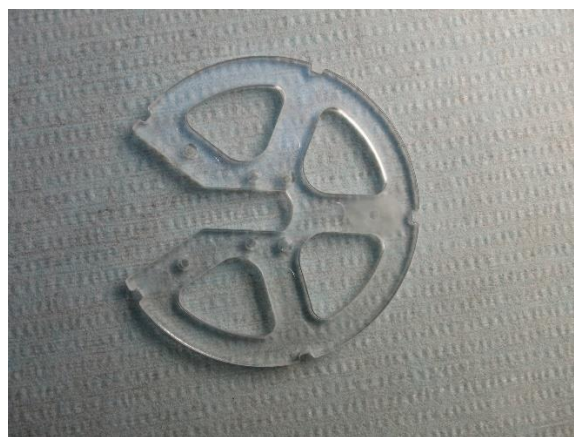
Figure 4.20. Visual inspection of retainer shelf, 1015 PSI
