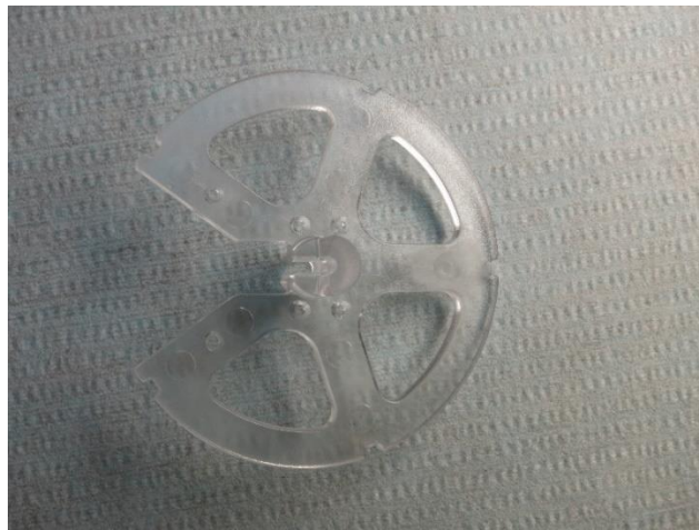
Figure 4.19. Visual inspection of Solo Smart retainer shelf, 1015 PSI
