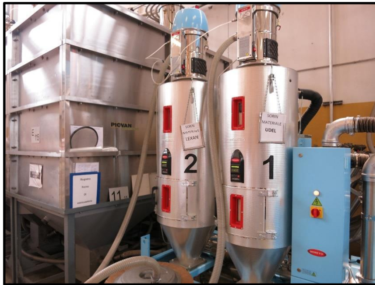
Figure 2.27. Hopper-drier system used by the external supplier
