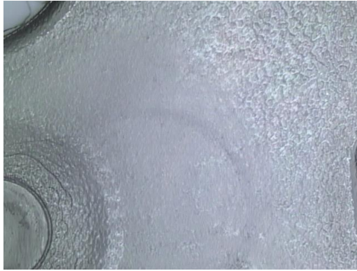
Figure 4.11. OGP inspection of retainer shelf, 2900 PSI
