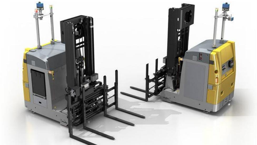
Figura 11 : AGV (Automatic Guided Vehicle)
