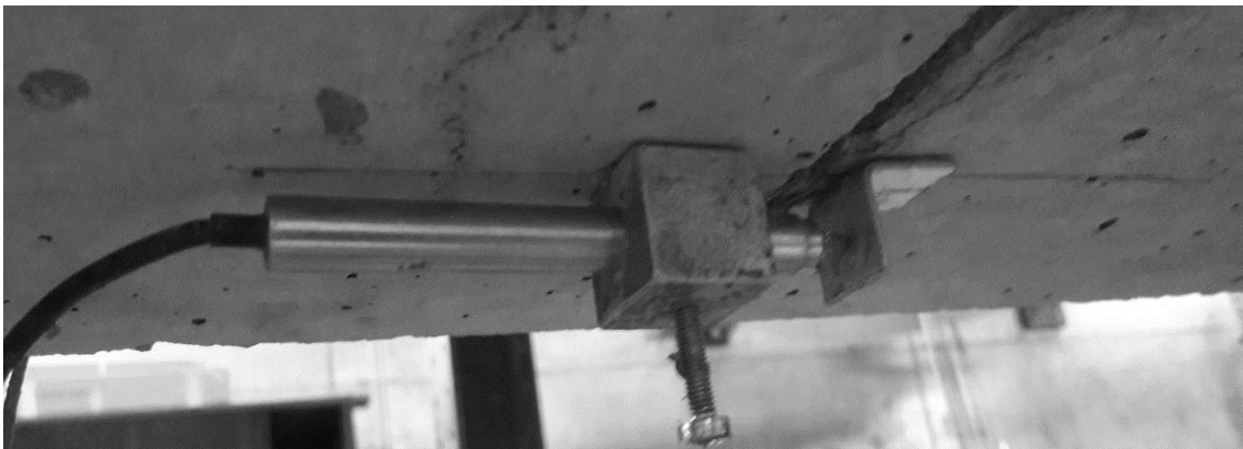
Figure 19 – Position of LVDT between the crack in the 3PNBBT.
