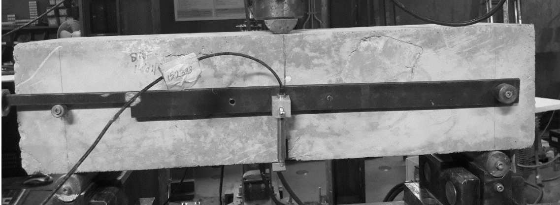
Figure 18 - Position of LVDT in a mid-span in the 3PNBBT.
