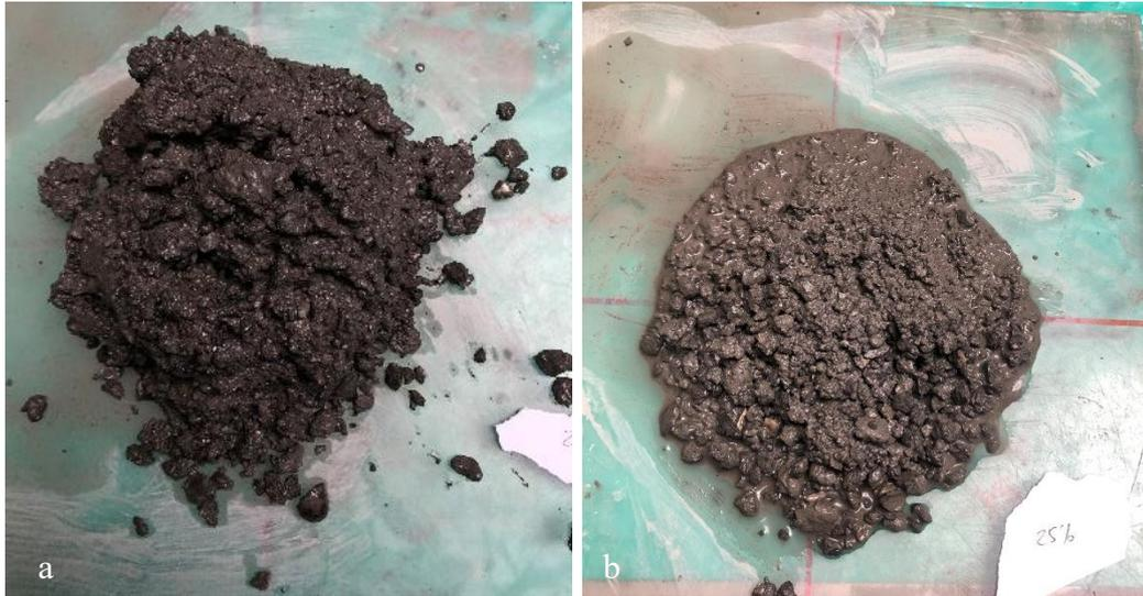
Fig. 5.4 Spandimento Mix1-P-20 (a) e Mix2-P-25 (b)
