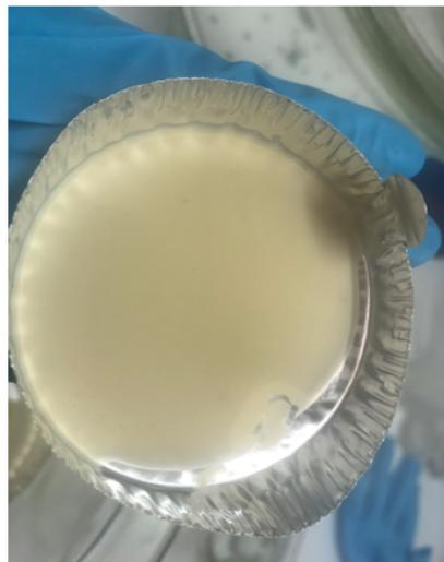
**Figure 4:** thermal curing of PET 1:10 EG degradation product
