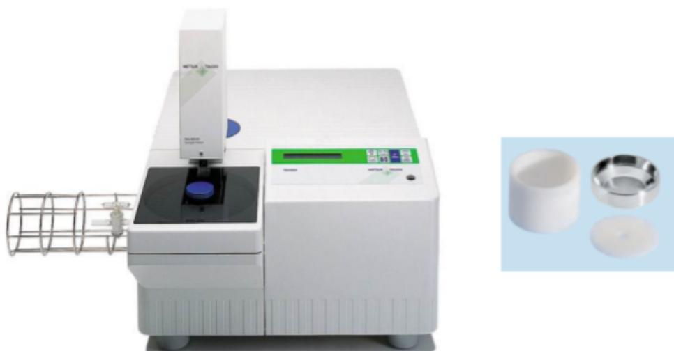
**Figure 3.9:** TGA apparatus and crucible used in the analysis
