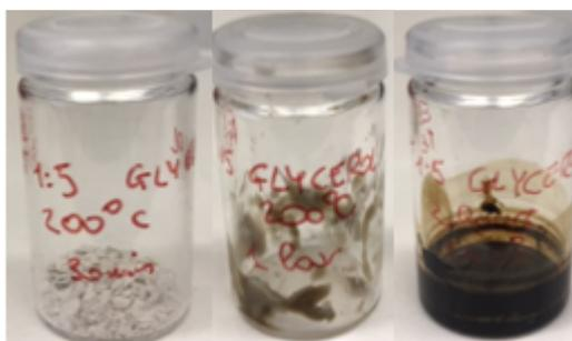
**Figure 2.4:** Depolymerization samples with GLY
