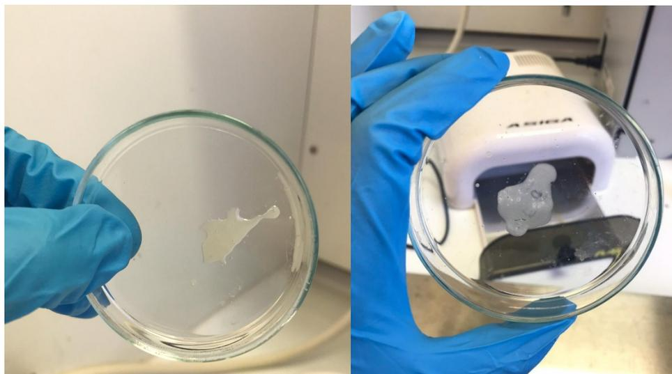
**Figure 4:** UV-curing of PET 1:10 EG degradation product
