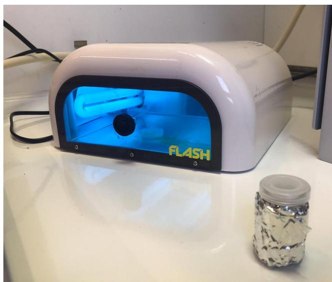
**Figure 2.10:** UV-curing apparatus used for the photopolymerization
