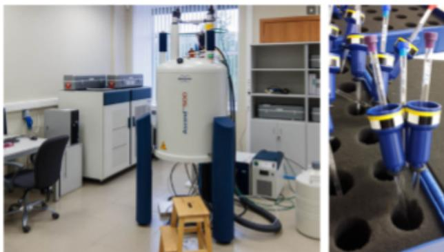
**Figure 3.3:** NMR apparatus [28] and sample tubes used for this analysis
