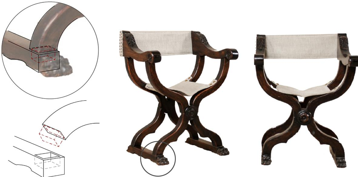
Figure 50. The structure of mortise and tenon at this chair (remade by author)
