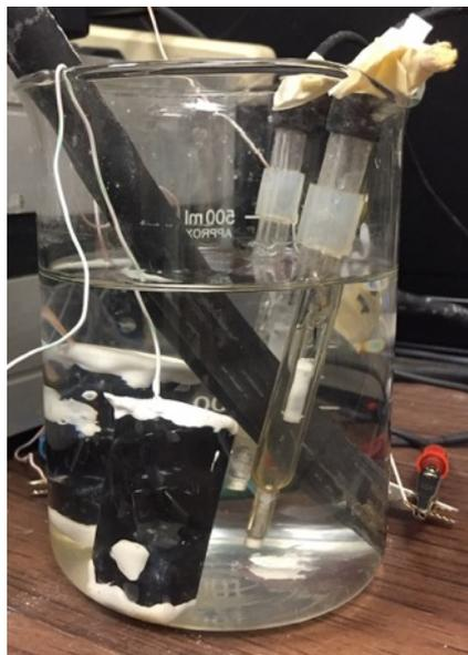
**Figure 3.11** Cell for Electrochemical Test.
