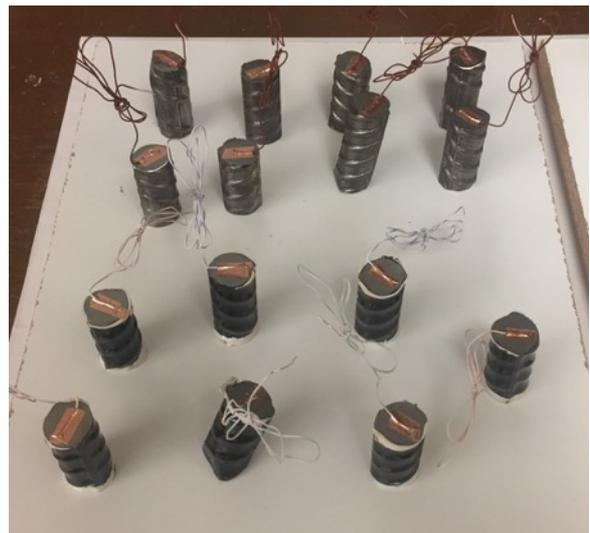
Figure 3.8 Samples Jointed with Wire and Copper Tape.
