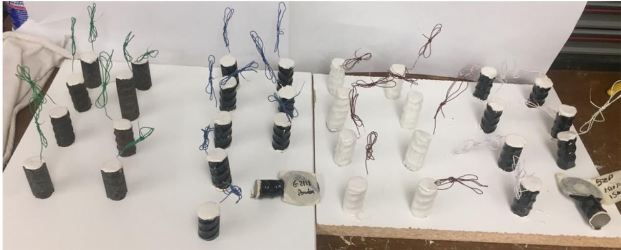
**Figure 3.9** Epoxy Coated Samples.
