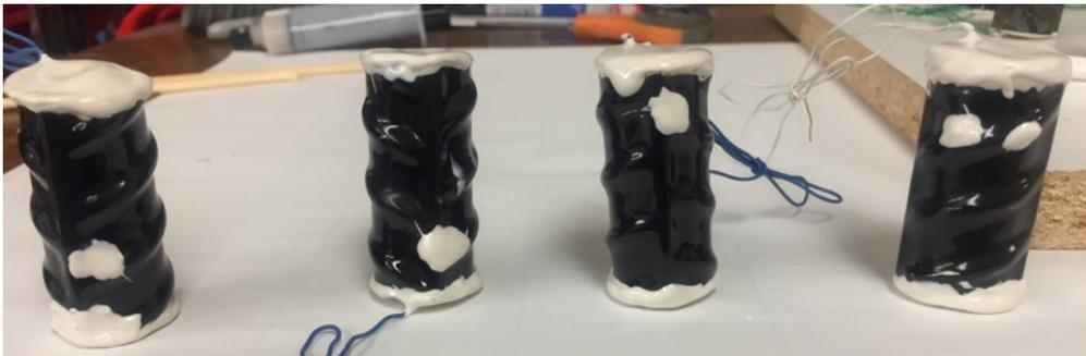
**Figure 3.10** Epoxy Coated Damages Points.
