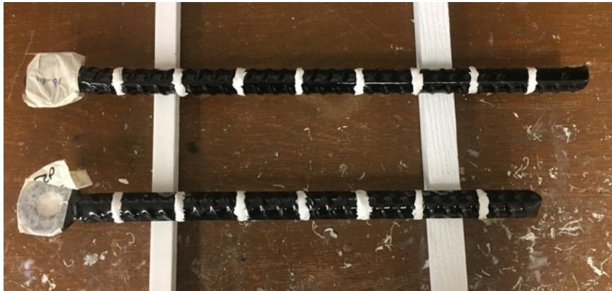
Figure 3.7 Marked Enamel Coated Rebar.
