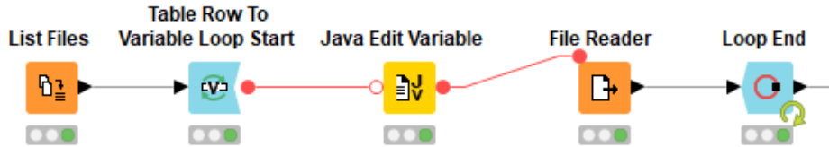
Figure 3.1: Workflow to read multiple Excel files and append them in a single file.
