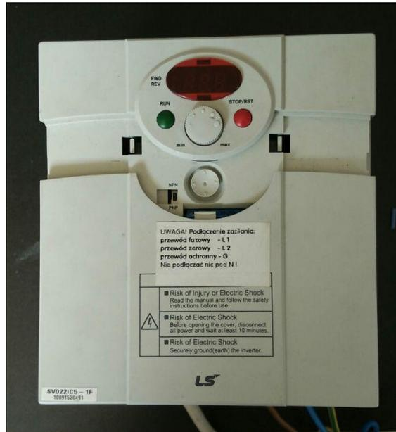
Figure 4.1: Front panel of the inverter
