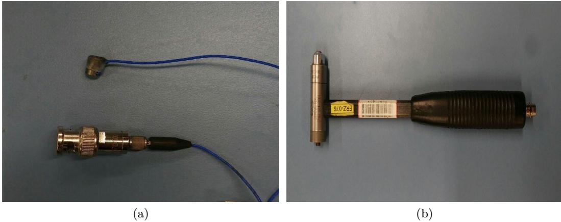
Figure 4.42: (a) Accelerometer and (b) hammer used for the evaluation of the FRF of the blade
