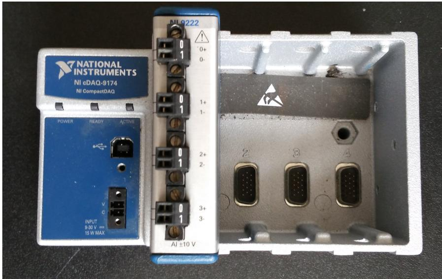
Figure 4.21: Analog-to-digital acquisition device
