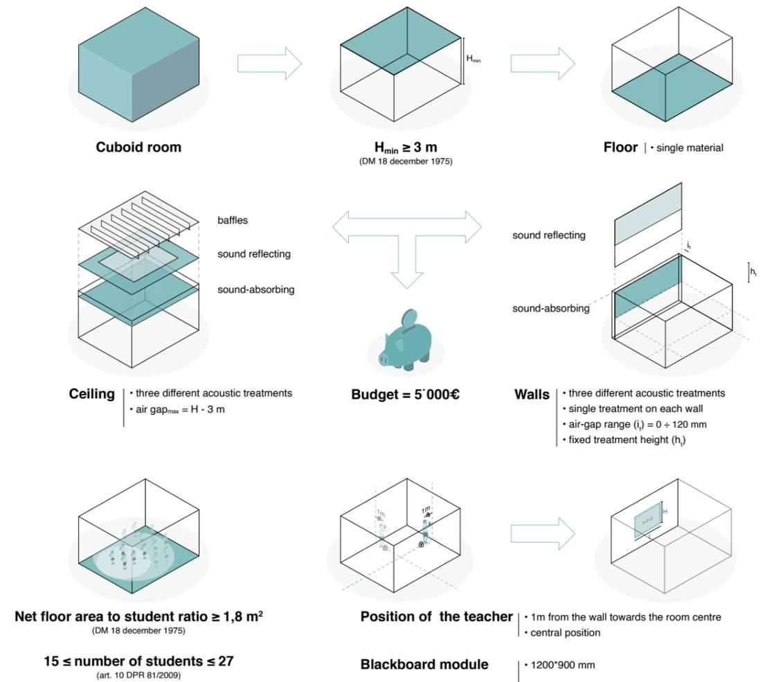
Figure 33. Main constraints adopted in the parametric model.
