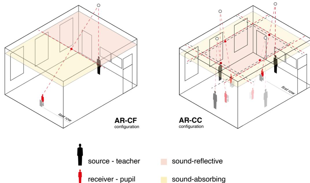
**Figure 39.** Image-source technique embedded the AR-C configurations in the algorithm.
