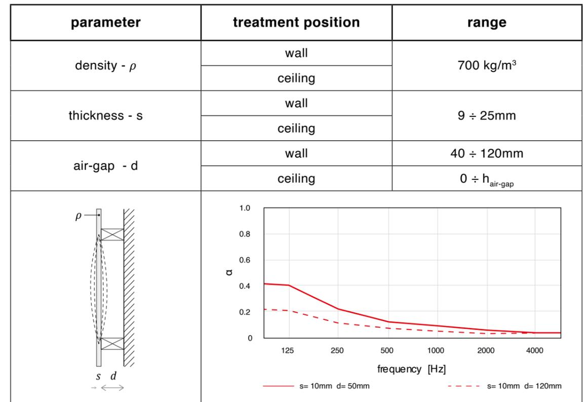
**Table 18.** Input data range and sound absorption curve for baffle system.
