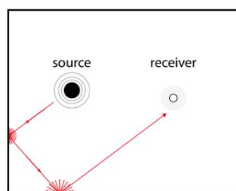
**Figure 50.** Principle of ray-tracing.
