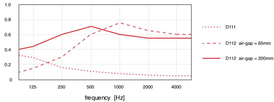
Figure 44. Sound-absorption curves of the brick-proof false-ceiling solutions.
