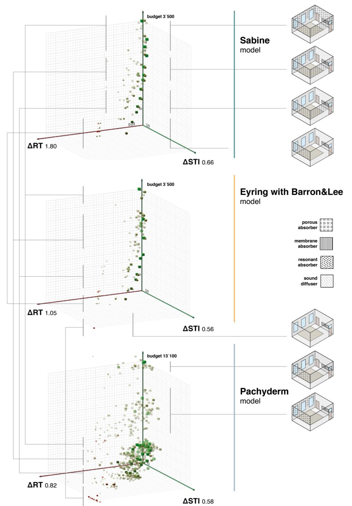
Figure 67. Final generation of Pareto-front solutions from RT-STI-budget based optimizations, with the constraint of no ceiling acoustic treatment.
