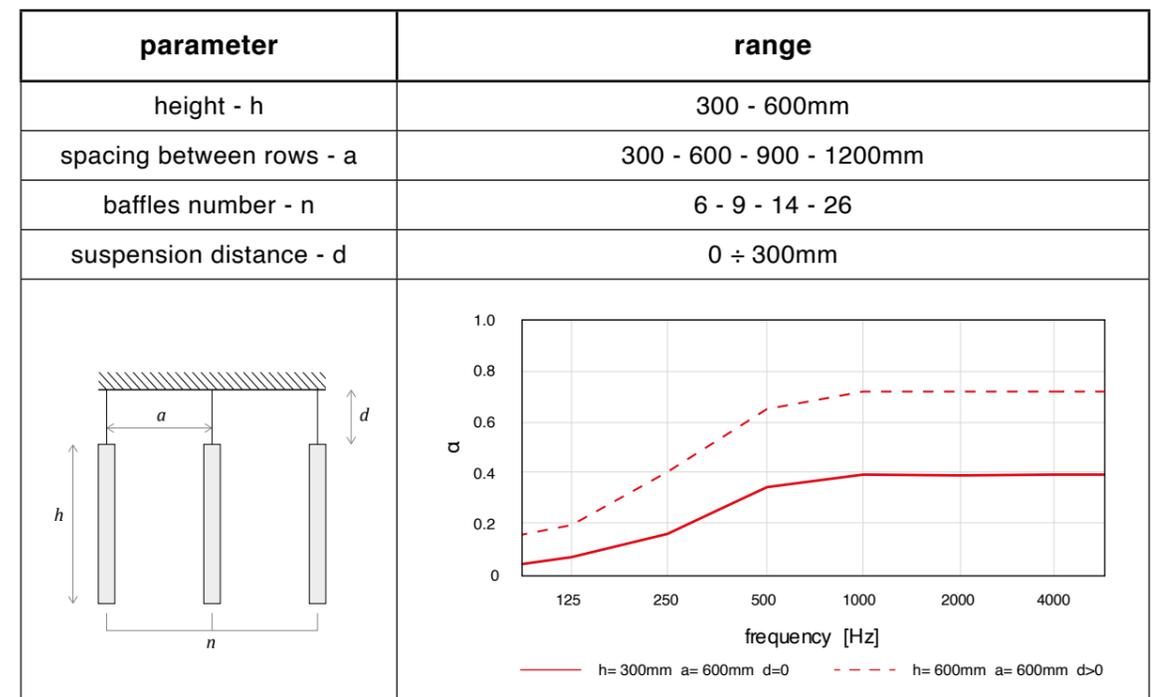
As far as the brick-proof false-ceiling are concerned, the main features of the available acoustic solutions have been indicated in Table 11, in the following figure, the respective sound-absorption curves are shown.
