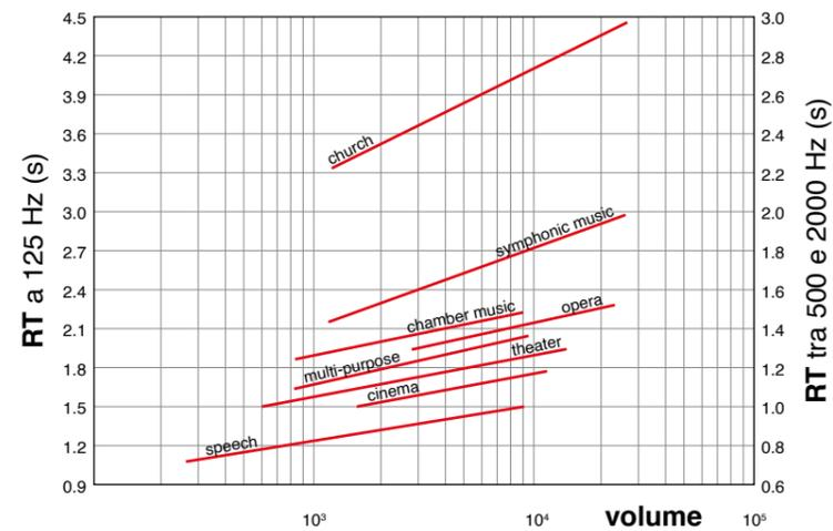
Figure 08. Optimum reverberation time for intended use.
