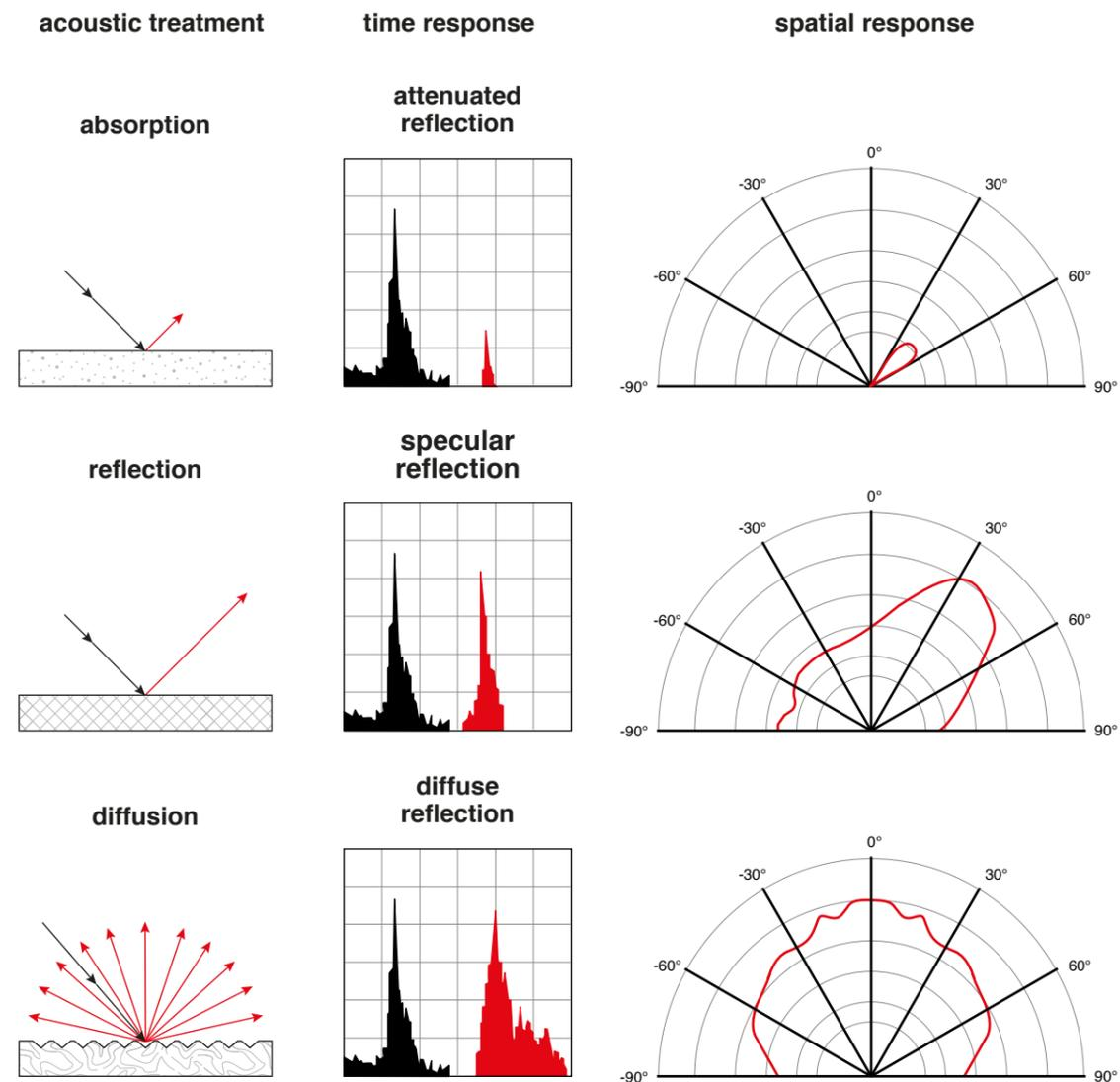
**Figure 12.** Correlation between reflection phenomenon and absorbing materials.
