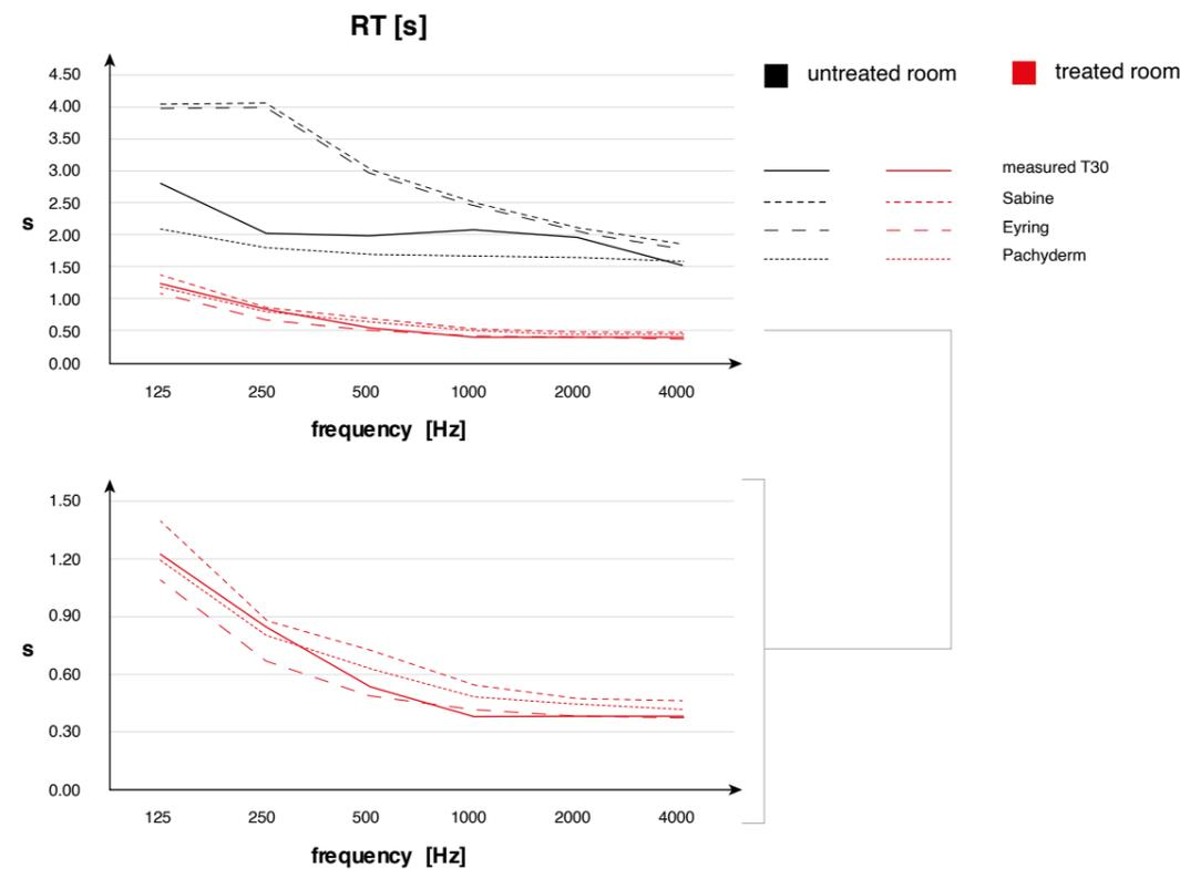
Figure 55. Reverberation time predictions with various calculation methods.
