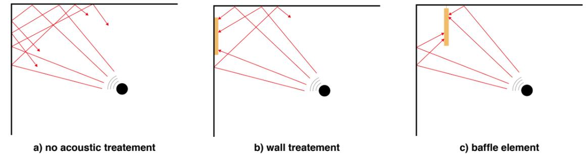
**Figure 40.** Baffle double sound absorption.
