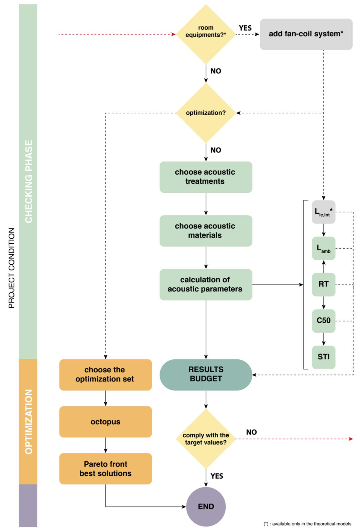
Figure 71. Simplified flow chart of the developed algorithm: project condition.
