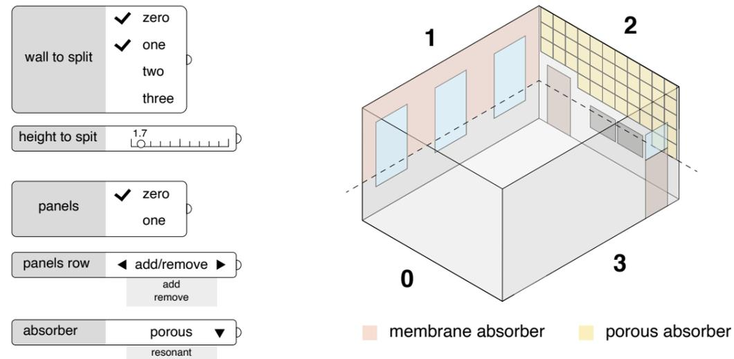
Figure 37. Available GH components for wall treatment.
