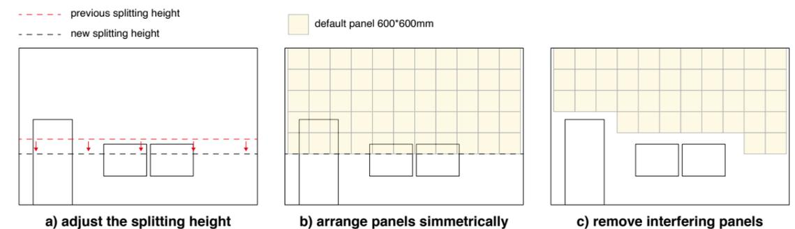
**Figure 36.** Algorithmic operations on the wall treatment.
