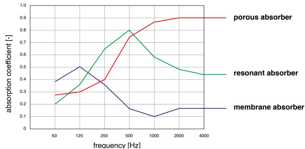
**Figure 13.** Absorption curves for absorbent materials.
