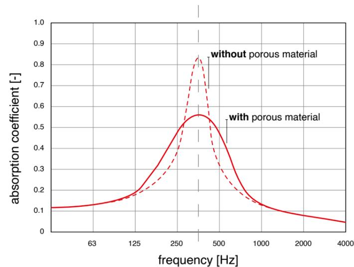
**Figure 15.** Absorption curve of an acoustic resonator as a function of frequency, with and without porous material inside the air cavity.
