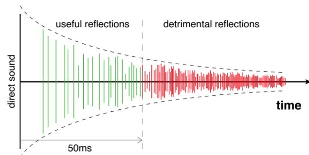
Figure 09. Relation between useful and detrimental reflections.
