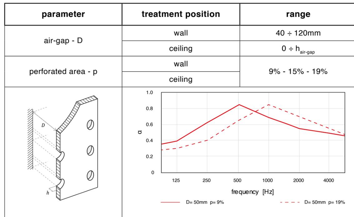
**Table 17.** Input data range and sound absorption curve for membrane absorbers.
