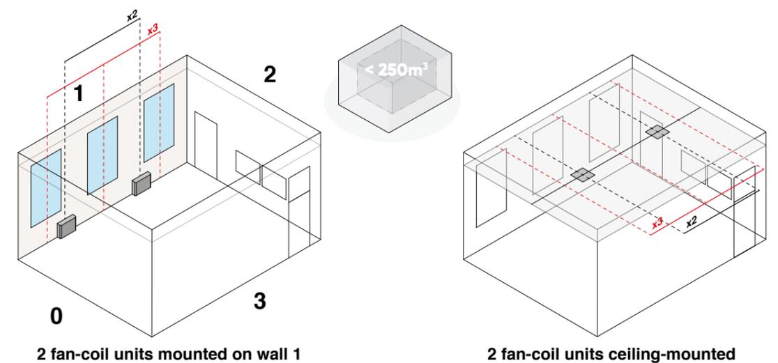
Figure 42. Fan-coil units arrangement.
