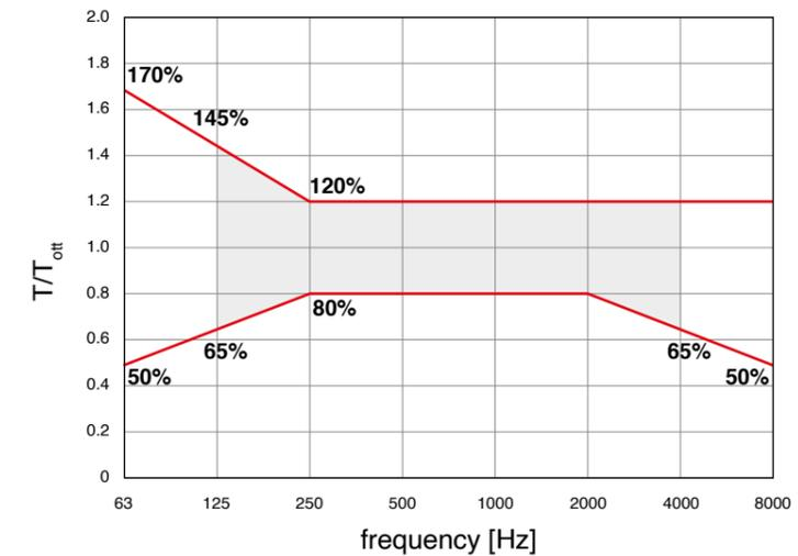
**Figure 18.** Frequency dependent tolerance range of reverberation time referred to  $T_{ott}$ .
