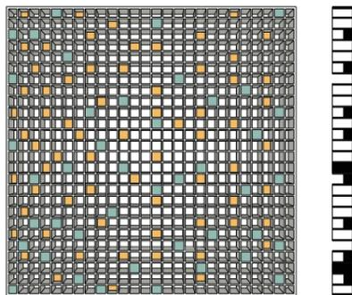
**Figure 52.** 2D Schroeder diffuser.
