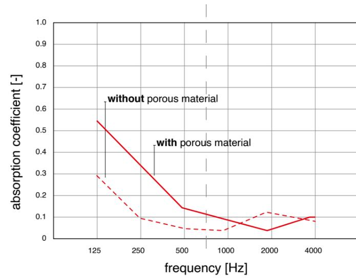
**Figure 16.** Absorption curve of a membrane absorber as a function of frequency with and without porous material in the air cavity.
