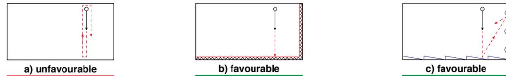
**Figure 20.** Distribution of the acoustic material on parallel surfaces.
