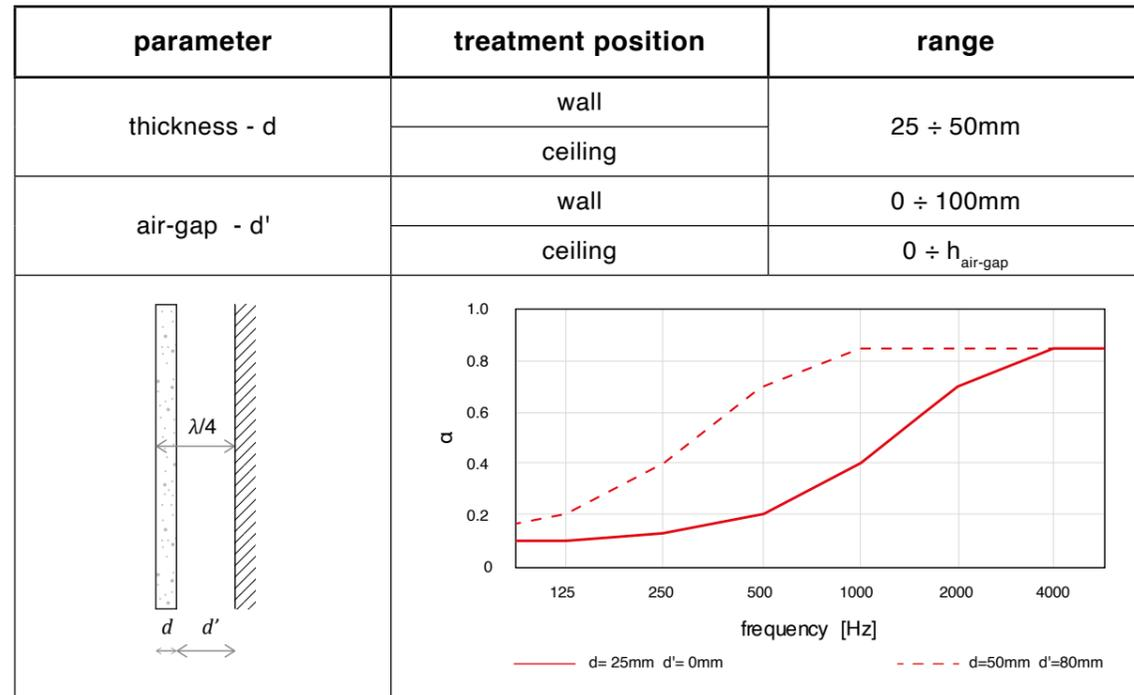
**Table 16.** Input data range and sound absorption curve for resonant absorbers, h=12.5mm.
