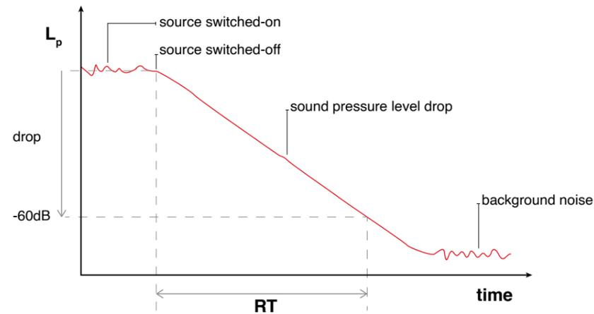
**Figure 06.** Graphic representation of the Reverberation Time.
