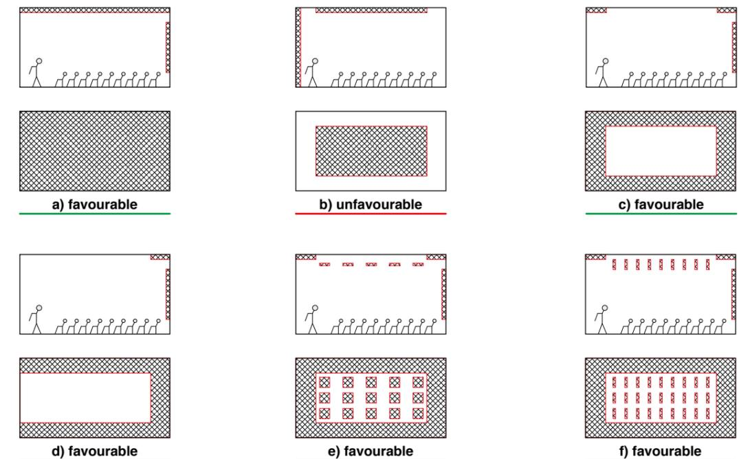
**Figure 19.** Distribution of sound absorption surfaces for small and medium-sized rooms.
