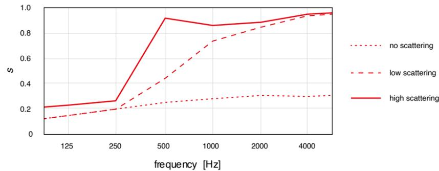
Figure 54. Comparison between the three scattering curves of materials in Pachyderm.
