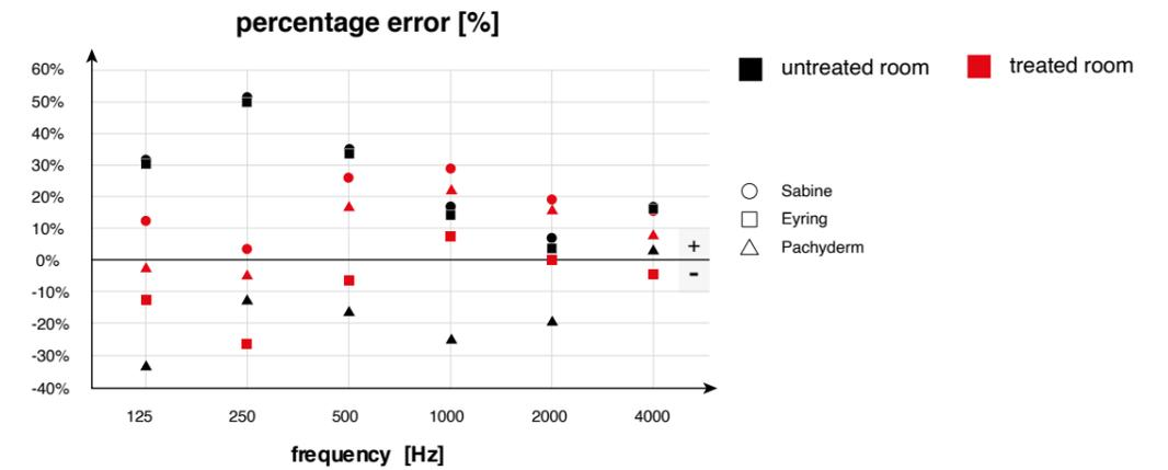
Figure 56. Percentage relative differences of reverberation time predictions with various calculation methods.
