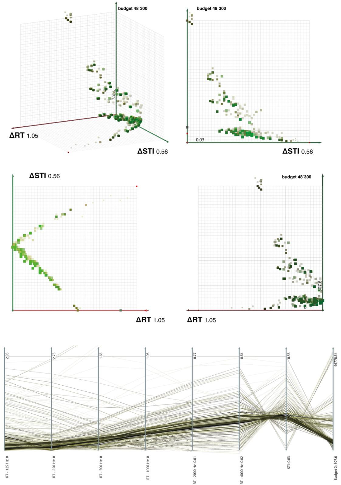
Figure A08. 2D and 3D views of Pareto-front optimization from Eyring with Barron&Lee model.
