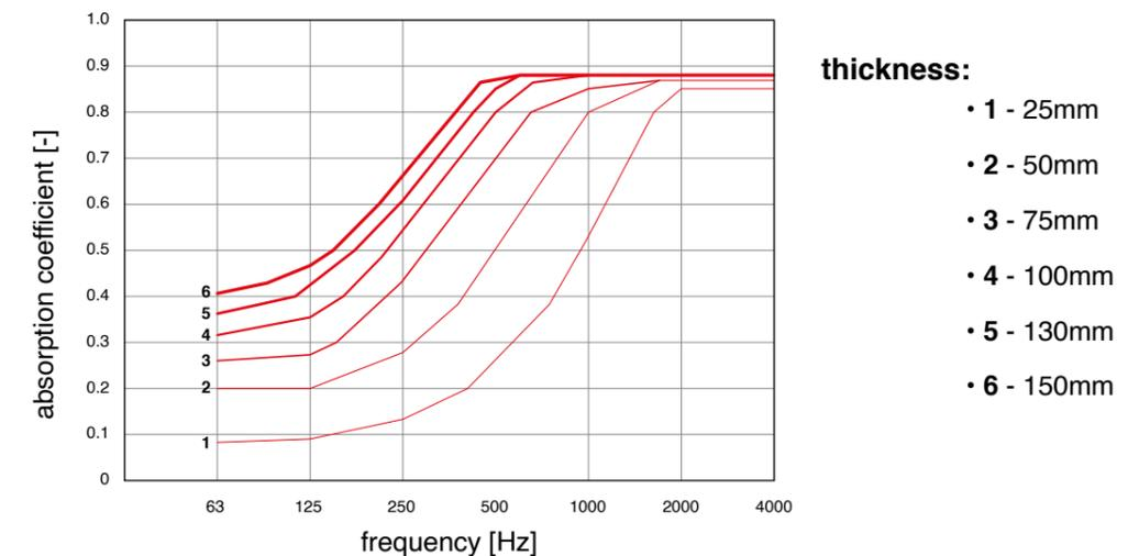
**Figure 14.** Incidence of different thickness sound on the mineral wool absorbers' absorption coefficient.
