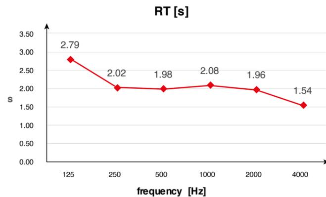
Figure 26. Measured reverberation time.
