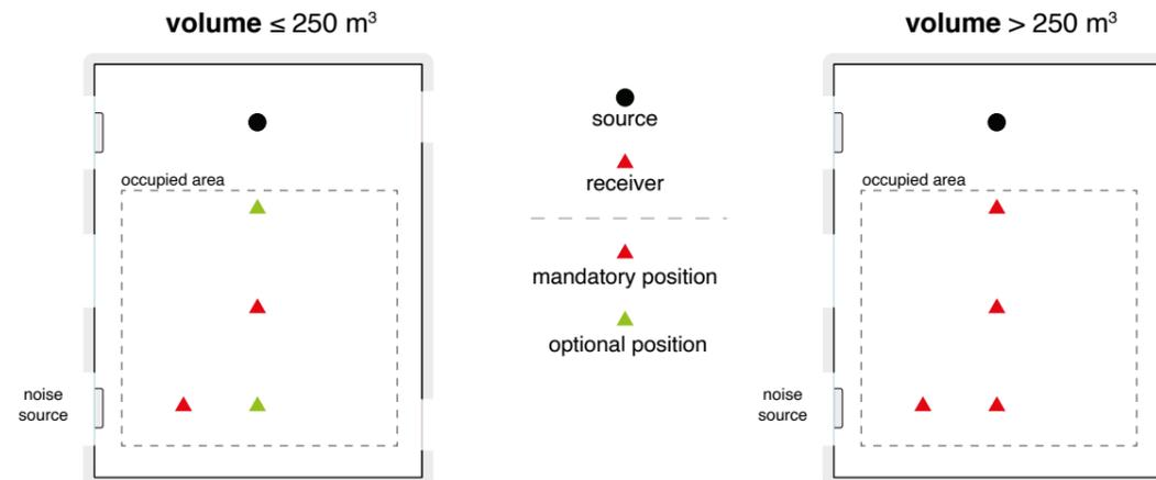
**Figure 17.** Identification of measurement user-receiver positions in relation to volume and noise source.
