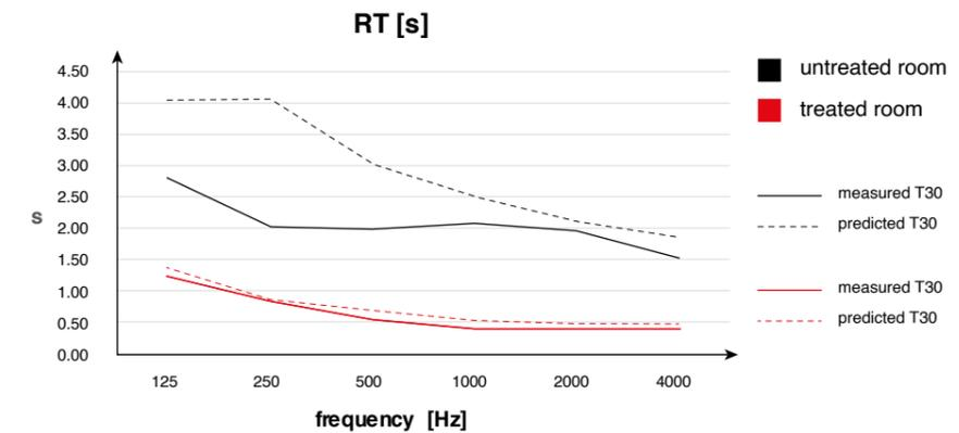
Figure 48. Comparison between the measured and predicted reverberation time in the untreated and treated classroom.
