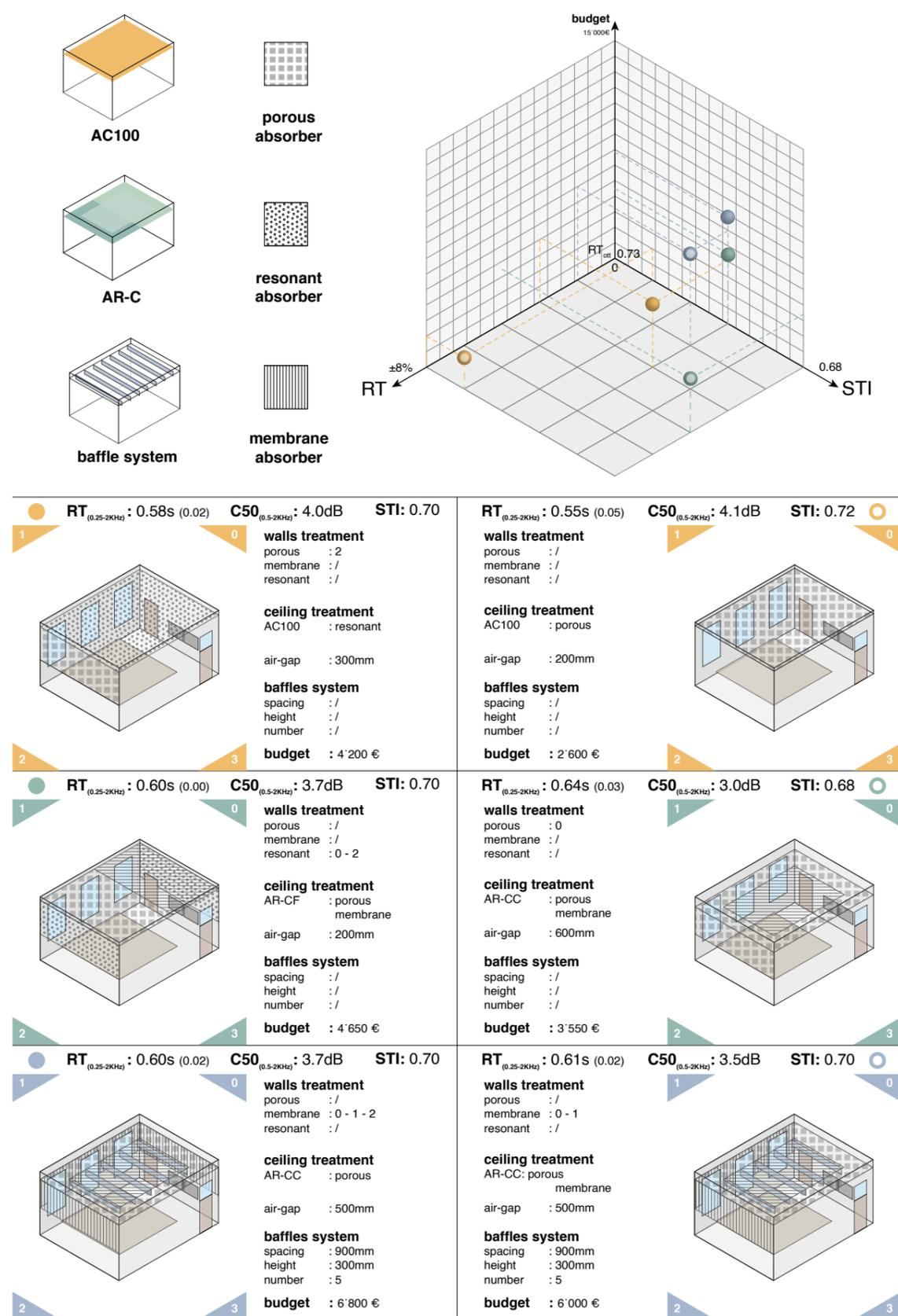
Figure 63. Eyring with Barron&Lee theory model best configurations.
