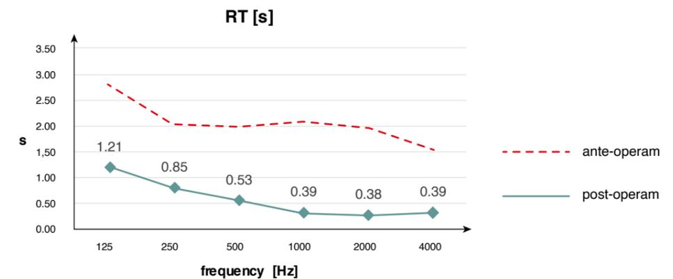
Figure 28. Measured reverberation time after the acoustical renovation.
