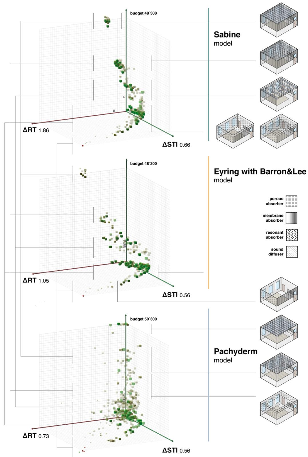
**Figure 59.** Final generation of Pareto-front solutions from RT-STI-budget based optimizations.
