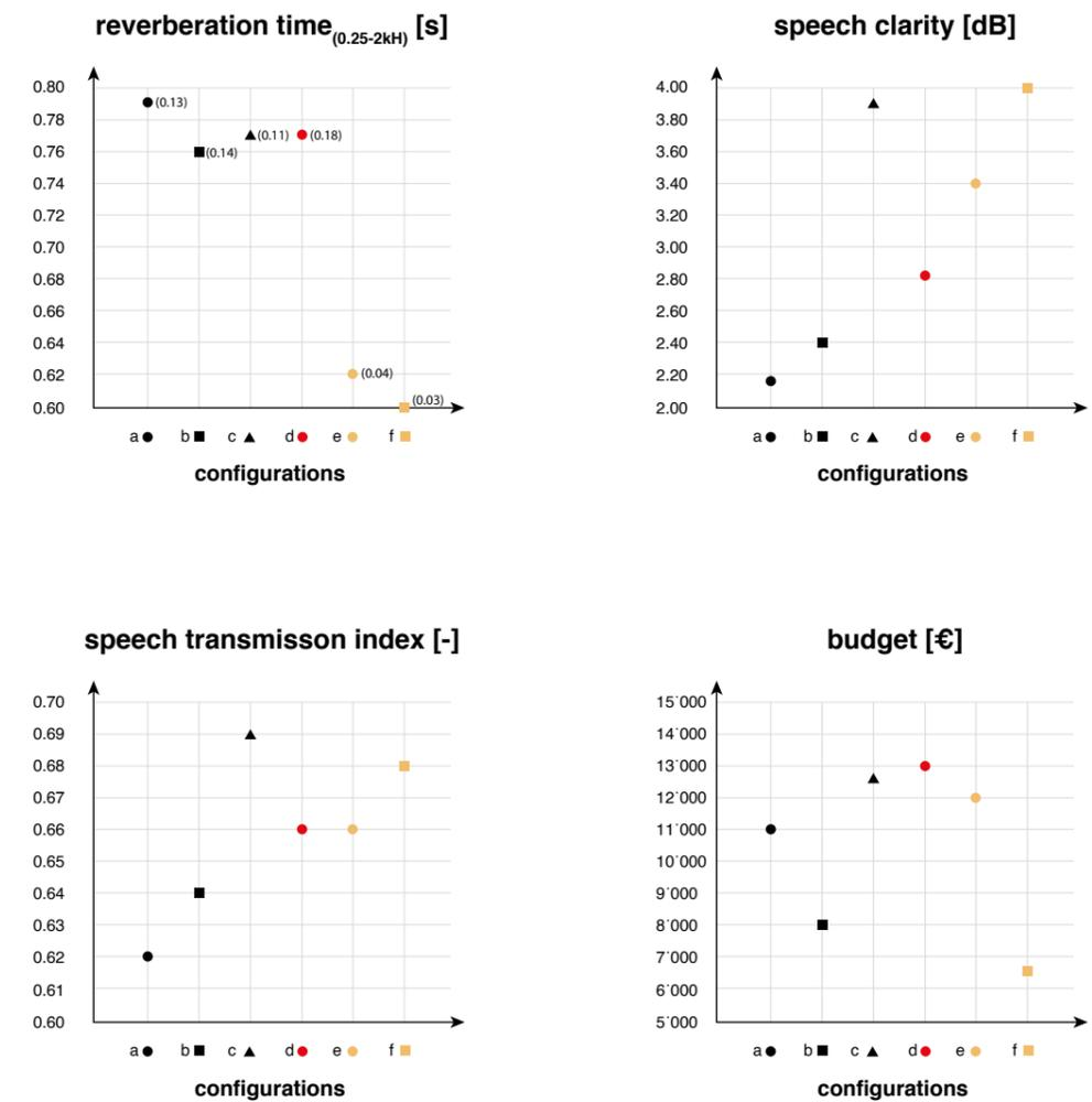
Figure 69. Comparison between the acoustic and objective parameters of the Pareto-front optimization.
