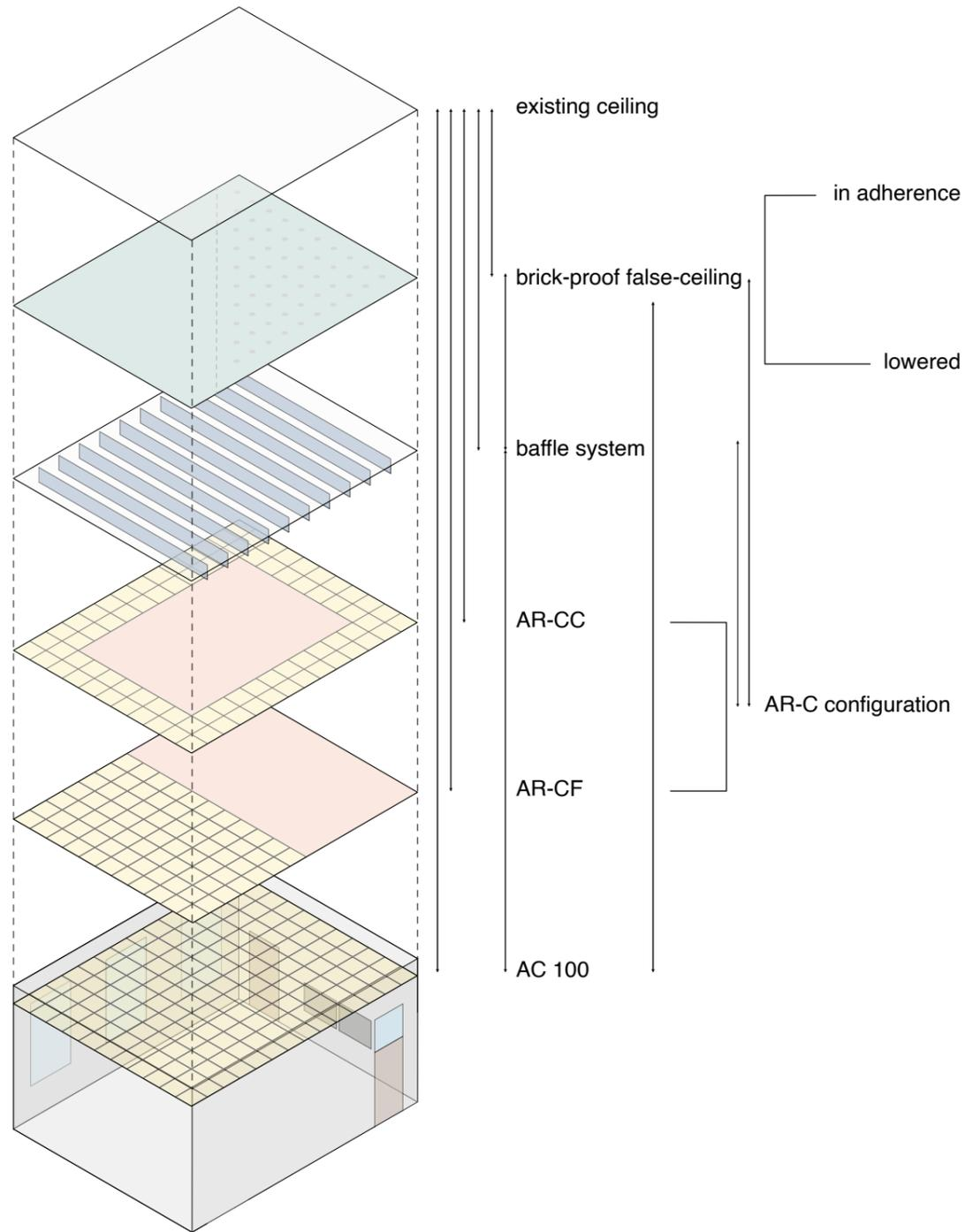
Figure 41. Ceiling acoustic treatments.
