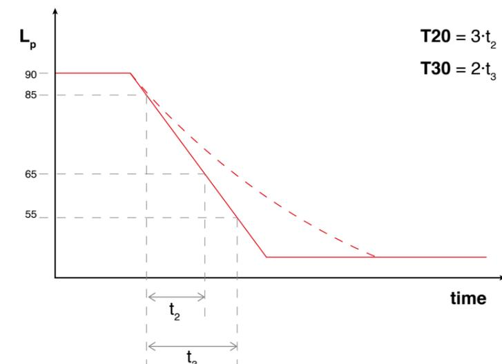
**Figure 07.** T20 and T30 can differ if the decay curve is bent.
