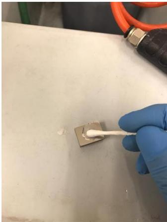
Figure 70) surface cleaned using a drop of liquid soap and a cotton-fioc.
