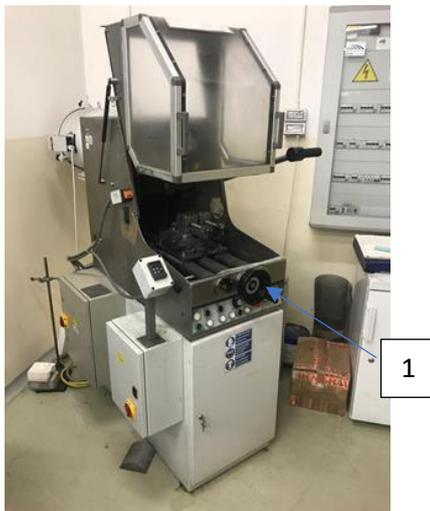
Figure 60) cutting machine with positioning system (1)
