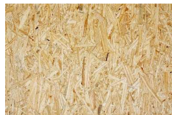
Figura 1. Oriented Strand Board.
