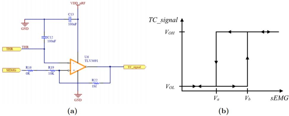
Figure 2.10. a) Comparator in Schmitt Trigger configuration, b) Output Hysteresis curve
