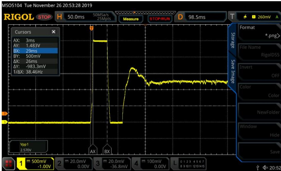
Figure 5.4. Focus on the INA behavior during the startup transient of the Acquisition Channel
