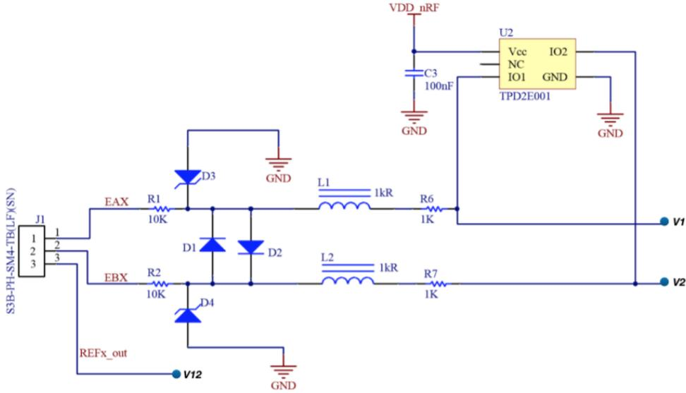
Figure 2.2. Mitor2 Analog Front End Overvoltage Protection circuit
