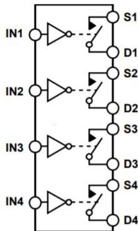
Figure 2.28. 4 Channel Switch SPST structure
