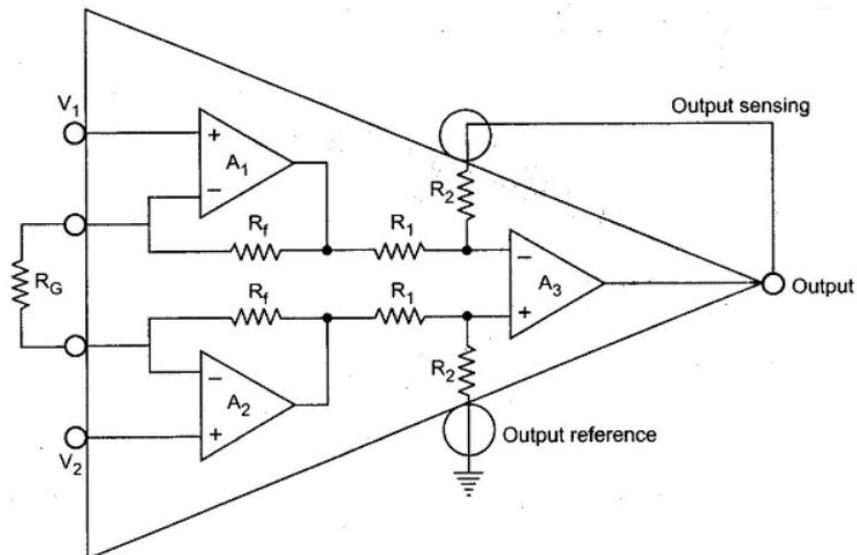
Figure 2.25. Instrumentation amplifier classic structure. Gain adjustable by changing  $R_G$
