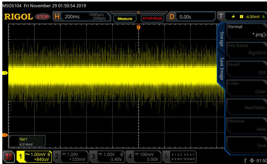
Figure 5.10. Dropout voltage on the acquisition channel 1.25V voltage reference output during the SD periodic writings in the new version of the system
