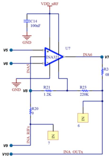
Figure 2.5. Amplification stage,  $G=922V/V$
