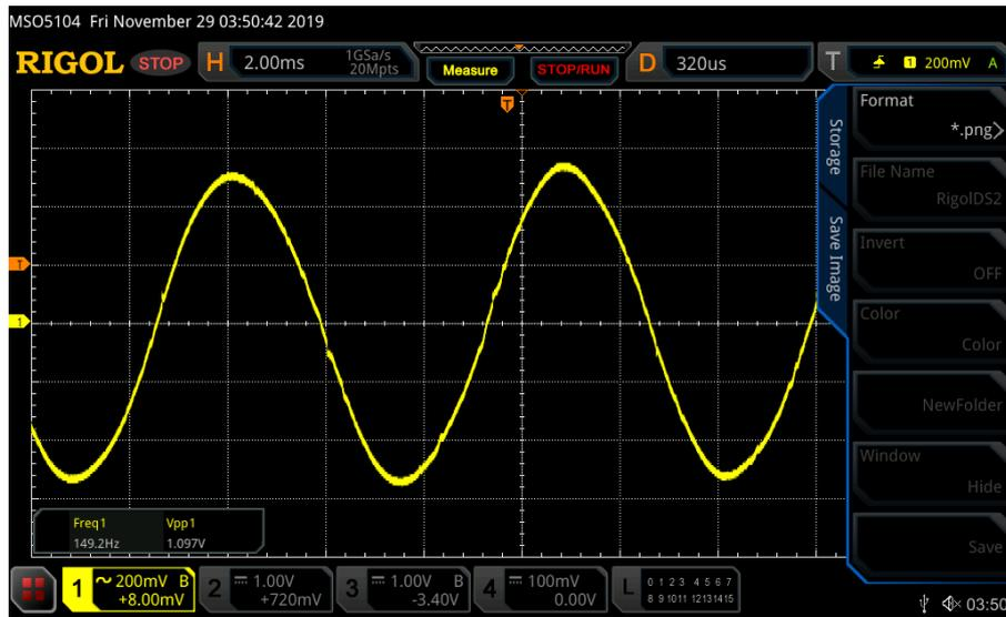
Figure 5.14. Gain 1500 test with hundreds of  $\mu V$  in INA differential input
