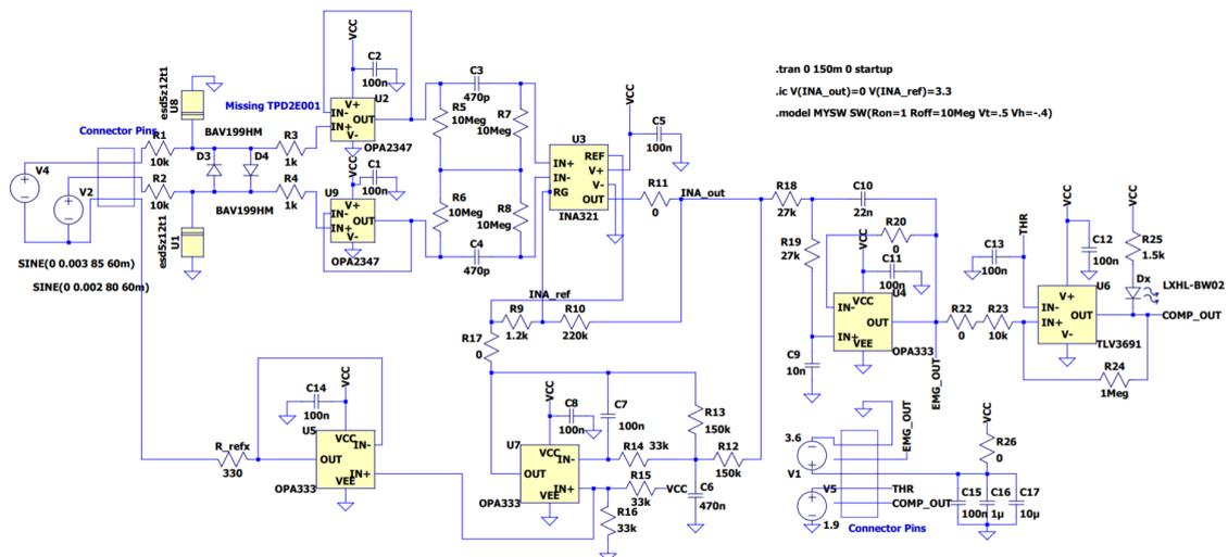
Figure 2.14. Analog Front End LTSpice circuit for deeper investigation
