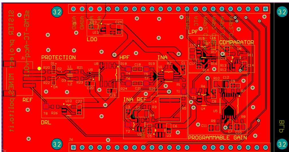
Figure 3.14. Analog Front End PCB Top
