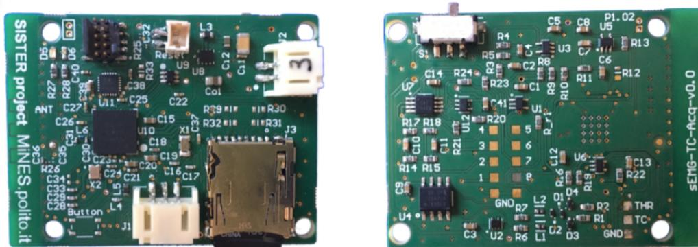
Figure 1.4. Mitor2 slave: Top side (*left*) is reserved for the digital part and bottom side (*right*) is reserved for the analog part
