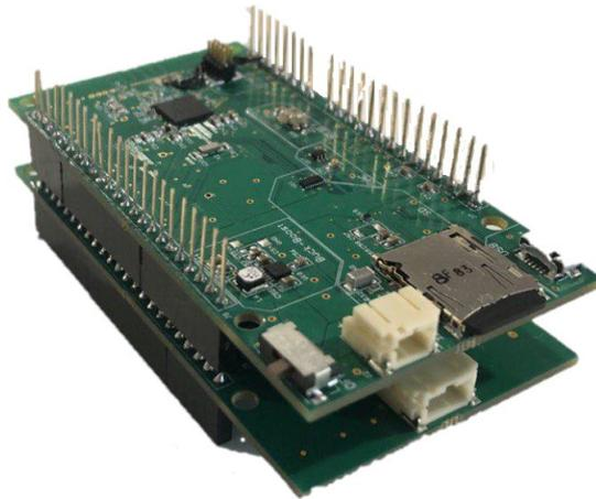
Figure 5.1. Two modules system assembled
