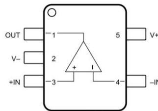
Figure 2.27. Operation Amplifier Component
