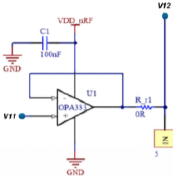
Figure 2.8. Driven Right Leg circuit
