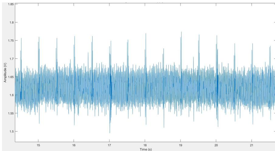
Figure 5.6. Baseline of sEMG signal acquired influenced by power supply dropout voltage during the periodic SD writings in the precedent versions of the system
