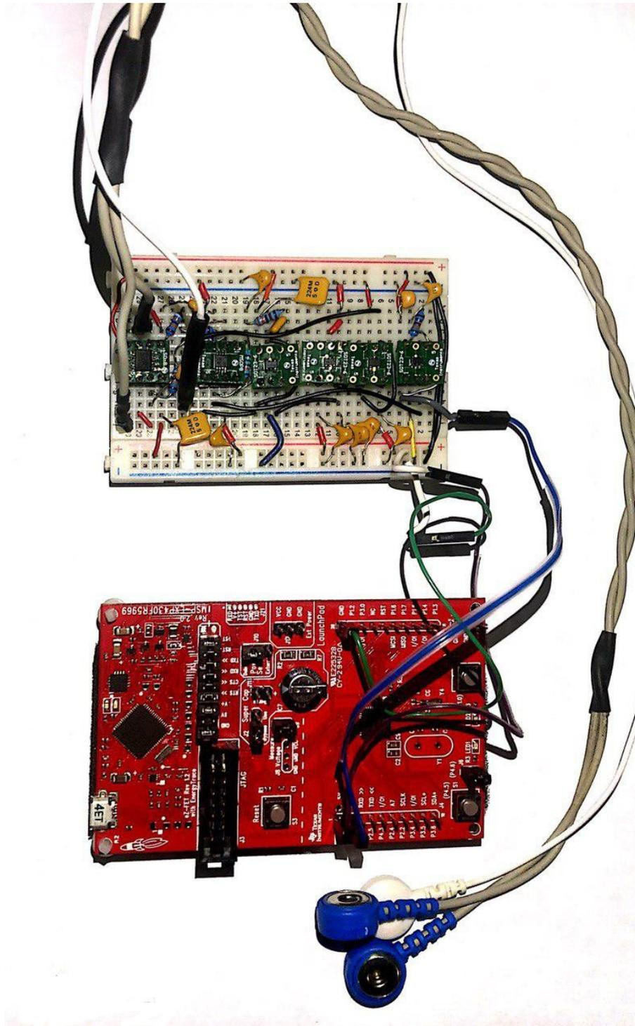
Figure 2.39. System composed by the Analog Front End Breadboard prototype and the MSP430FR5969 Launchpad
