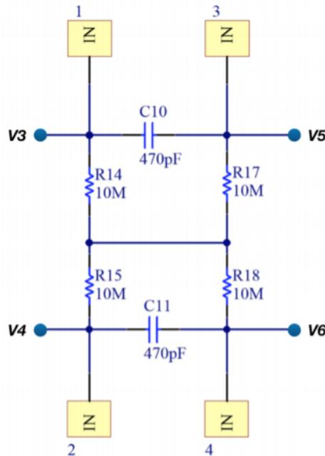
Figure 2.4. Second order passive High Pass Filter 33.86Hz
