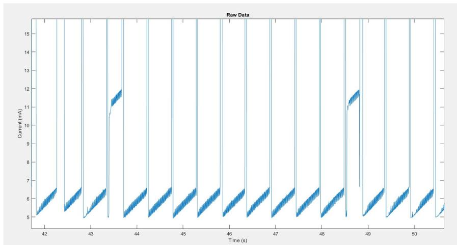
Figure 5.22. Power consumption analysis during Raw Data mode - Focus on the small peaks
