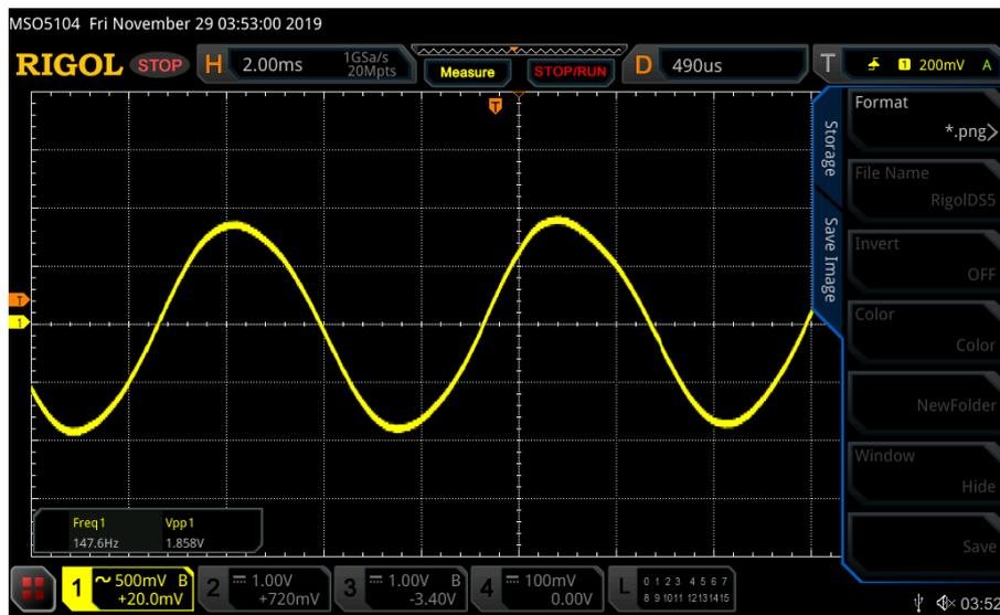
Figure 5.15. Gain 2500 test with hundreds of  $\mu V$  in INA differential input
