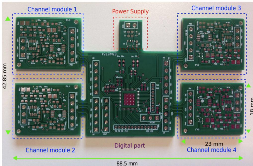
Figure 2.11. First acquisition system prototype
