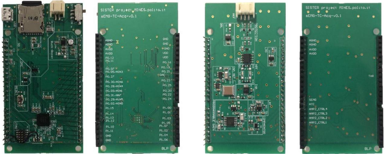
Figure 5.2. Main board top and bottom view Figure 5.3. AFE module top and bottom view
