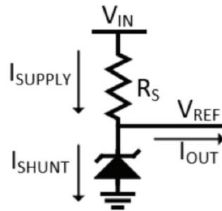
Figure 2.30. Shunt Voltage Reference structure
