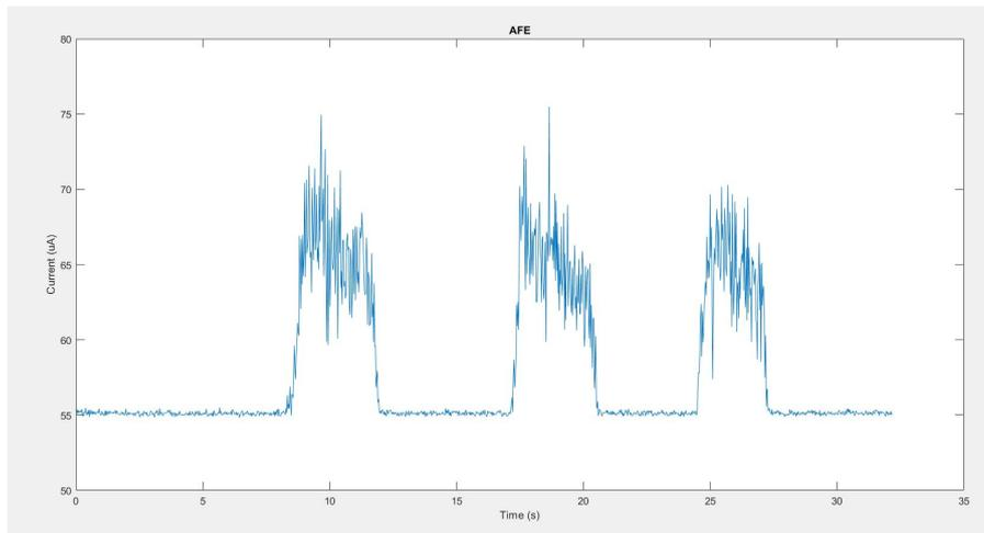
Figure 5.20. Analog Front End power consumption analysis during three maximal voluntary contractions
