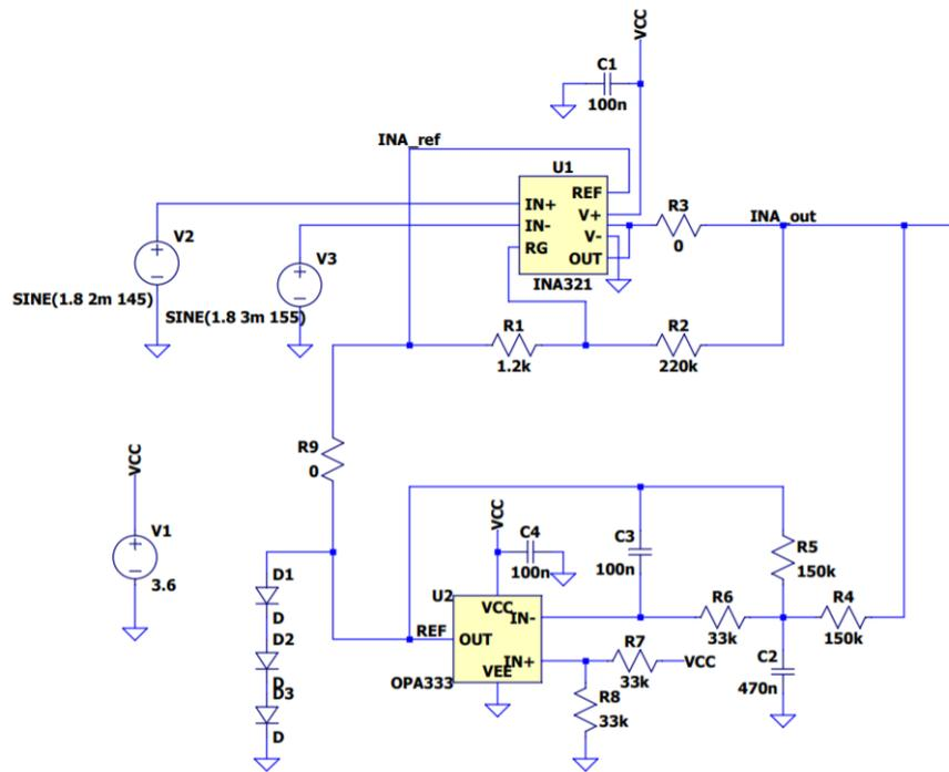
Figure 2.18. INA loop with parallel diodes to prevent the reference to exceed the safe range
