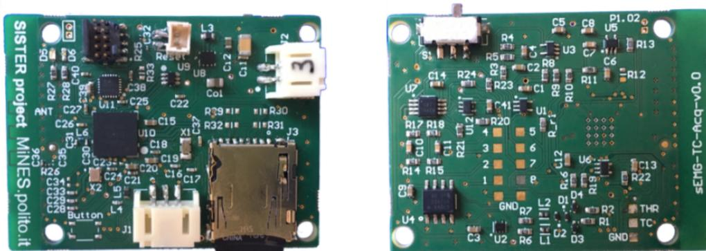
Figure 2.12. Mitor2 slave: Top side (*left*) is reserved for the digital part and bottom side (*right*) is reserved for the analog part
