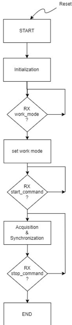
Figure 4.1. Slave High level flowchart
