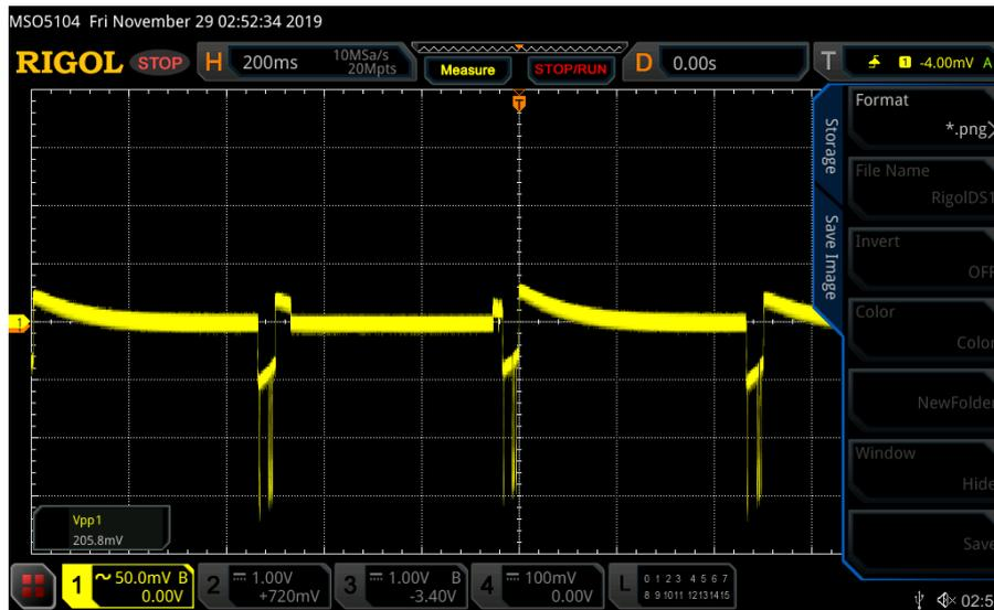
Figure 5.7. Dropout voltage on the battery terminals during the SD periodic writings in the new version of the system
