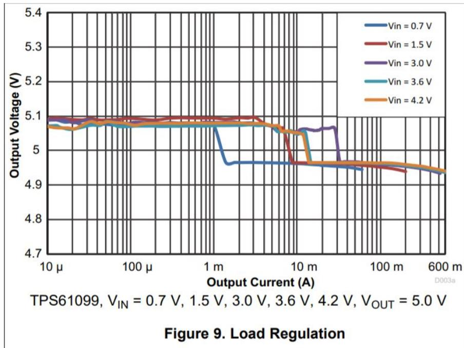
Figure 2.23. TPS61099x datasheet load regulation: Output Voltage vs Output Current
