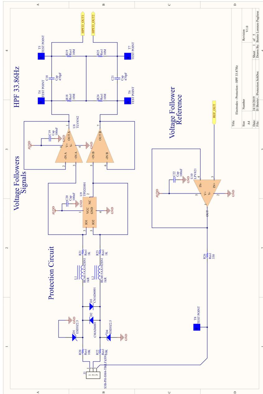
Figure 3.2. Input Stage Schematic: Protection Circuit; Buffers; 30Hz Differential High Pass Filter; Driven Right Leg Circuit
