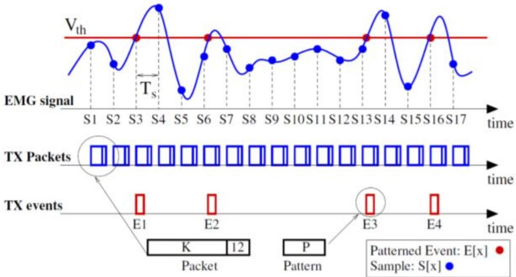
Figure 1.1. Amount of data comparison between the ATC technique and the classic approach
