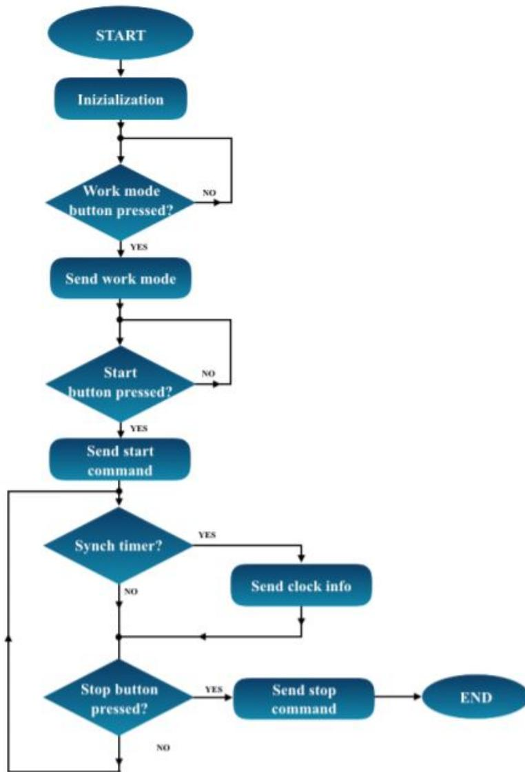
Figure 4.7. Master High Level flowchart
