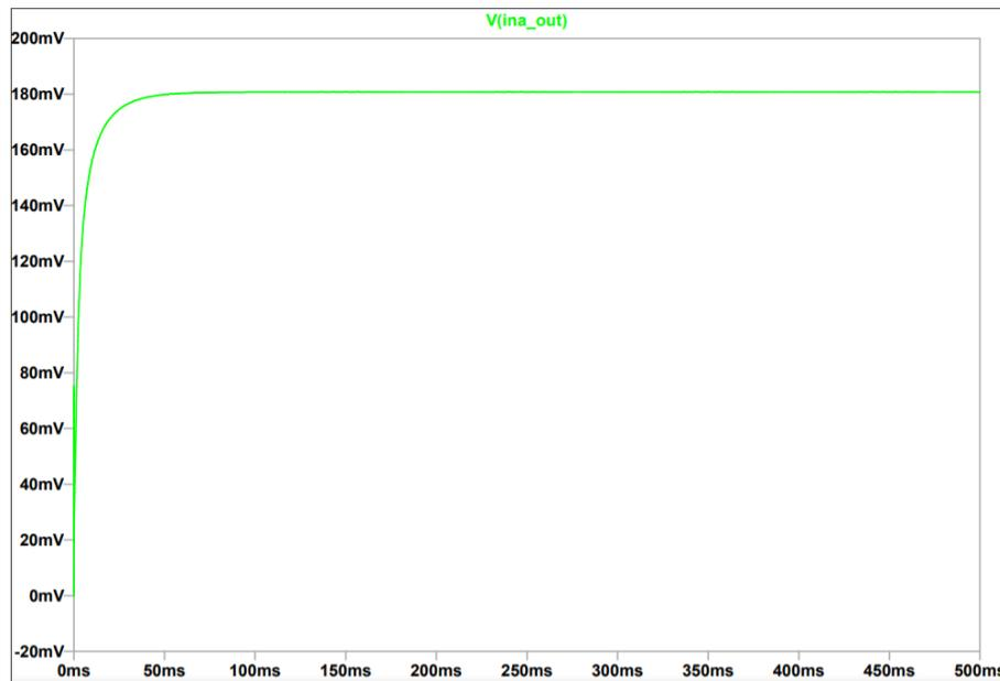
Figure 2.16. LTSpice INA output when reference forced to high voltage
