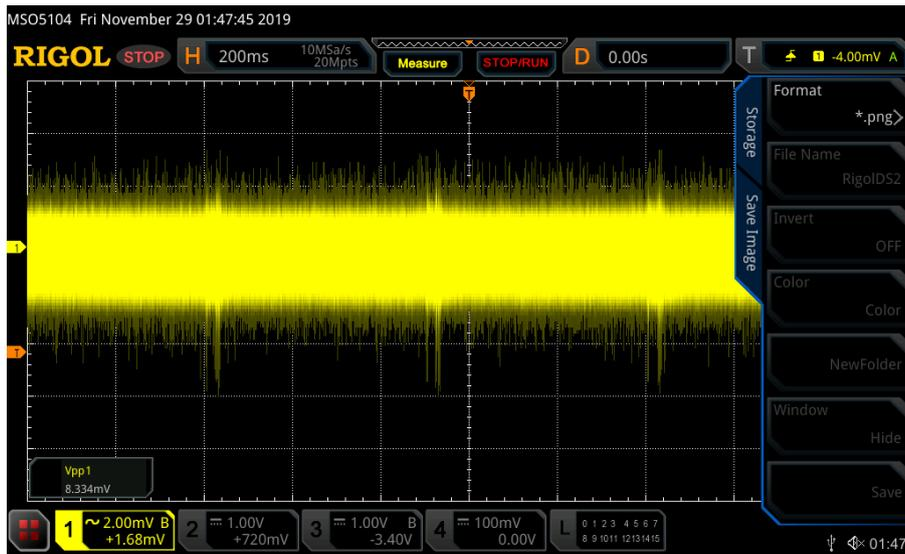
Figure 5.9. Dropout voltage on the acquisition channel LDO output during the SD periodic writings in the new version of the system
