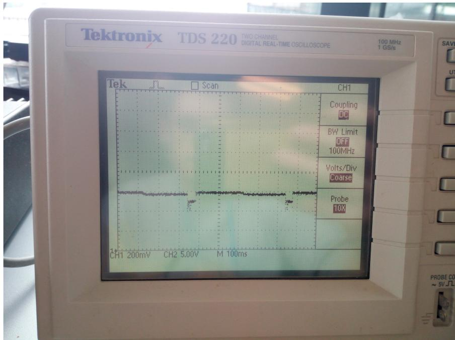
Figure 5.5. Dropout voltage on the INA reference during the SD periodic writings in the precedent versions of the system
