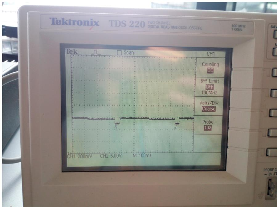
Figure 2.20. Dropout voltage on the INA reference during the SD periodic writings
