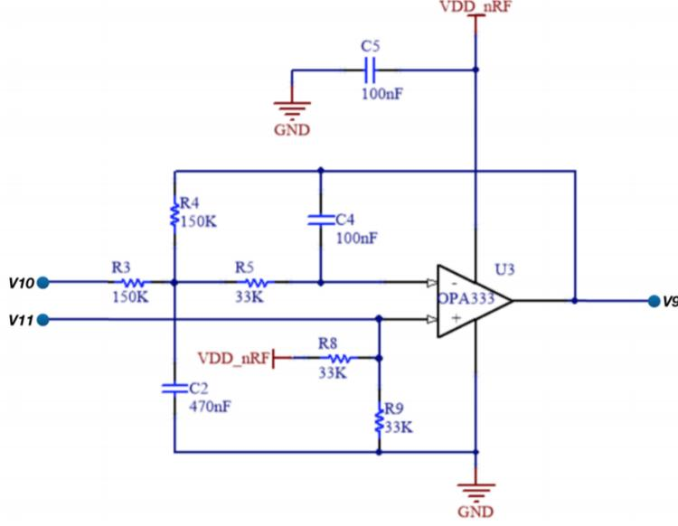
Figure 2.7. INA feedback and Low Pass Filter 10Hz for INA reference voltage generation
