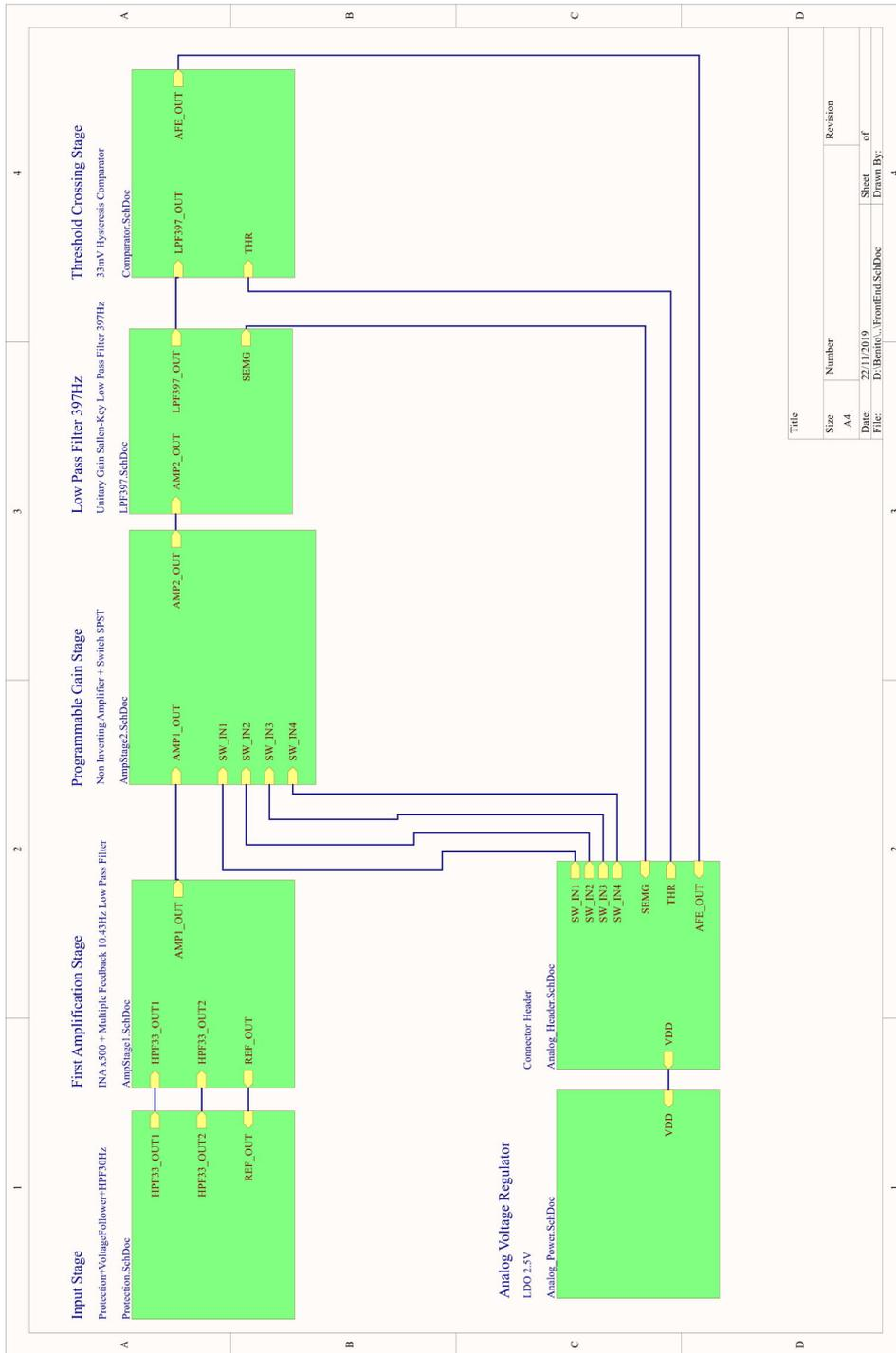
Figure 3.1. Analog Front End Module Block Scheme
