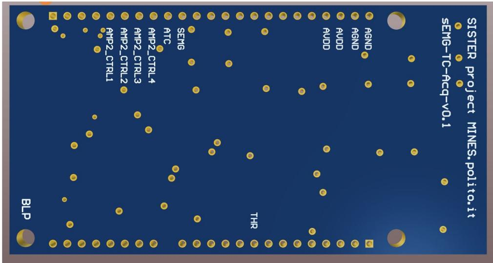
Figure 3.17. Analog Front End PCB 3D Bottom
