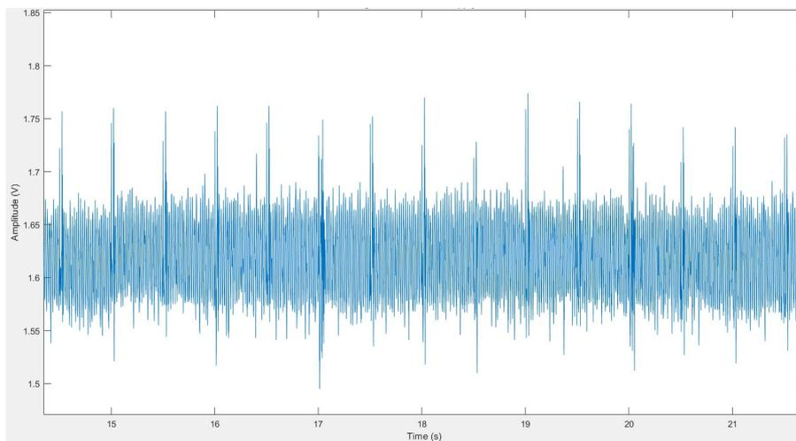
Figure 2.22. Baseline of sEMG signal acquired influenced by power supply dropout voltage during the periodic SD writings
