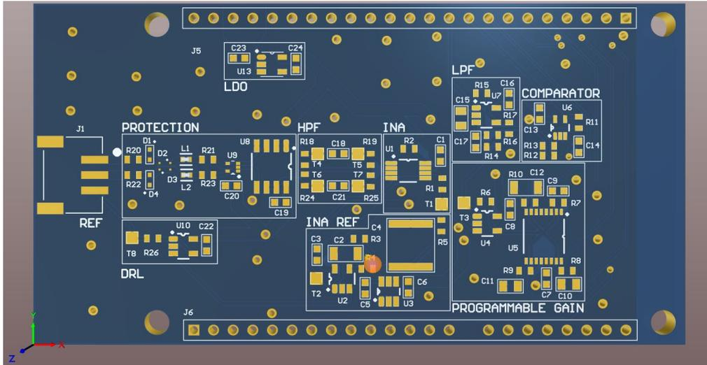
Figure 3.16. Analog Front End PCB 3D Top
