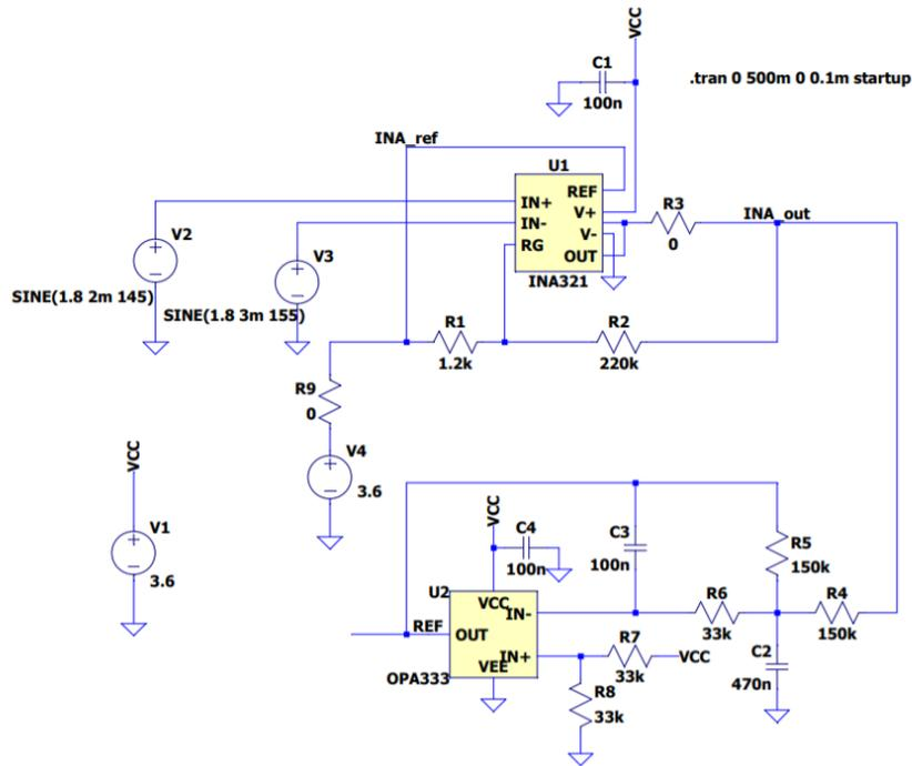
Figure 2.15. INA loop with INA reference forced to high voltage
