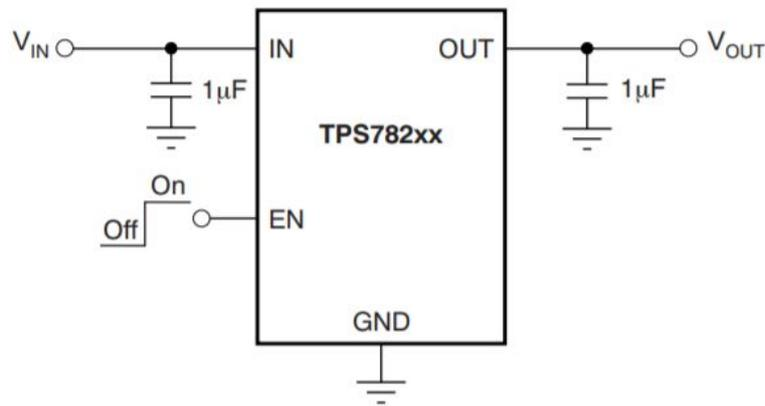
Figure 2.31. Low Drop Out voltage regulator
