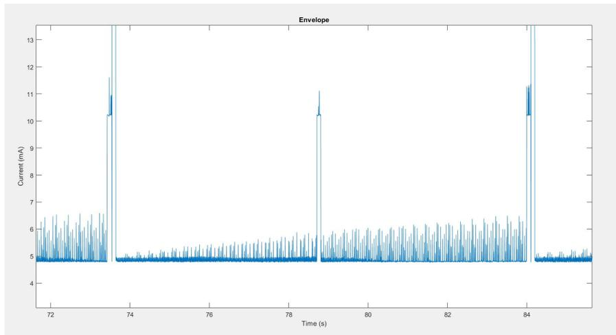
Figure 5.24. Power consumption analysis during Envelope mode - Focus on the small peaks
