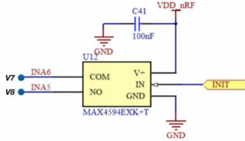
Figure 2.6. Analog Switch between INA reference and output
