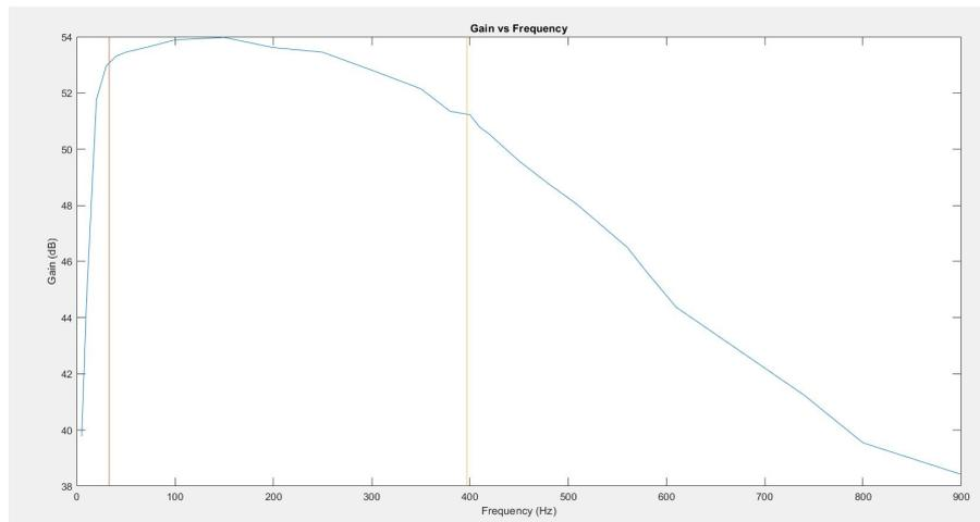
Figure 5.11. Gain variation with respect to the input signal frequency. Gain of the acquisition channel is set to 500.
