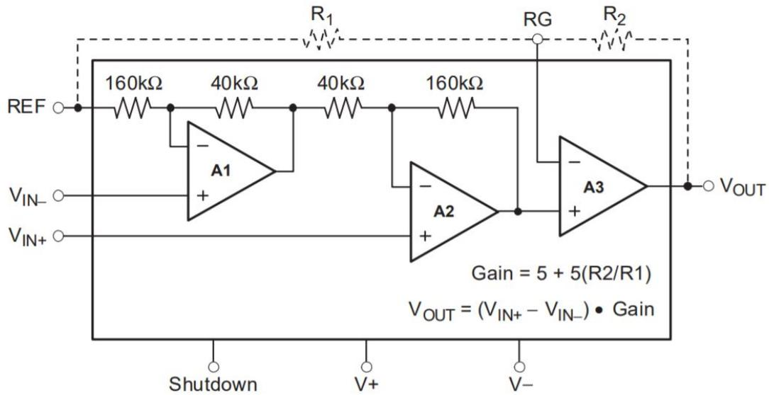
Figure 2.26. INA321 internal structure and gain
