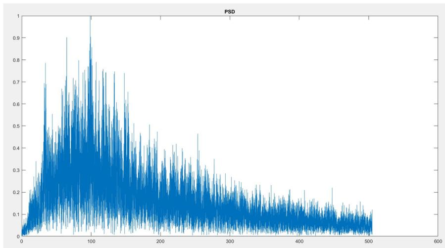
Figure 2.41. Power Spectral Density signals acquired and processed by the breadboard, sampled by the MSP430 and graphed with Matlab during 14 gaits
