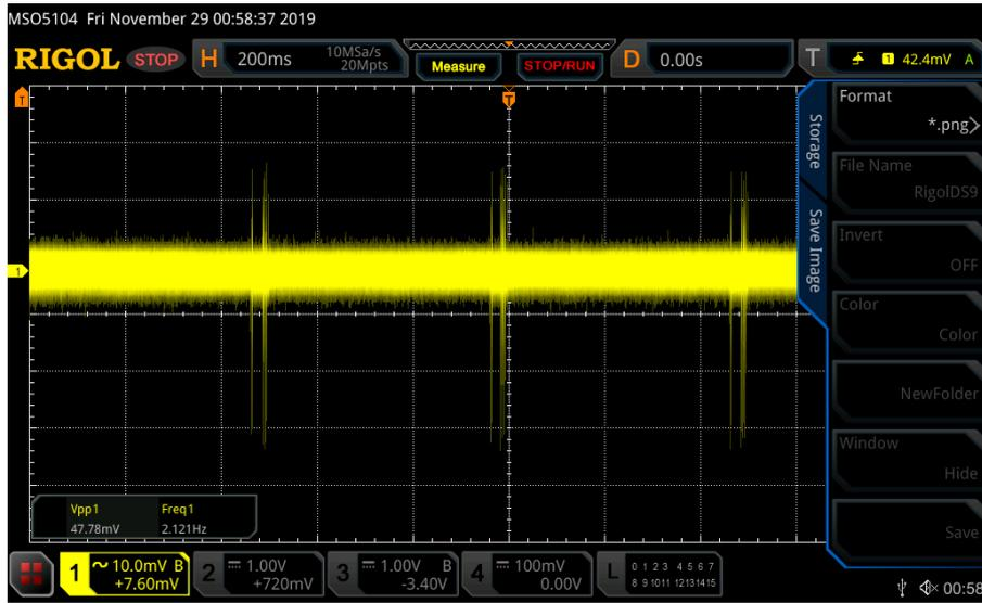
Figure 5.8. Dropout voltage on the buck-boost output during the SD periodic writings in the new version of the system
