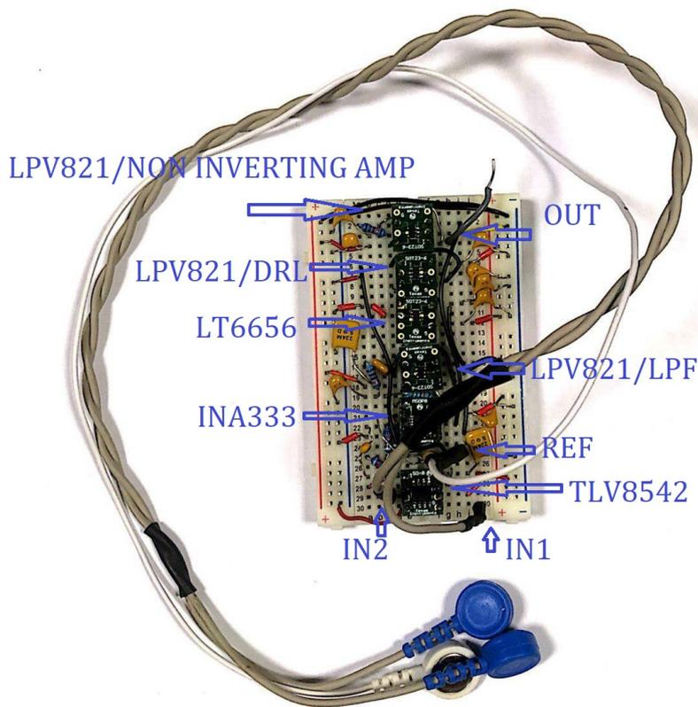
Figure 2.37. Analog Acquisition Channel Breadboard Prototype
