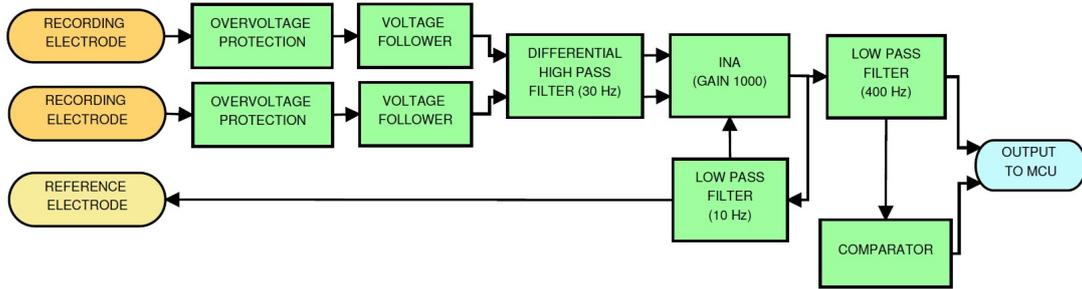
Figure 2.1. Mitor2 Analog Front End block scheme
