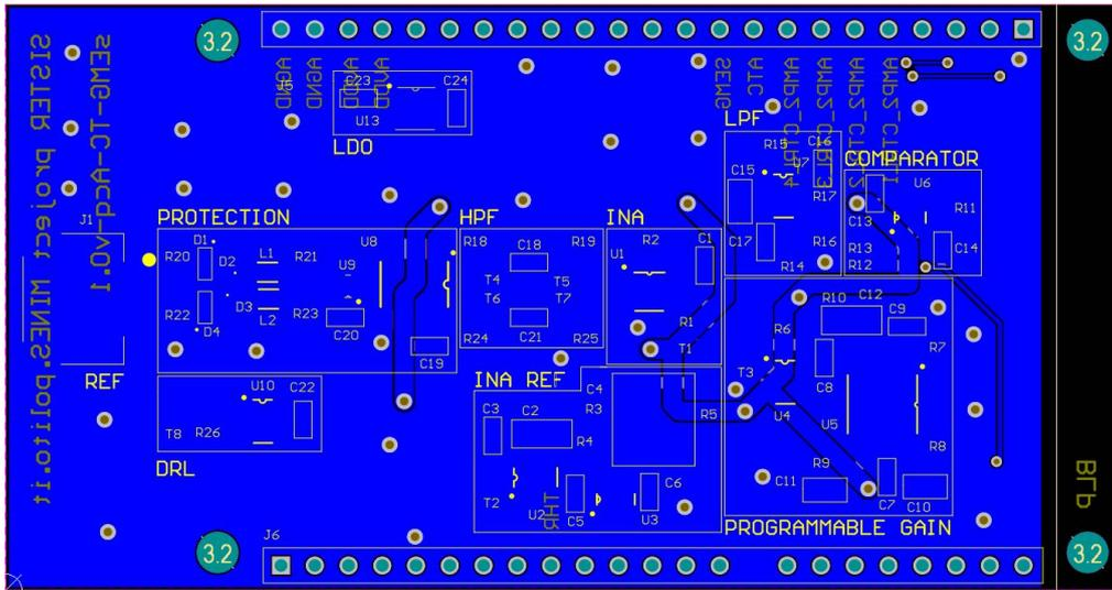
Figure 3.15. Analog Front End PCB Bottom
