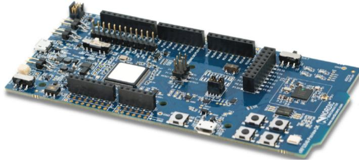
Figure 1.6. nRF52840 Development Kit by Nordic Semiconductor
