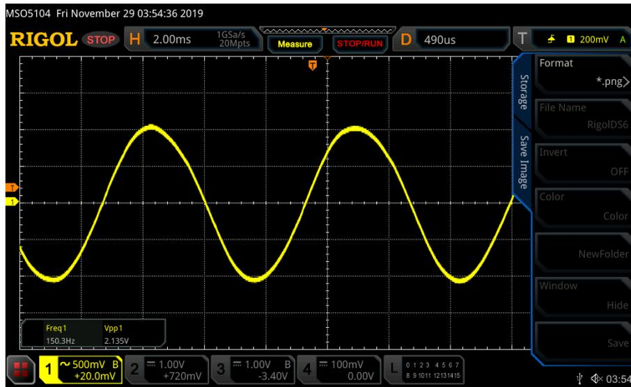
Figure 5.16. Gain 3000 test with hundreds of  $\mu V$  in INA differential input
