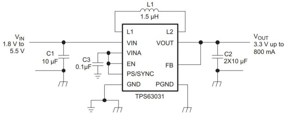
Figure 2.32. Buck-Boost voltage regulator
