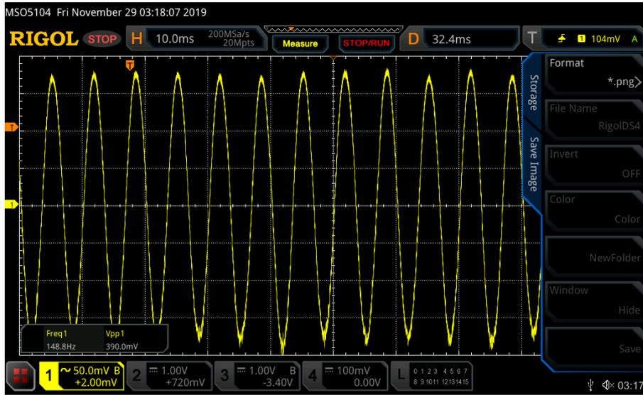
Figure 5.12. Gain 500 test with hundreds of  $\mu V$  in INA differential input
