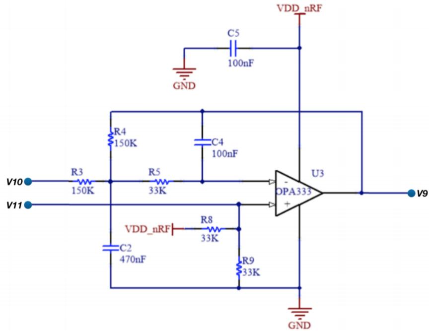
Figure 2.21. Focus on the voltage divider R8,R9 for the INA voltage reference generation
