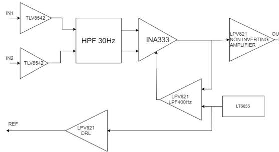
Figure 2.36. Breadboard Prototype Analog Acquisition Channel
