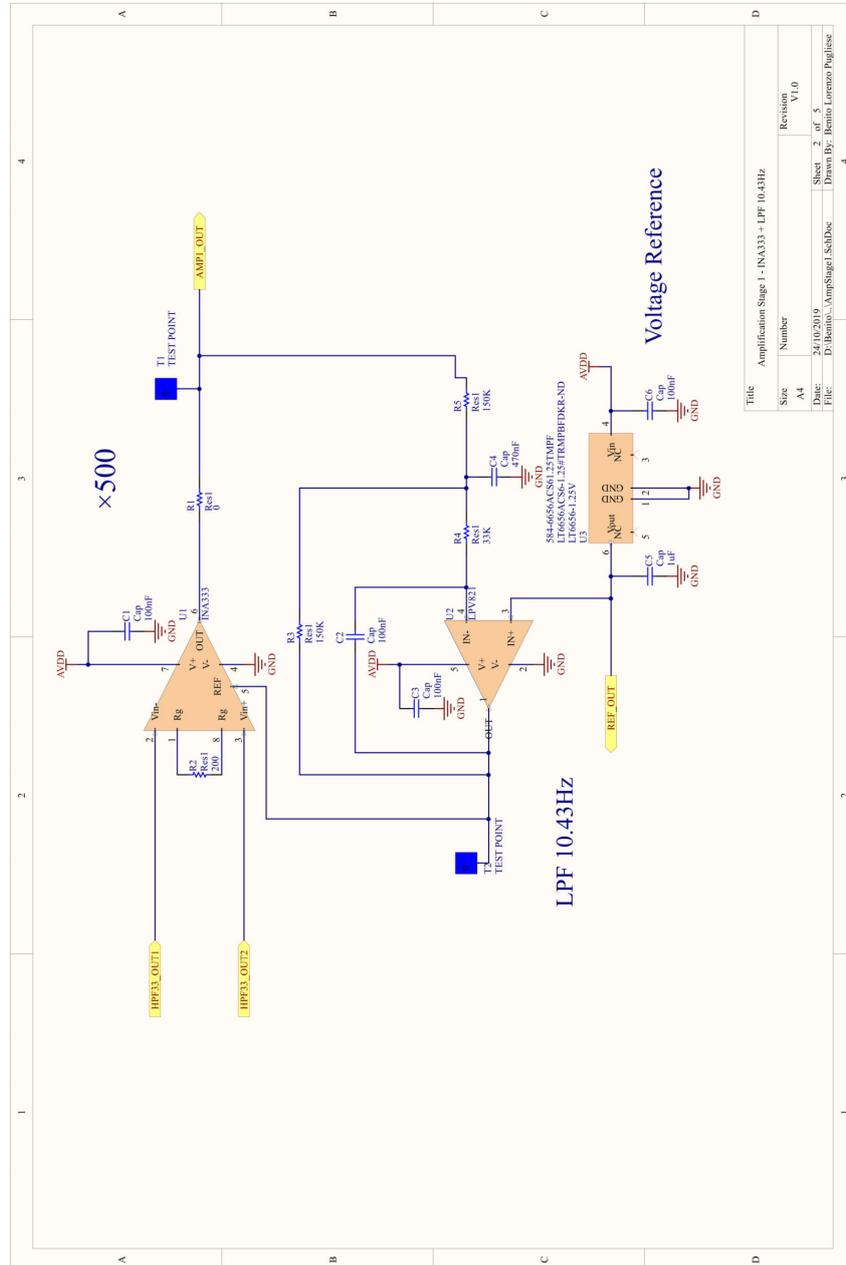
Figure 3.3. First Amplification Stage: 500 Gain Instrumentation Amplifier; Feedback 10Hz Low Pass Filter; 1.25V Voltage Reference
