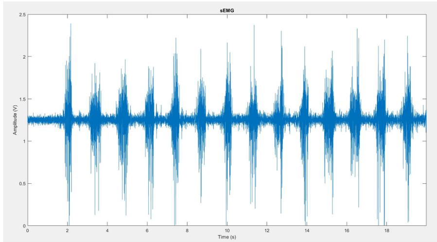
Figure 2.40. Gastrocnemio Medialis sEMG signals acquired and processed by the breadboard, sampled by the MSP430 and graphed with Matlab during 14 gaits
