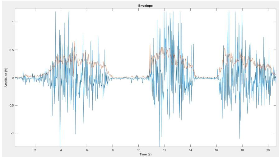
Figure 5.18. Wrist extension acquired in Envelope mode
