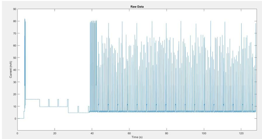
Figure 5.21. Power consumption analysis during Raw Data mode
