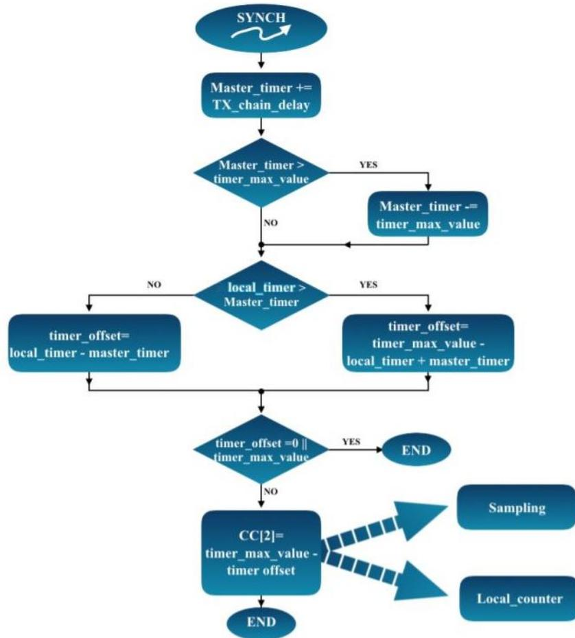
Figure 4.6. Slaves Synchronization flowchart
