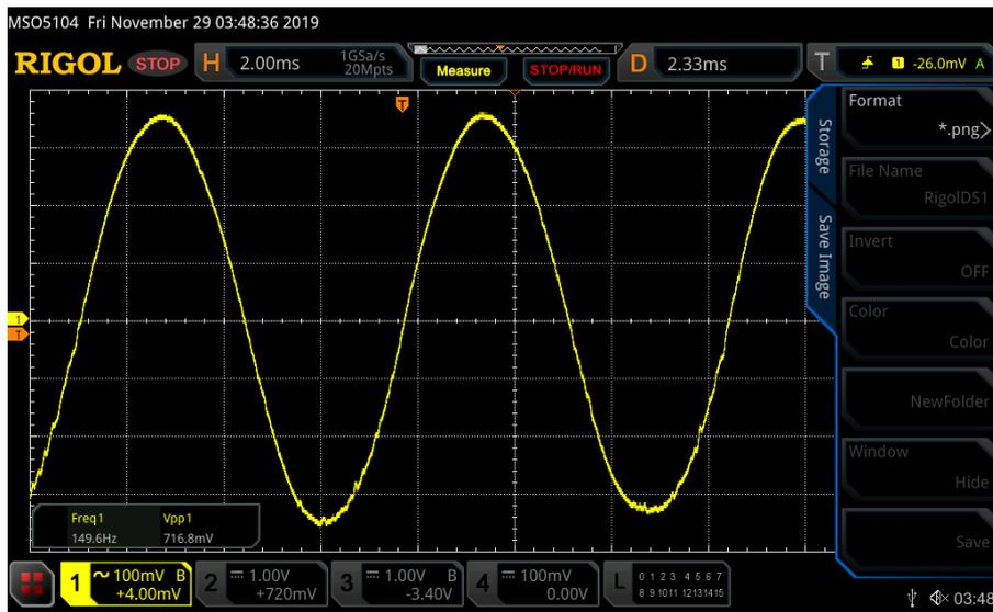
Figure 5.13. Gain 1000 test with hundreds of  $\mu V$  in INA differential input
