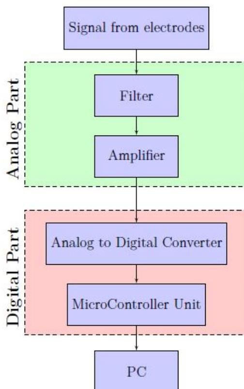
Figure 1.2. Standard structure of sEMG acquisition chain
