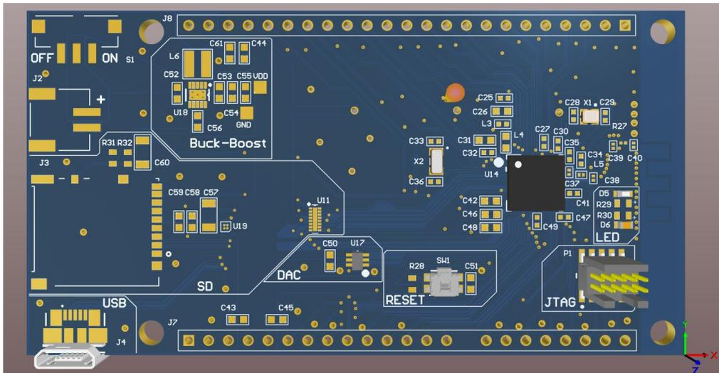
Figure 3.20. Main Board End PCB 3D Top
