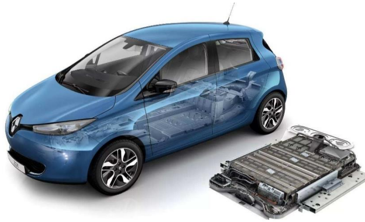
Figure 3.2 41 kWh Renault Zoe R110 Z.E. 40 battery pack (Photo by Mark Kane)
