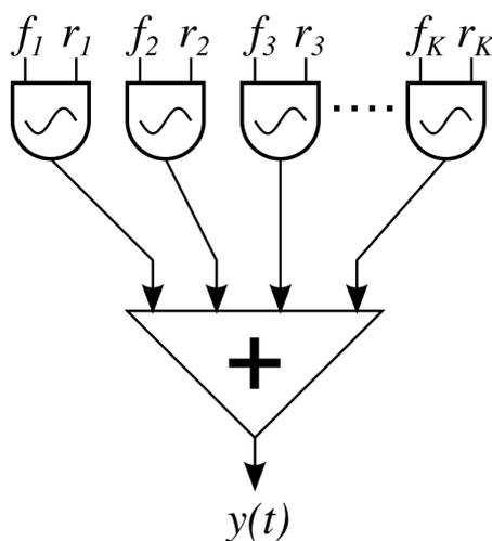
Additive synthesis uses exactly this mechanism to imitate the sound of any musical instrument. The output of several oscillators, modulated and adjusted according to the Fourier decomposition is combined to generate the final output [36]. In this way it is possible to reproduce the waveform corresponding to the timbre of the specific instrument, thus emulating its sound.
