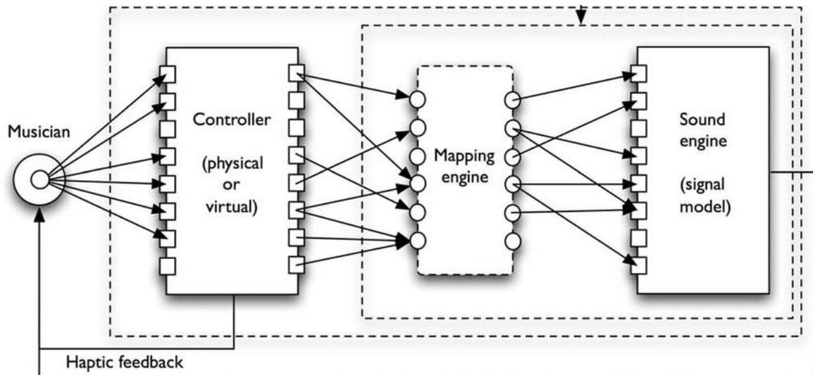
Figure 5.5. Typical structure of a DMI interface (Wanderley 2000; Leman 2008; Wessel and Wright 2001), divided into gesture controllers, sound engine and mapping. Figure taken from "Designing Constraints: Composing and Performing with Digital Musical Systems" by Thor Magnusson.
