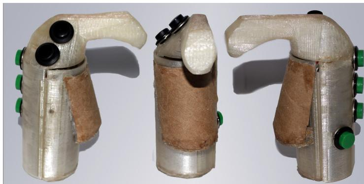
was used to correct the DMI model dimension. The Blender model was then printed out in 3D. The DMI circuit, designed in KiCAD, is made of three components: an accelerometer (MPU6050) used to modulate the Velocity of our DMI, the microcontroller (Arduino Nano) and the six buttons. The audio synthesis engine and the mapping strategy used for this project has been programmed Pure Data<sup>6</sup>.
