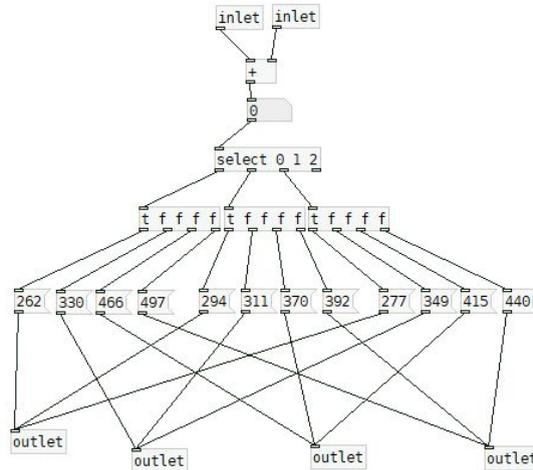
Figures 6.13. Output note selection function. Depending on the status selected by the Status Buttons (SWA1 e SWB1), this function assigns to each Note Button the pitch to be played.
