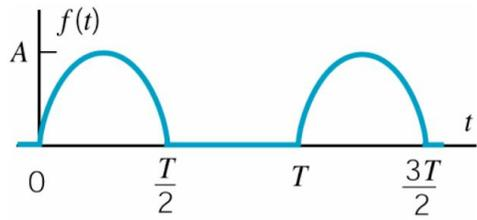
Half wave rectified sine wave:  $\omega_0 = \frac{2\pi}{T}$
