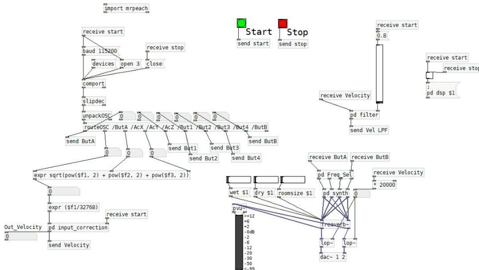
Figures 6.9. The Main project program of the mapping between the electronics and the sound synthesis.
