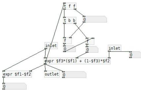
Figure 6.12. Input Filtering Function. Using a prediction filter.
