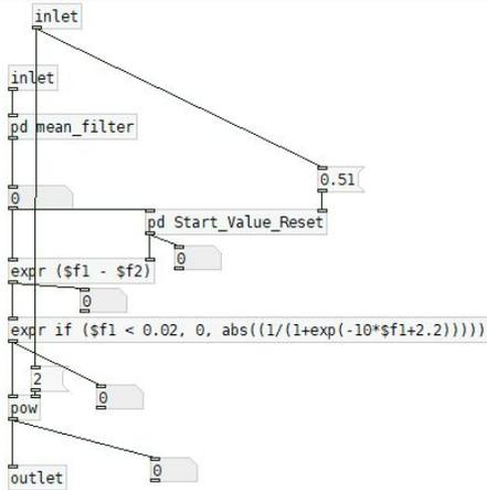
Figures 6.10. Input correction function. Used to stabilize the input, as a noise gate and has a non-linear mapping function.
