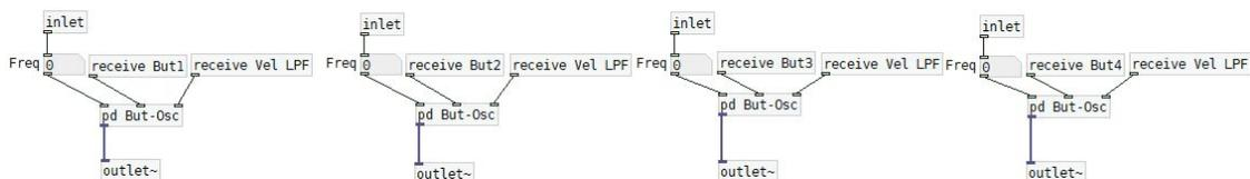
Figure 6.14. Output note assignment function. Assigns to the four oscillators the frequency they will play at.
