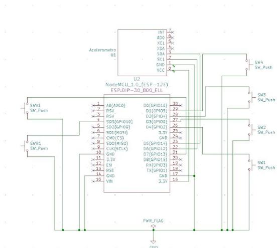
Figure 6.4. Wiring diagram of the components, Image created from the KiCAD software. From the top left the selection buttons SWA1 and SWB1, from the top right the note buttons SW4, SW3, SW2, SW1.
