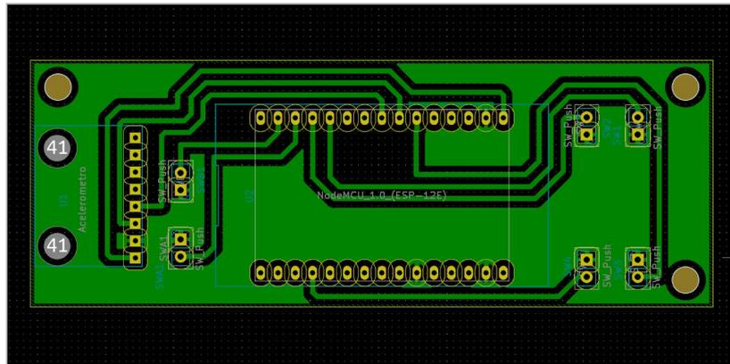
Figure 6.5. PCB tracks, designed in KiCAD.
