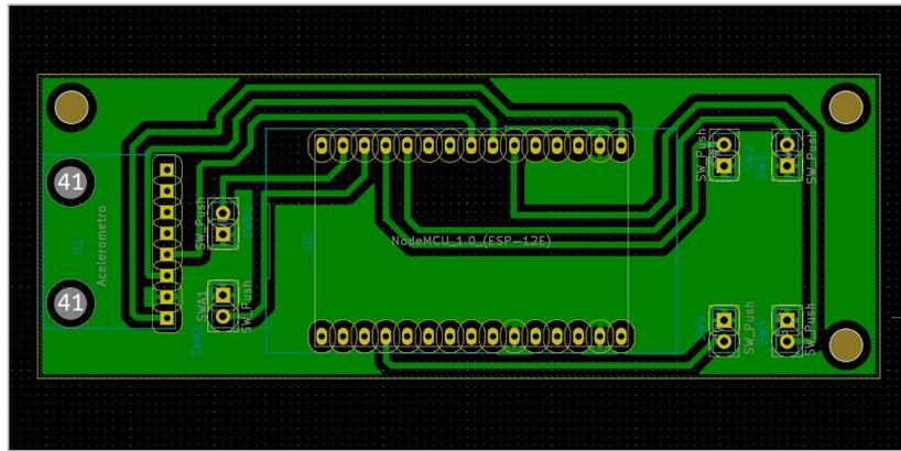
Figure 6.5. PCB tracks, designed in KiCAD.
