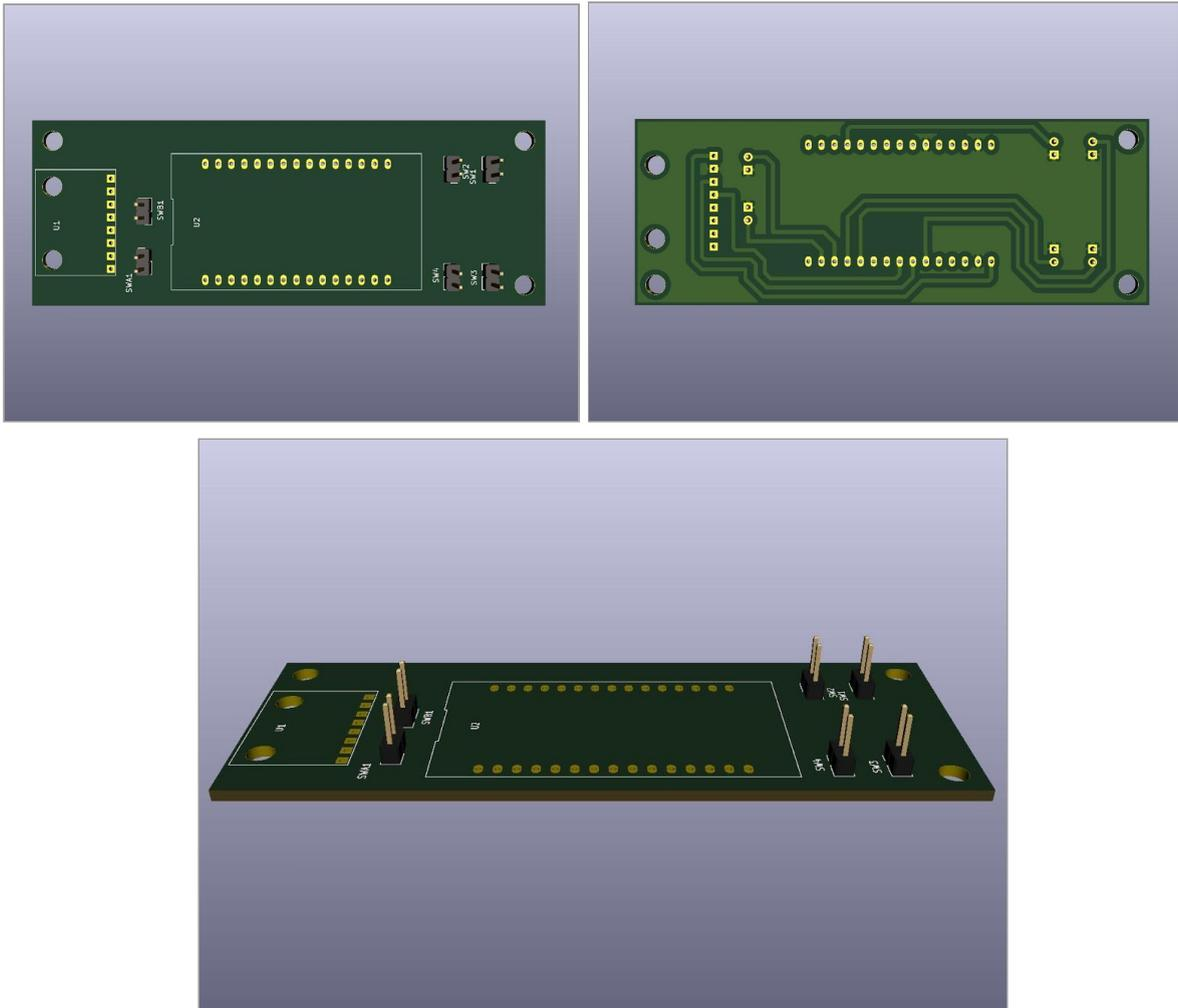
Figure 6.7. Front (a), Back (b) and lateral (c) view of the PCB 3D model.
