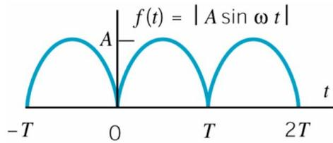
Full wave rectified sine wave:  $\omega_0 = \frac{2\pi}{T}$
