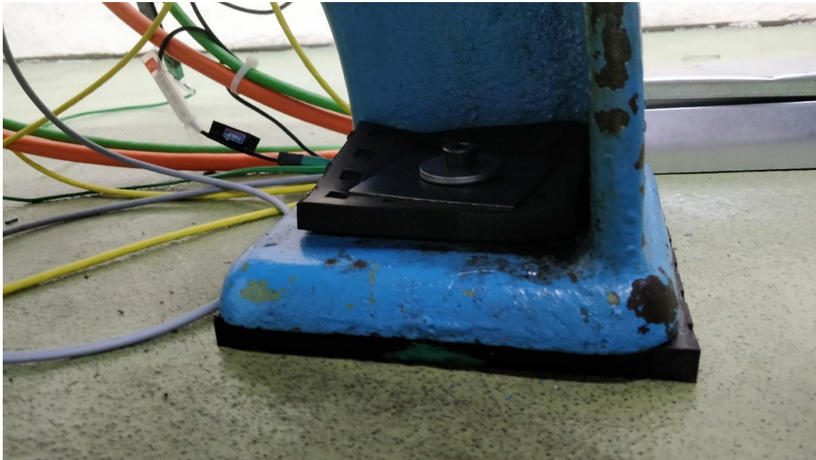
Figure 65 Test rig feet with isolation mats
