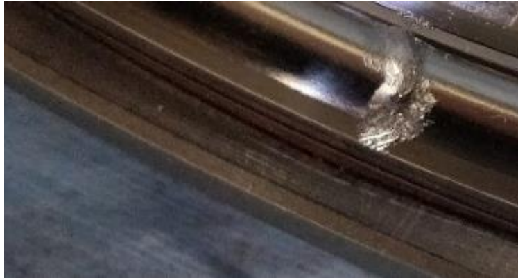
Figure 47 Artificial damage to ACBB outer ring
