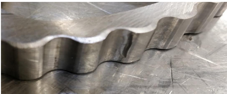
Figure 49 Artificial Damage on to Disk undulations
