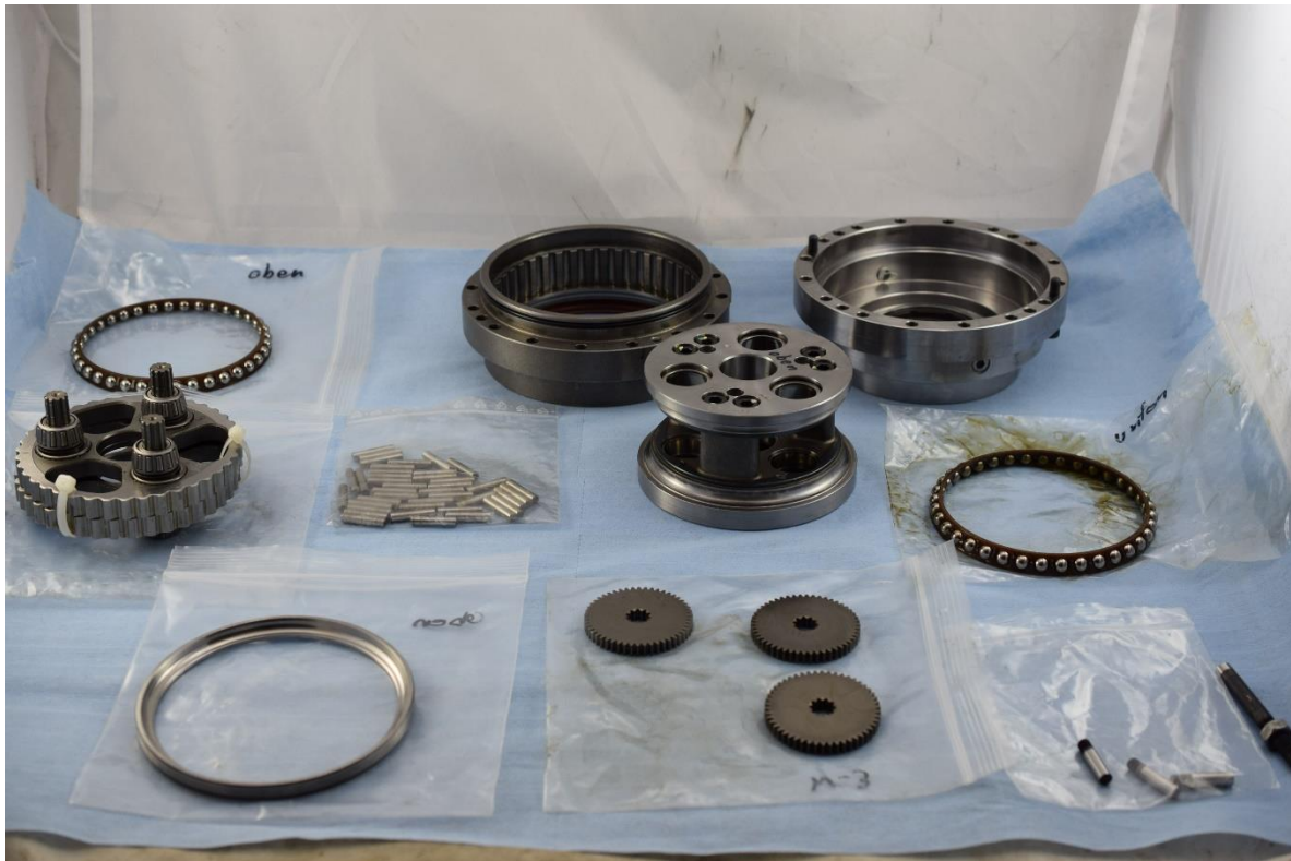
Figure 44 Dismantled Nabtesco RV-42N
