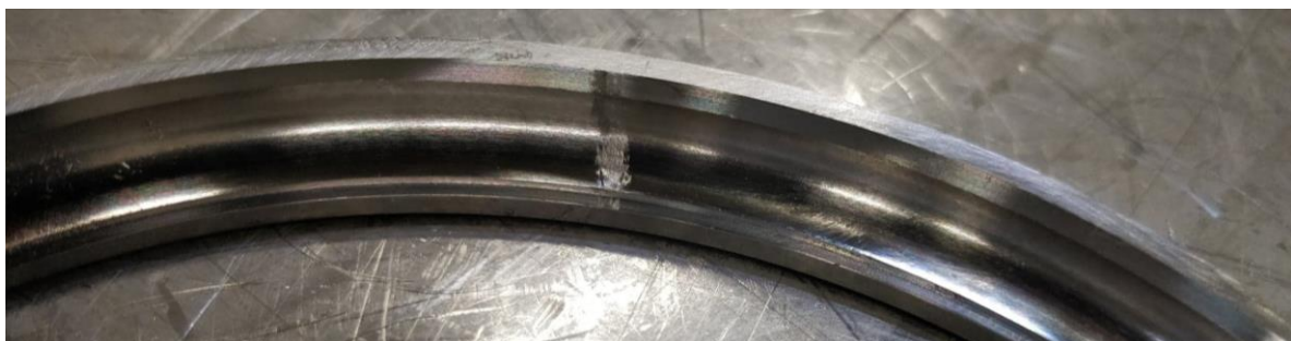
Figure 64 Initial Damage on ACBB outer ring
