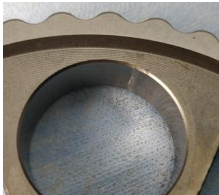
Figure 63 Initial Damage on the integrated CRB outer ring
