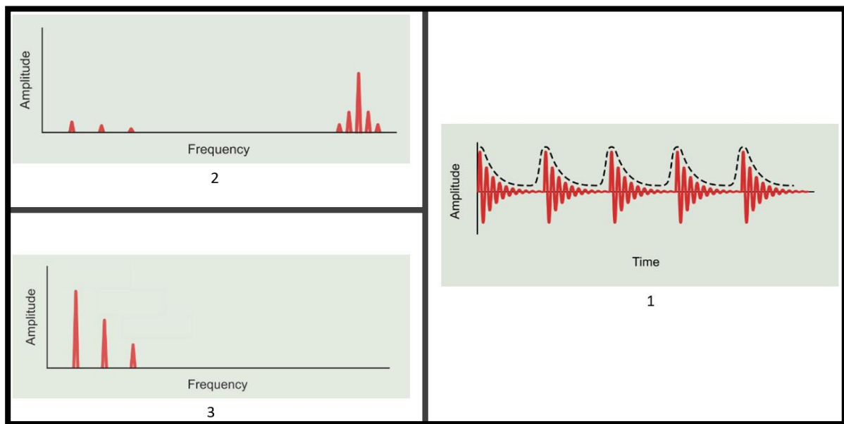
Figure 24 Image 1: Red is raw vibration signal and dotted is the enveloped signal Image 2: Frequency spectrum of raw signal Image 3: Frequency spectrum of enveloped signal [30]
