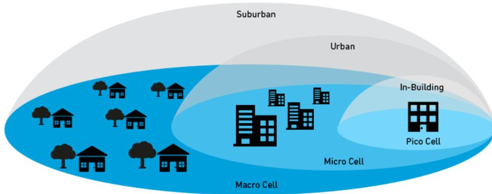
Figure 1.3: Coverage area for cells using different technologies
