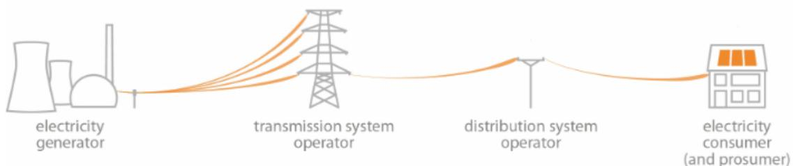
Figure 1.1: Power network structure
