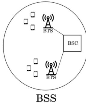
Figure 1.2: Portion of the cellular network composed of a single BSS and multiple BTS
