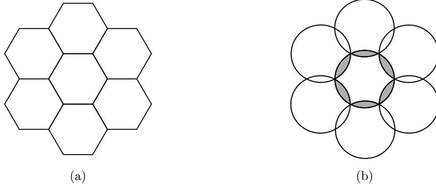
Figure 1.4: BTS transmission and interference area
