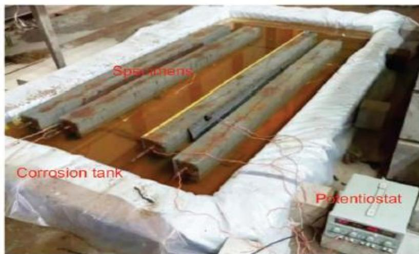
**Figure 5.2 Accelerated corrosion device [1]**
