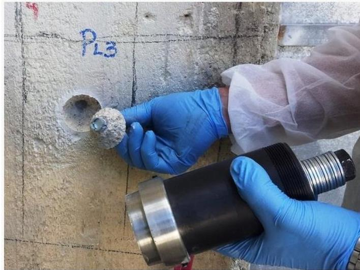
Figure 3.7 Pull-out test [15]
