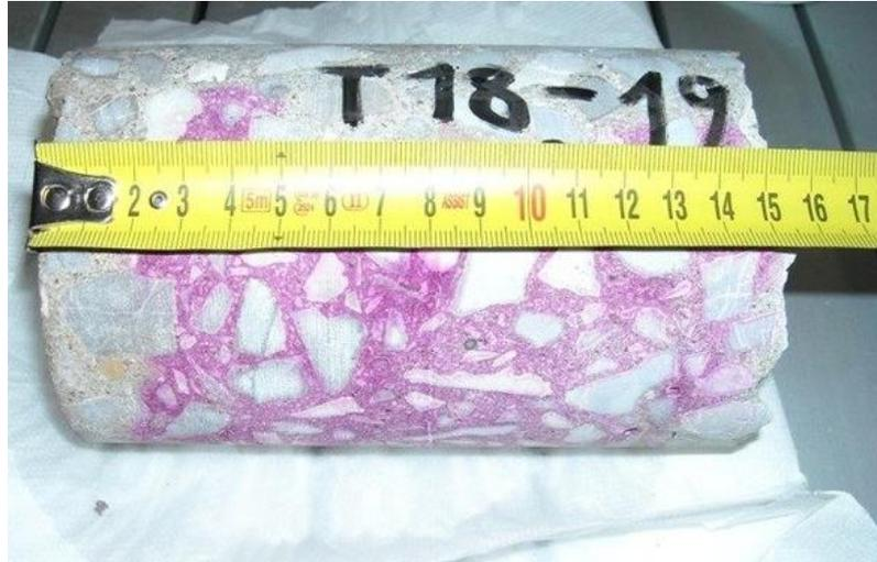
**Figure 2.4 Determination of the carbonated front using the phenolphthalein test**
