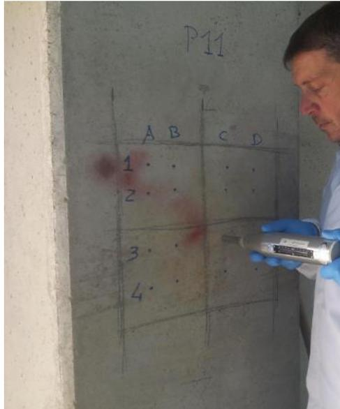
Figure 3.3 Sclerometric tests [15]
