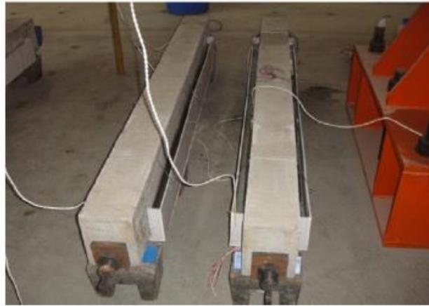
Figure 4.5 Accelerated corrosion test of beams [4]
