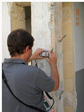
Figure 3.5 Pacometric test [15]
