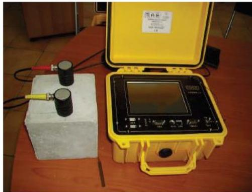
Figure 3.4 Ultrasonic tests performed on the specimens [15]
