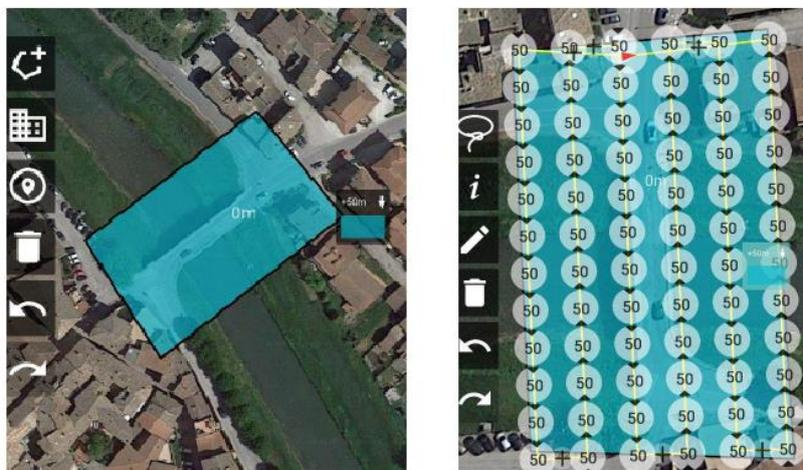
Figure 3.29 Flight plan for a height of 50 meters
