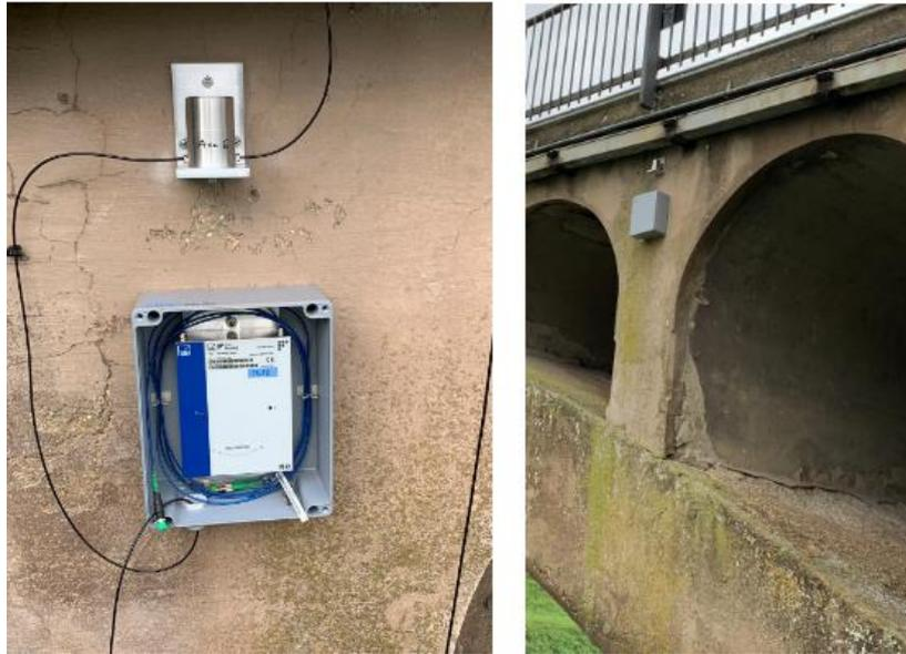
*Figure 3.50 Accelerometer 6 and tilt meter 2 on the left and accelerometer 4 and tilt 7 on the right*
