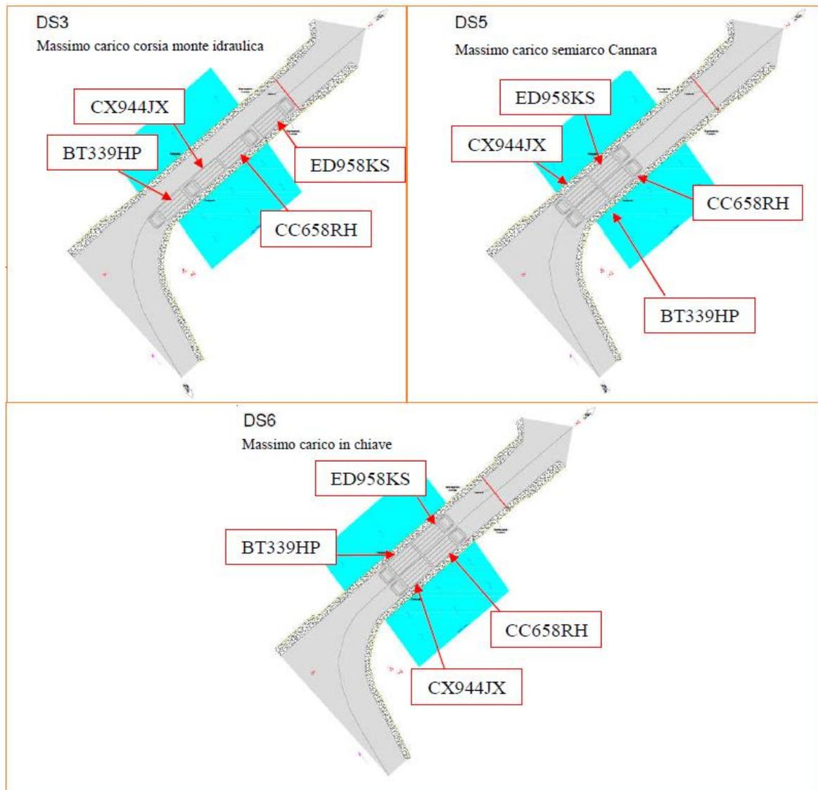
Figure 3.14 Load test configurations
