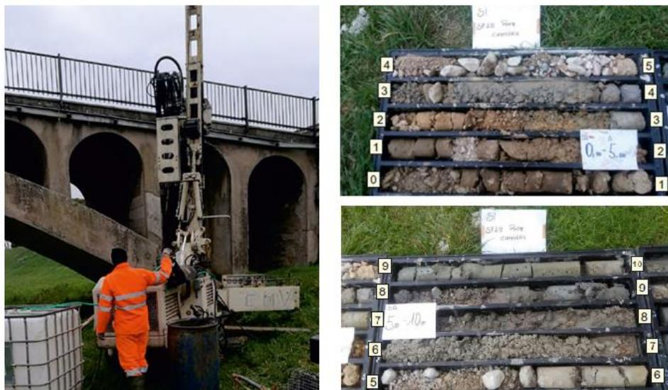
Figure 3.22 Cataloging boxe relative to specimen S1
