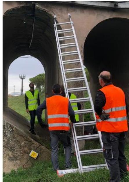
Figure 3.54 Installation of Acc1 with basket on the left and the ladder used to install sensors on the right
