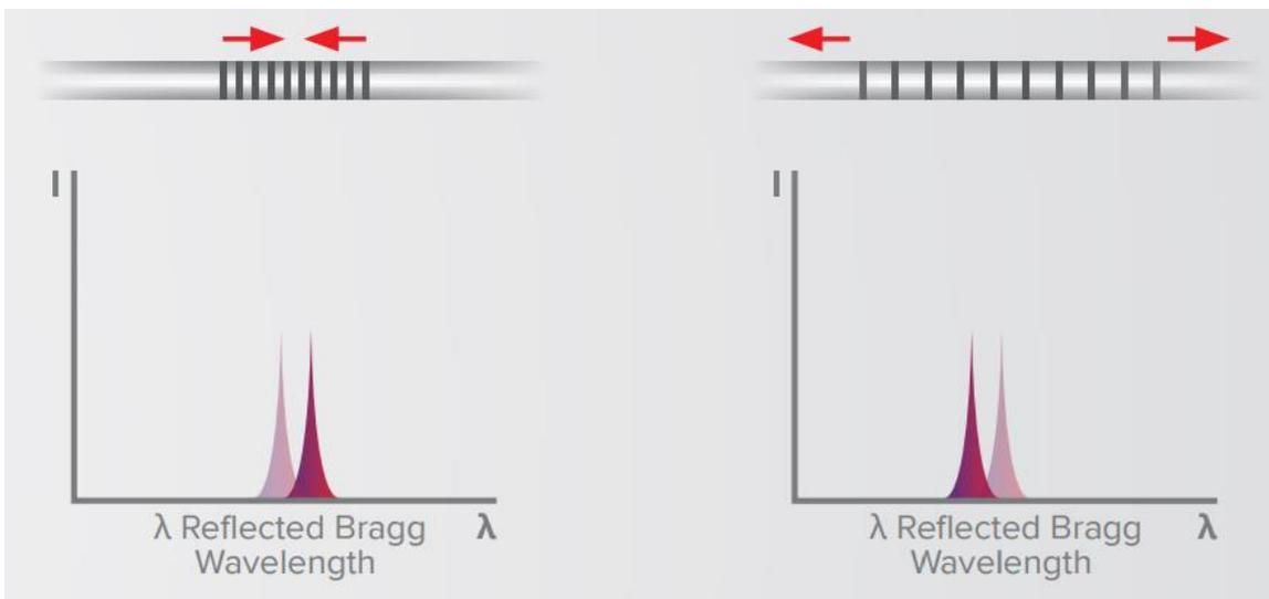
*Figure 2.6 Application of tension and compression in a fiber with a FBG sensor*
