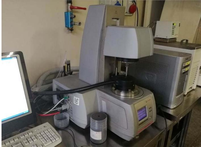
Figura 4.21 Dynamic Shear Rheometer
