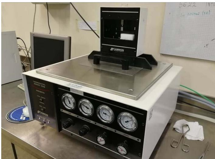
Figura 4.14 Bending Beam Rheometer
