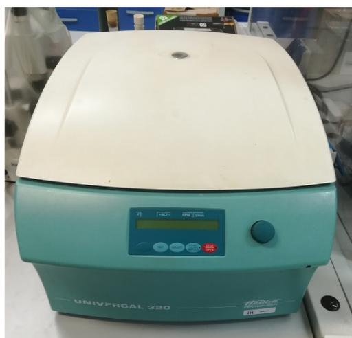
Figure 3.4: The centrifuge machine used for collecting and washing step, a UNIVERSAL 320 Hettich, Andreas Hettich GmbH &amp; Co. KG.
