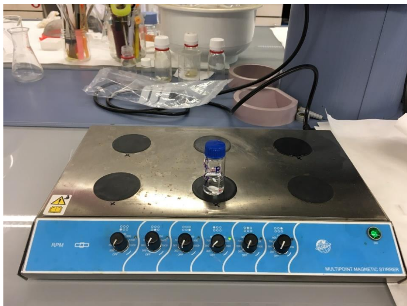
Figure 15. Magnetic stirring set up for preparing copolymer solutions
