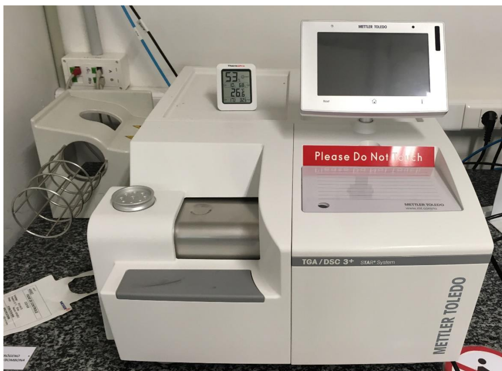
Figure 19. Experimental set up used for thermal analysis
