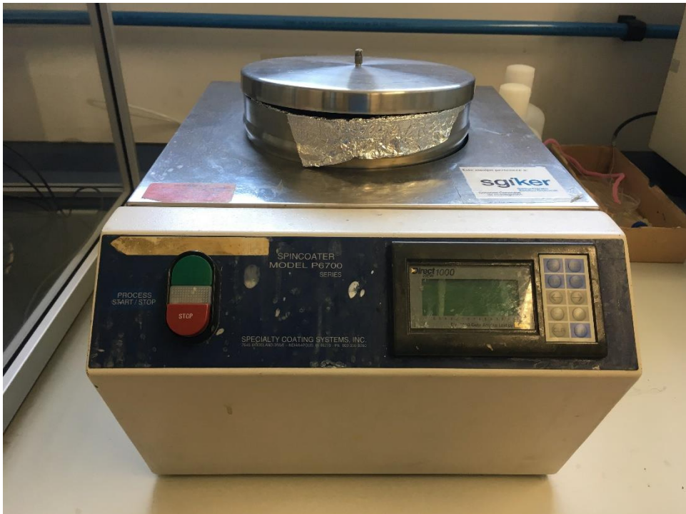
Figure 16. The spin coating set up used in this work
