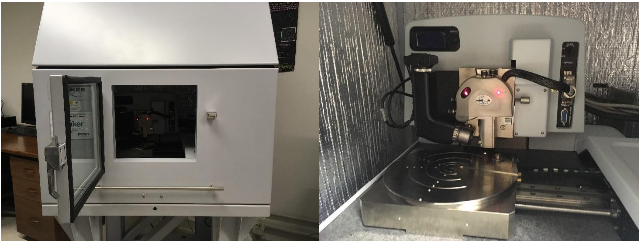
Figure 20. A picture of the AFM equipment used in this work. On the left the whole instrument, on the right a zoom of the sample holder and the tip.
