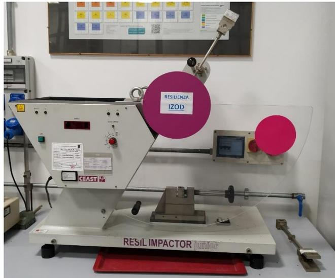
**Figura 3.14:** Instron 6963 Resil Impactor JR.
