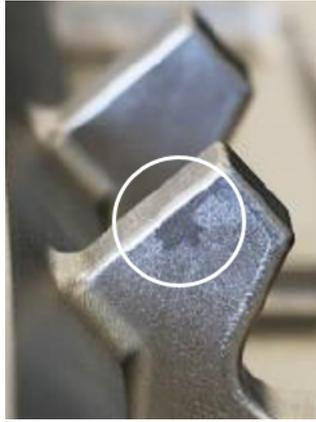
**Figure 1.3:** Foreign grain marked on a component, made of MAR M 247, visualized after etching. The Foreign grain is spontaneously nucleated on the surface of the component during solidification. The different crystallographic orientation is clearly visible due to the different colors between the grain marked with the white circle and the remaining part of the component [2].
