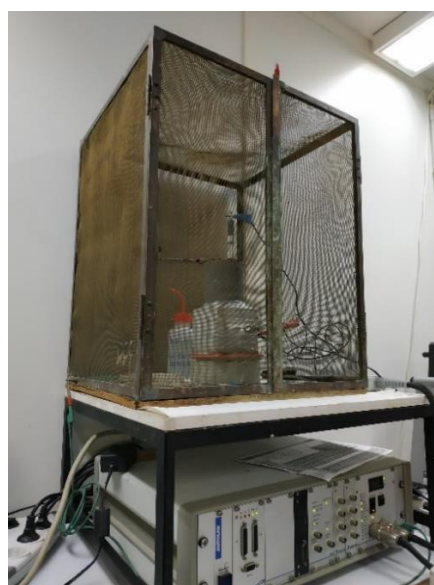
Figure 4.12: Autolab device and electrochemical cell.
