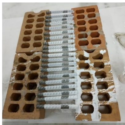
Figure 4.2: Epoxy-resin coated 2304 DSS tested rebars.
