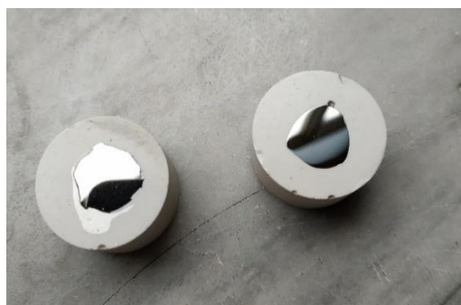
Figure 4.19: incorporated DSS 2304 corroded and not-corroded rebars after polishing..
