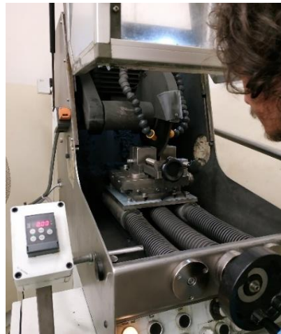
Figure 4.18: DSS 2304 rebar cutting step.
