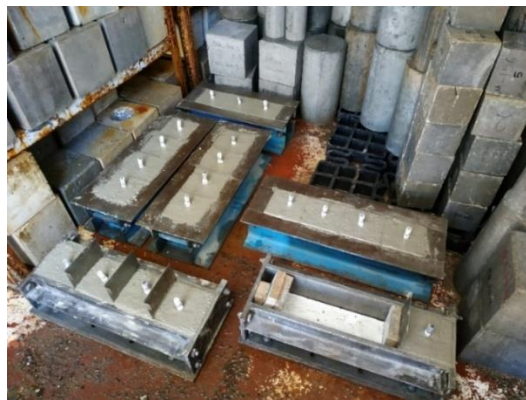
Figure 4.6: Tested samples left in humid chamber for solidification.
