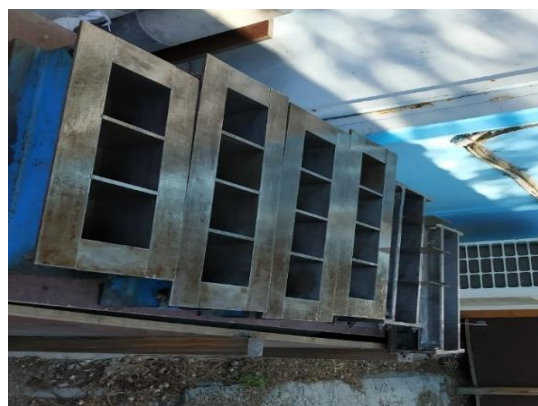
Figure 4.4: Steel moulds used for the samples preparation.
