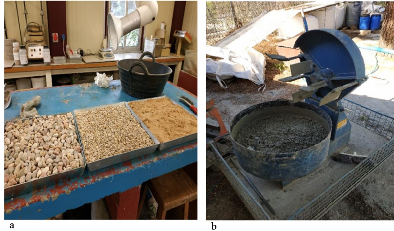
Figure 4.3: a) Three different types of aggregates used for the concrete; b) Final concrete mixture.
