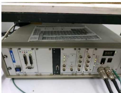
Figure 3.7: Metrohm Autolab PGSTAT30 used for the testing.
