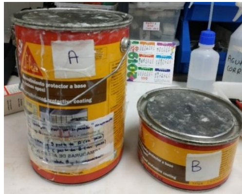
Figure 3.4: Epoxy resins as result of a mixture of Type A and Type B.
