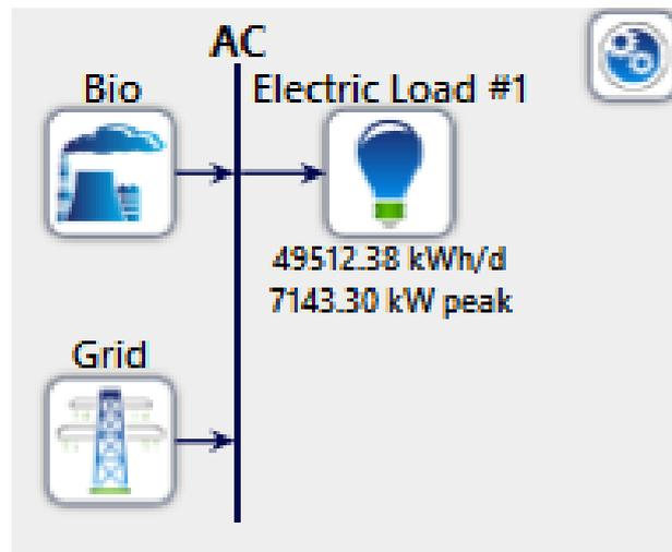
Figure 18 - First configuration: biogas genset
