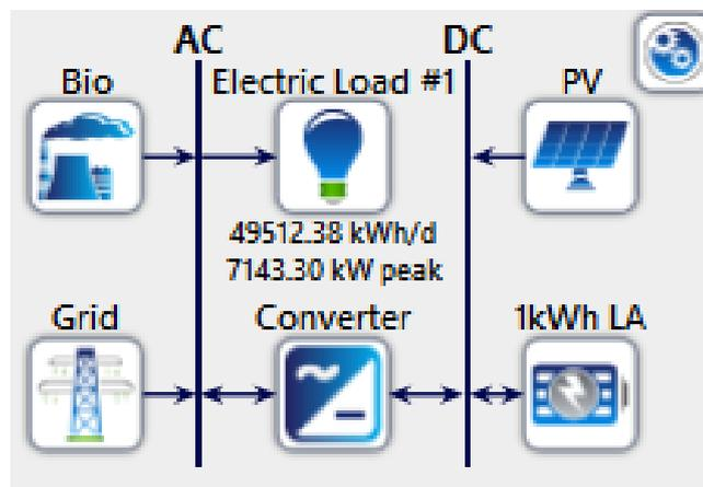
Figure 19 - Second configuration: biogas genset plus PV
