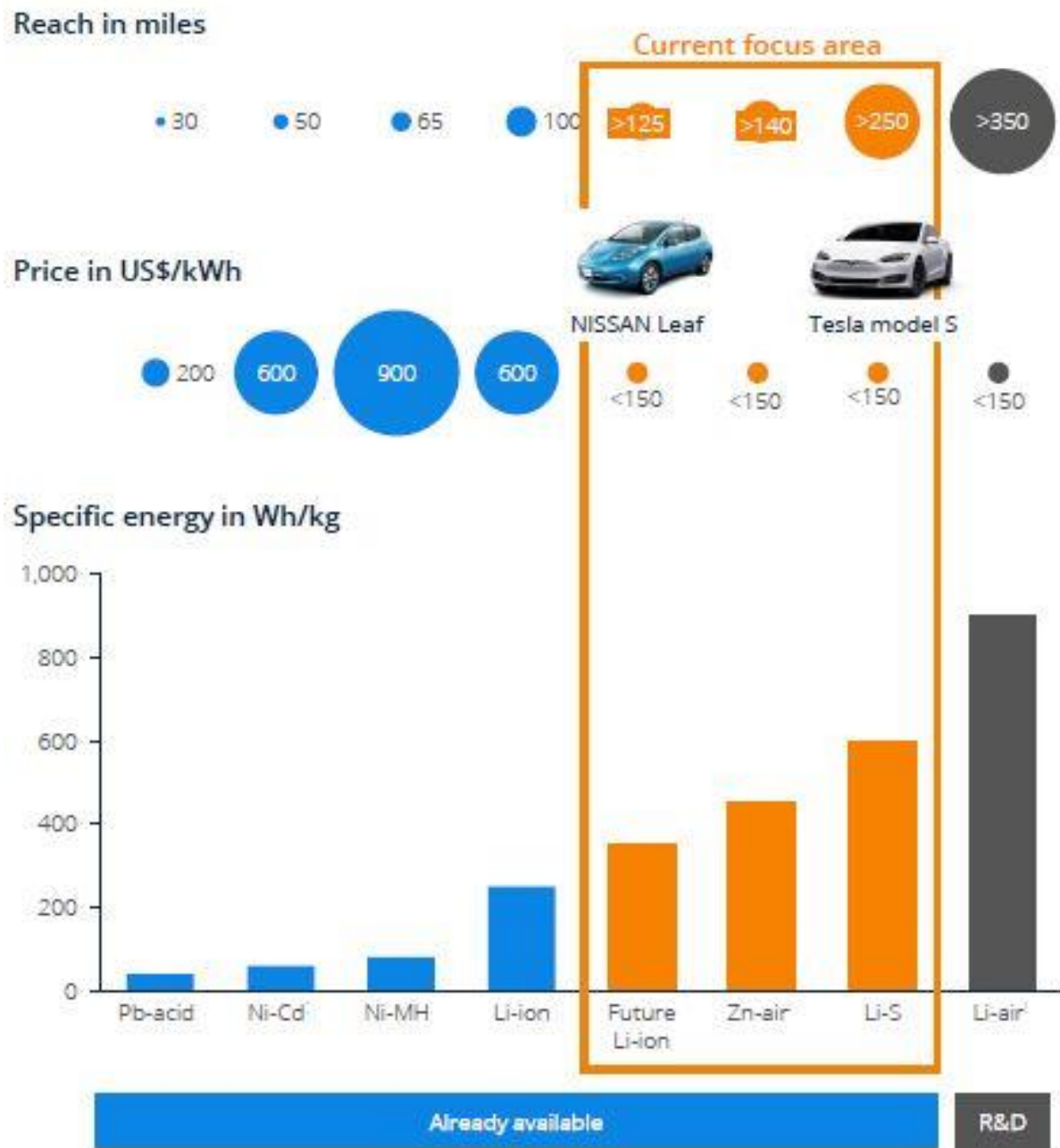
Figure 6 - Comparison between battery technologies in terms of mileage, price and specific energy (Statista, 2017)
