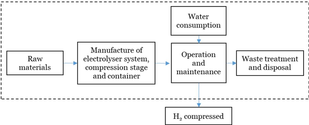
Figure 4-8: LCA boundaries assumed for the electrolyser system.
