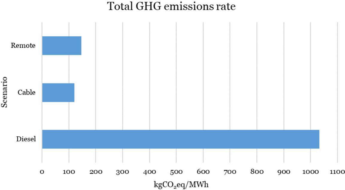
Figure 5-1: Comparison of the total GHG emissions rates of the three scenarios (Remote, Cable, Diesel).
