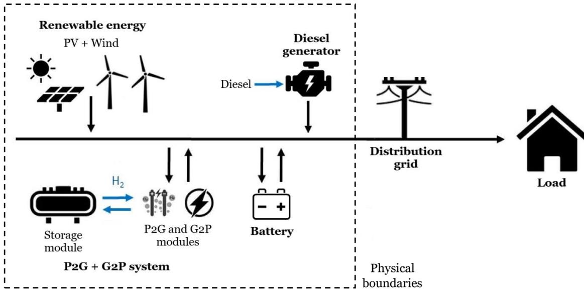
Figure 4-12: LCA physical system boundaries of the Remote scenario [21].
