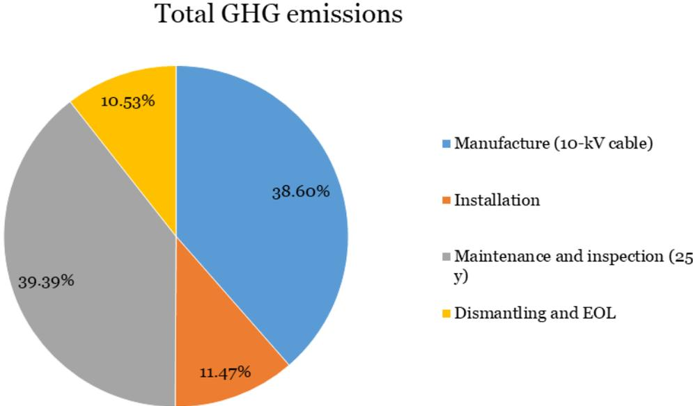
Figure 4-18: Relative contributions to the total GHG emissions of the submarine cable system.
