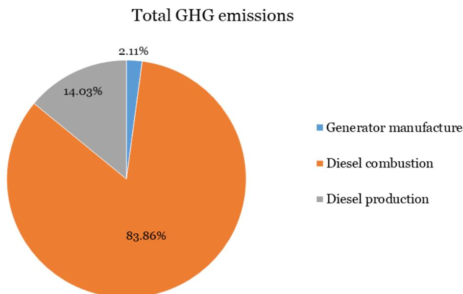
Figure 4-11: Relative contributions to the total GHG emissions of the diesel generator system (Remote scenario).
