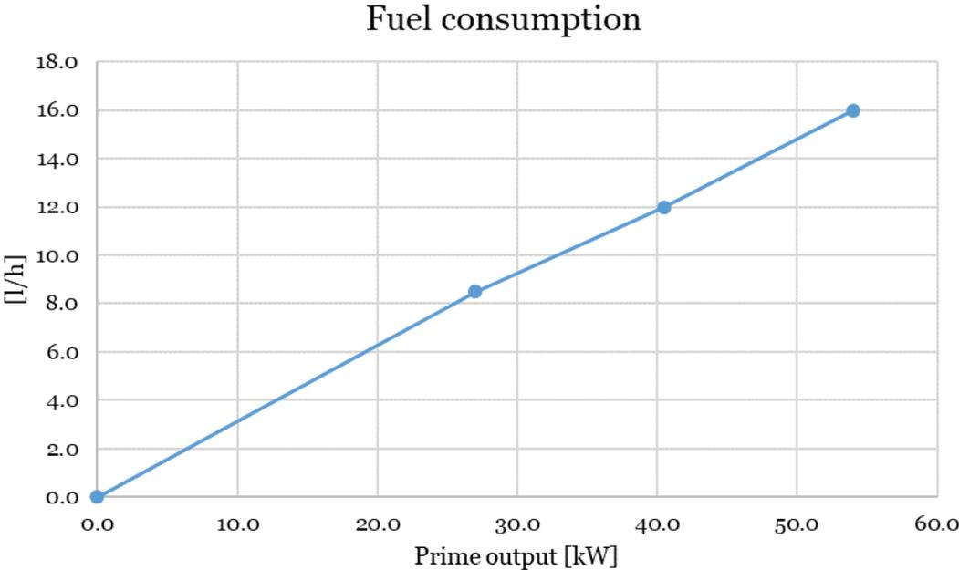
Figure 4-22: Fuel consumption of the diesel generator in function of the prime output.
