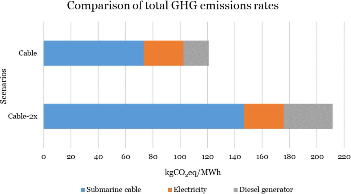
Figure 6-4: Comparison of the total GHG emissions rates of the Cable and Cable-2x scenarios.
