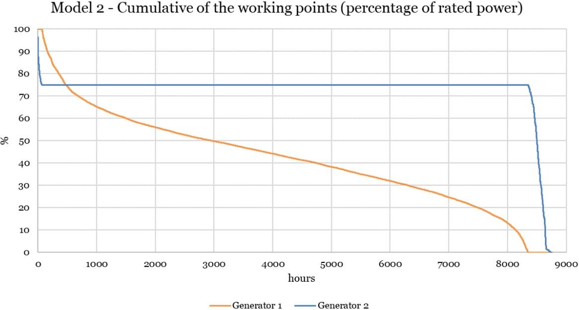
Figure 4-25: Cumulative curve of the generators working points (load model 2).
