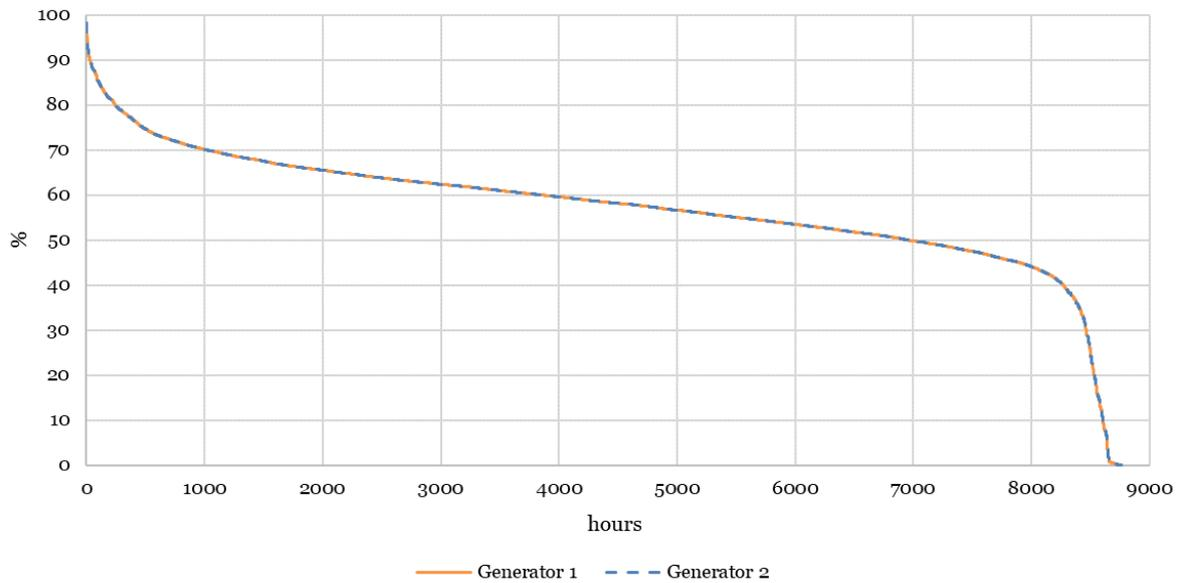
Figure 4-27: Cumulative curve of the generators working points (load model 4).
