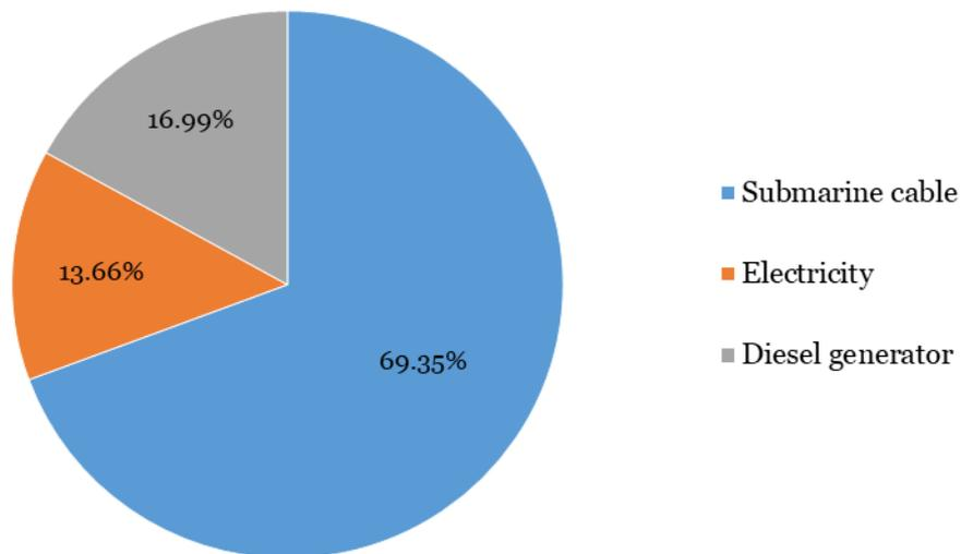
Figure 6-3: Relative contributions of each subsystem to the total GHG emissions of the Cable-2x scenario.
