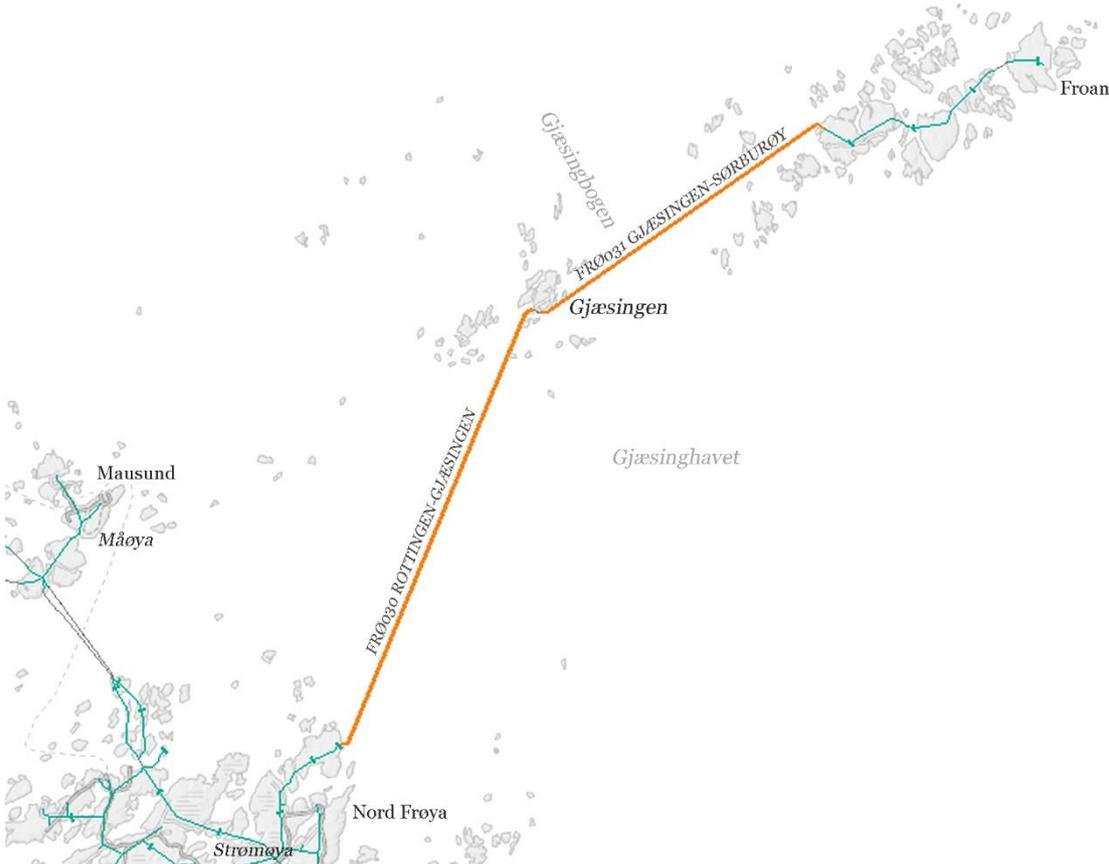
Figure 4-15: Sea cables electrically connecting the Froan Islands to the mainland [VI].
