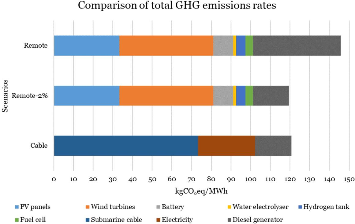
Figure 6-2: Comparison of the total GHG emissions rate (subdivided in each contribution) of the Remote-2% scenario with the Remote and Cable cases.
