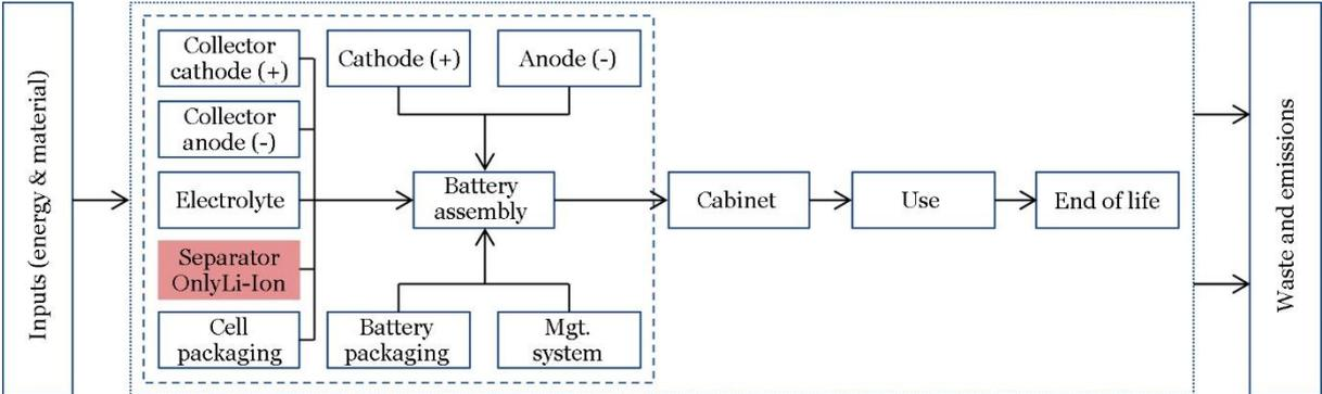
Figure 4-7: LCA boundaries of the battery system [74].
