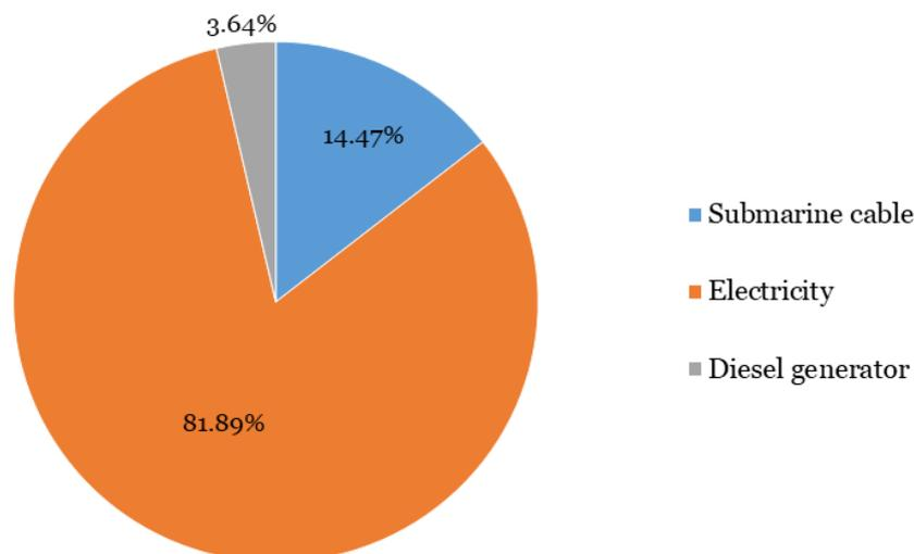
Figure 6-6: Relative contributions of each subsystem to the total GHG emissions of the Cable-Italy scenario.
