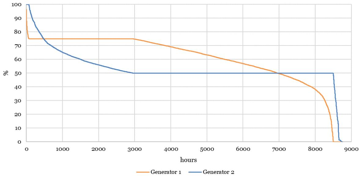
Figure 4-26: Cumulative curve of the generators working points (load model 3).
