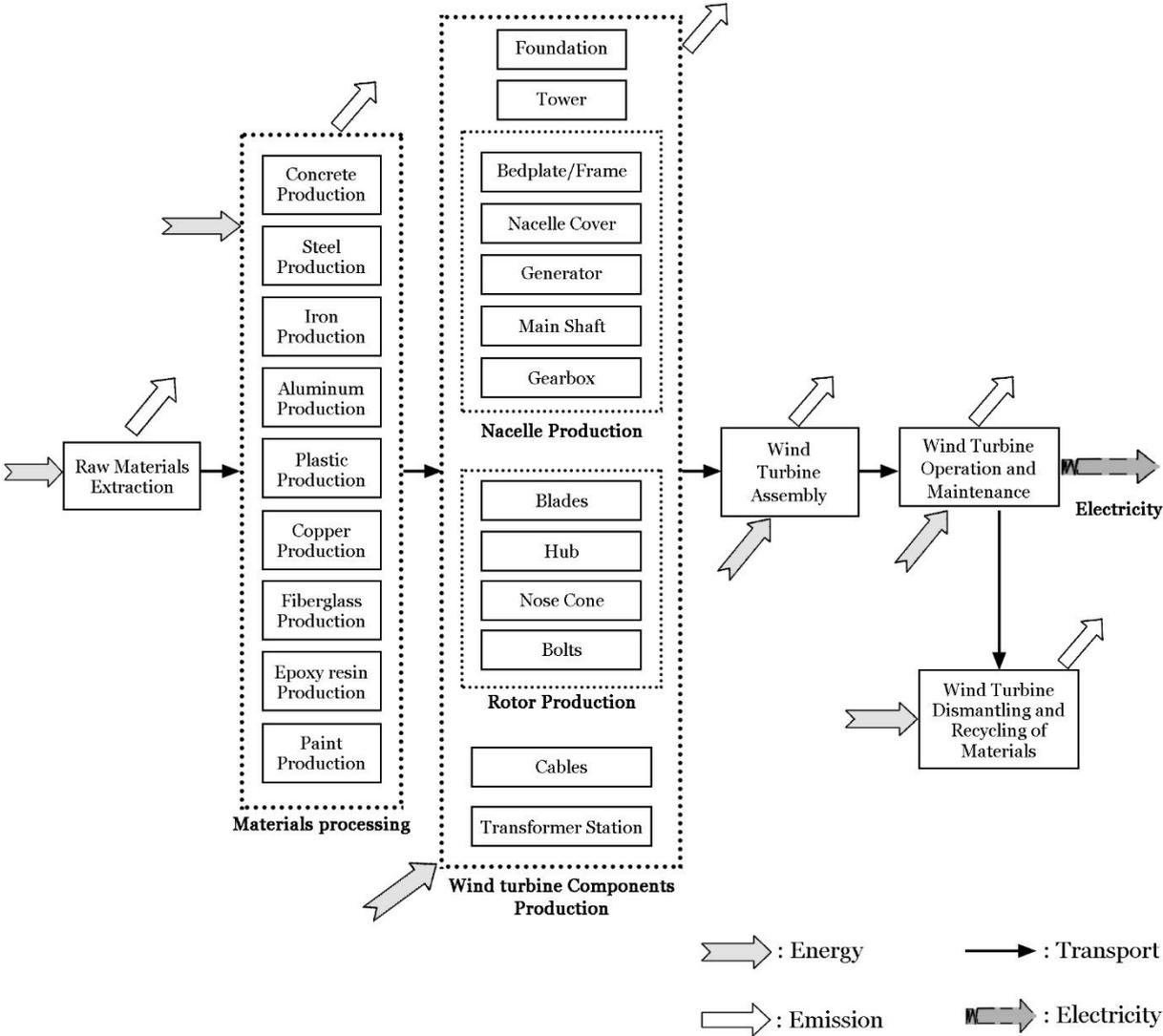
Figure 4-4: LCA boundaries of the WT system [80].
