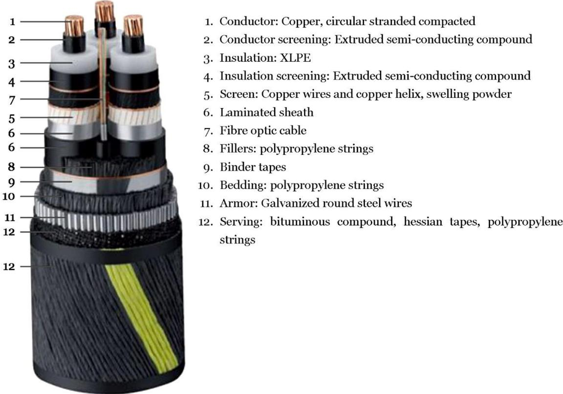
Figure 4-17: Construction layers of the XLPE three-core cable provided by Nexans [129].
