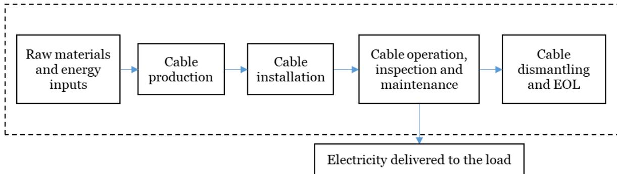
Figure 4-16: LCA boundaries assumed for the submarine cables system.
