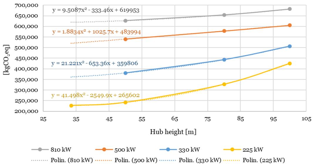
Figure 4-5: GHG emissions in function of hub heights and WT capacities, calculated from [80].
