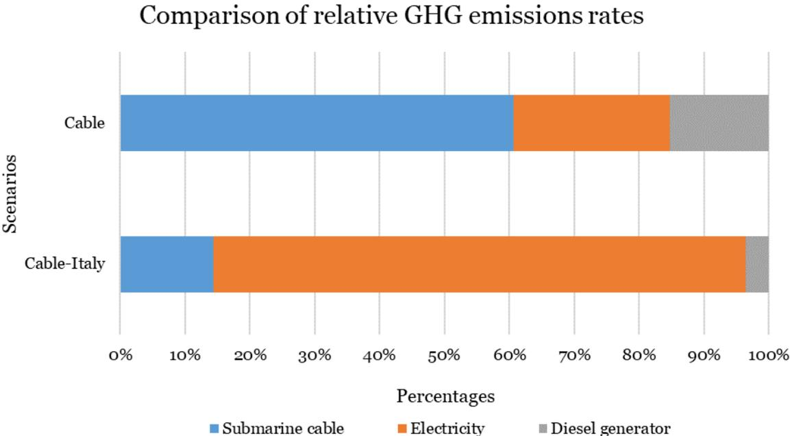
Figure 6-7: Comparison of the relative impacts to the total GHG emissions rate of the Cable and Cable-Italy scenarios.
