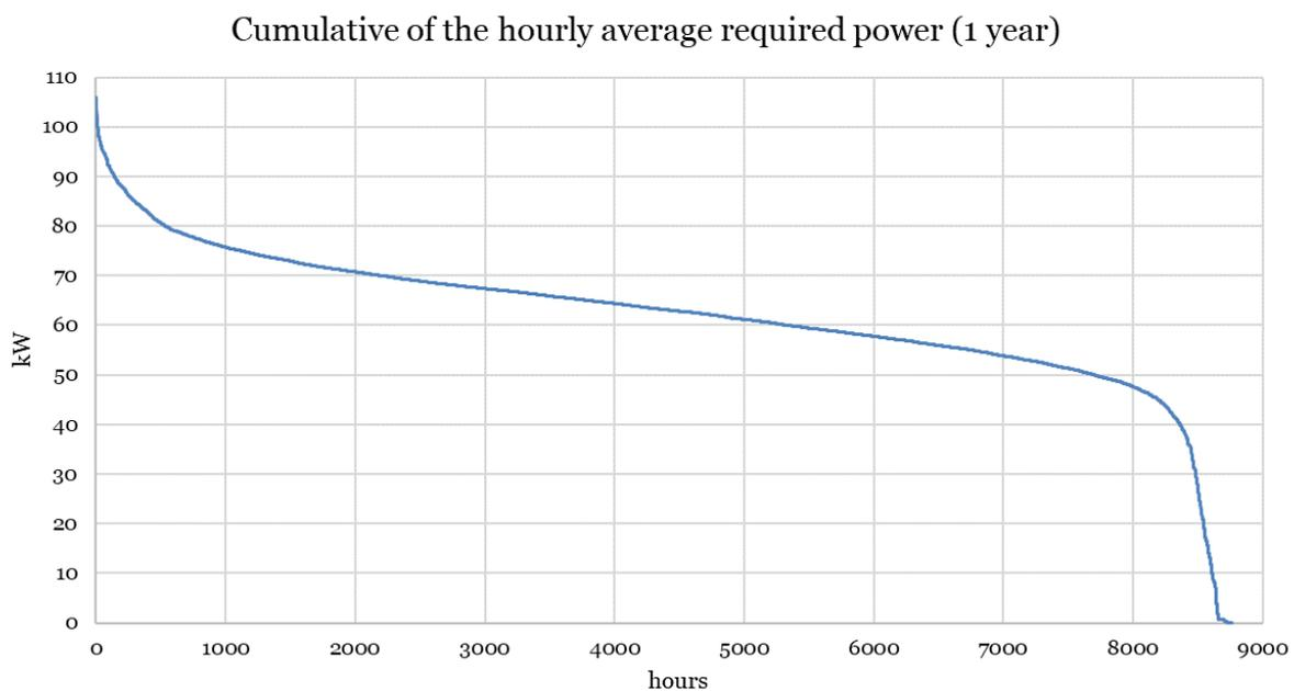
Figure 4-23: Cumulative curve of the hourly average power required by the Froan load (1-year simulation).
