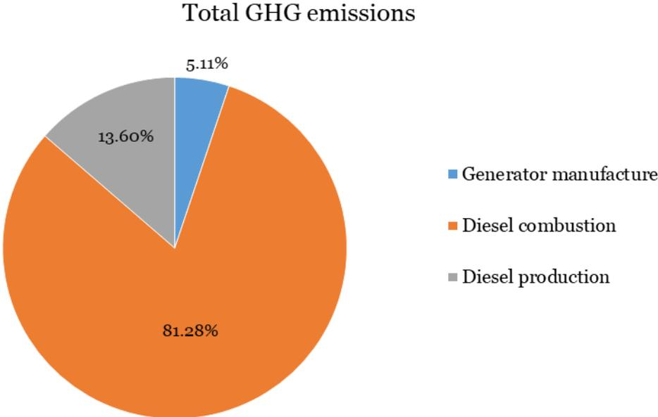
Figure 4-19: Relative contributions to the total GHG emissions of the diesel generator system (Cable case).
