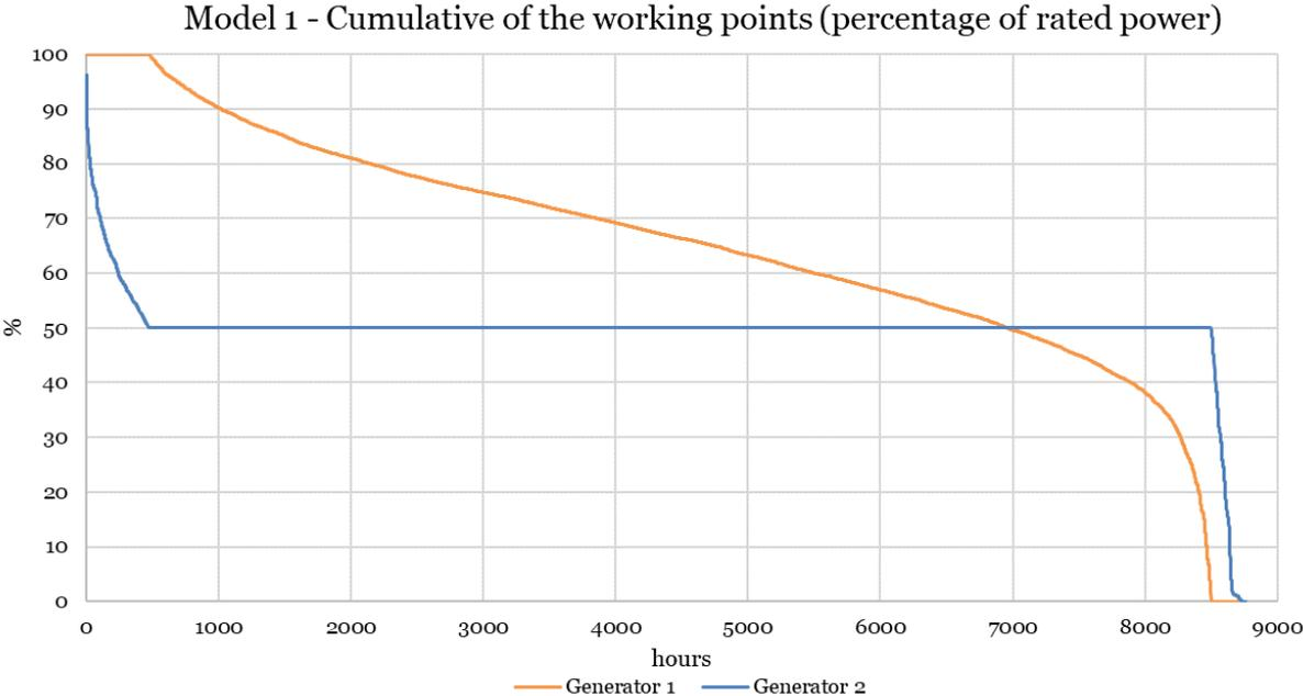
Figure 4-24: Cumulative curve of the generators working points (load model 1).
