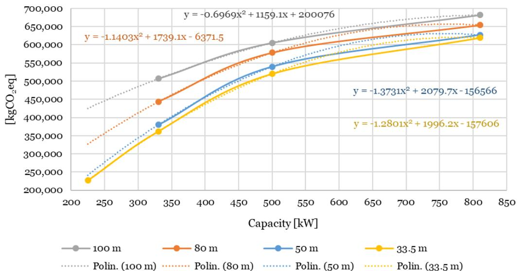
Figure 4-6: GHG emissions in function of WT capacities and hub heights, calculated from [80].
