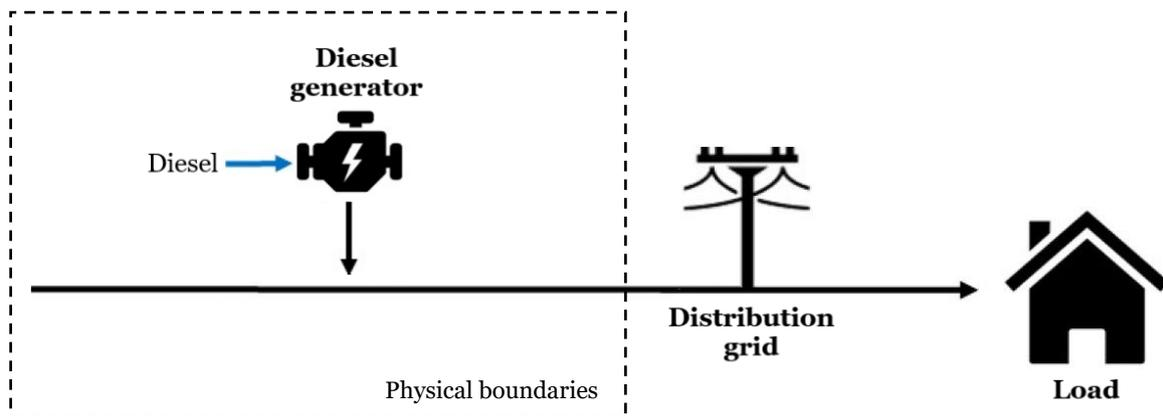
Figure 4-21: LCA physical system boundaries of the Diesel scenario [21].
