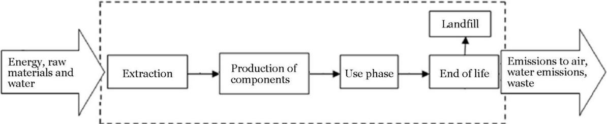
Figure 4-3: LCA boundaries of the PV system [82].
