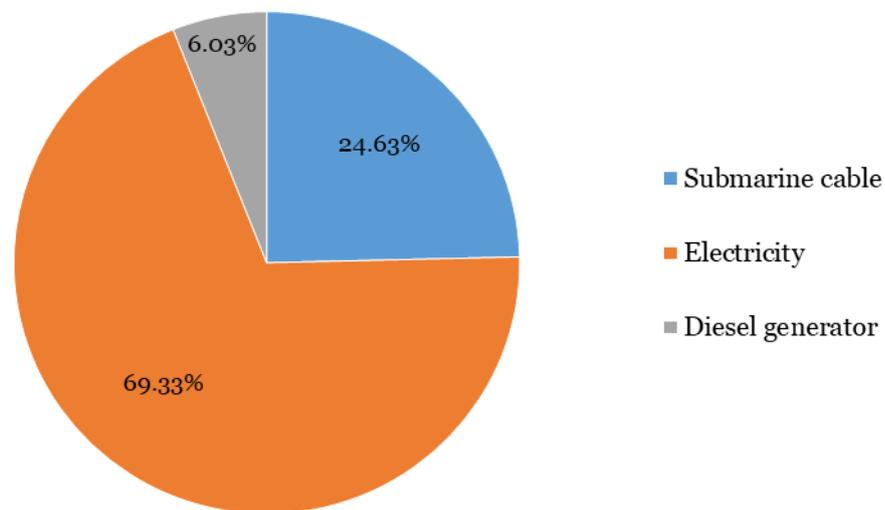
Figure 6-8: Relative contributions of each subsystem to the total GHG emissions of the Cable-2x-Italy scenario.
