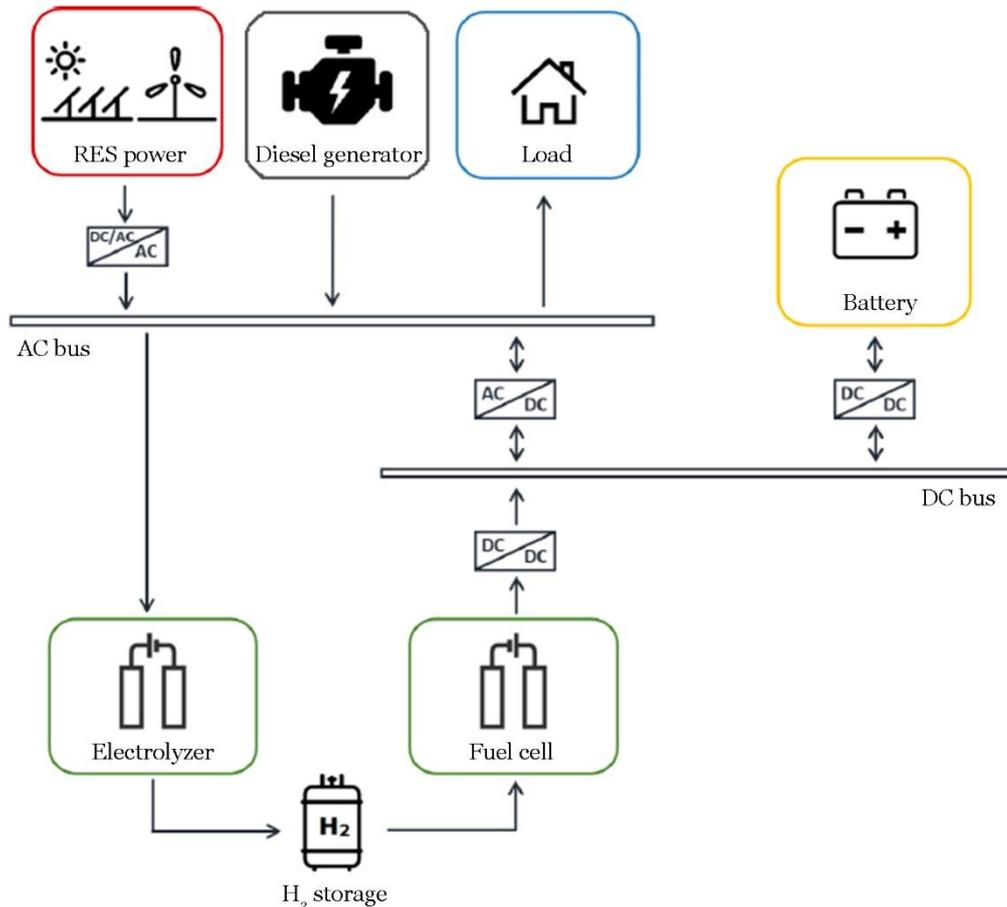
Figure 4-2: Scheme of the components and qualitative energy and mass exchanges in the Remote scenario [24].
