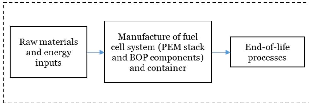
Figure 4-9: LCA boundaries assumed for the fuel cell system.
