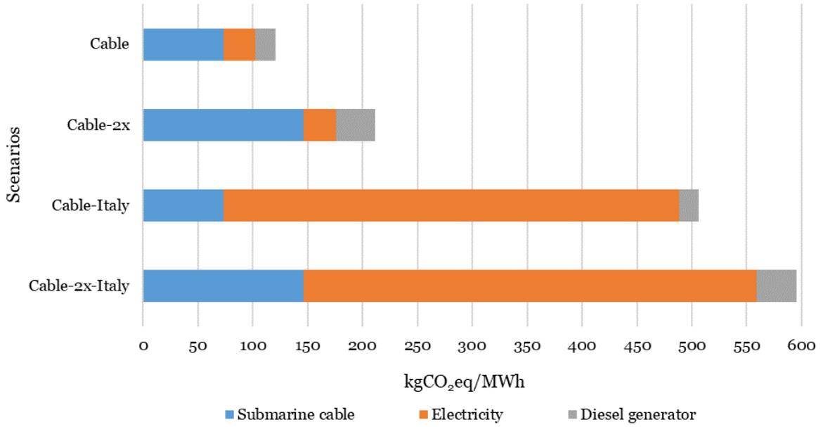
Figure 6-9: Comparison of the total GHG emissions rates of the Cable, Cable-2x, Cable-Italy and Cable-2x-Italy scenarios.
