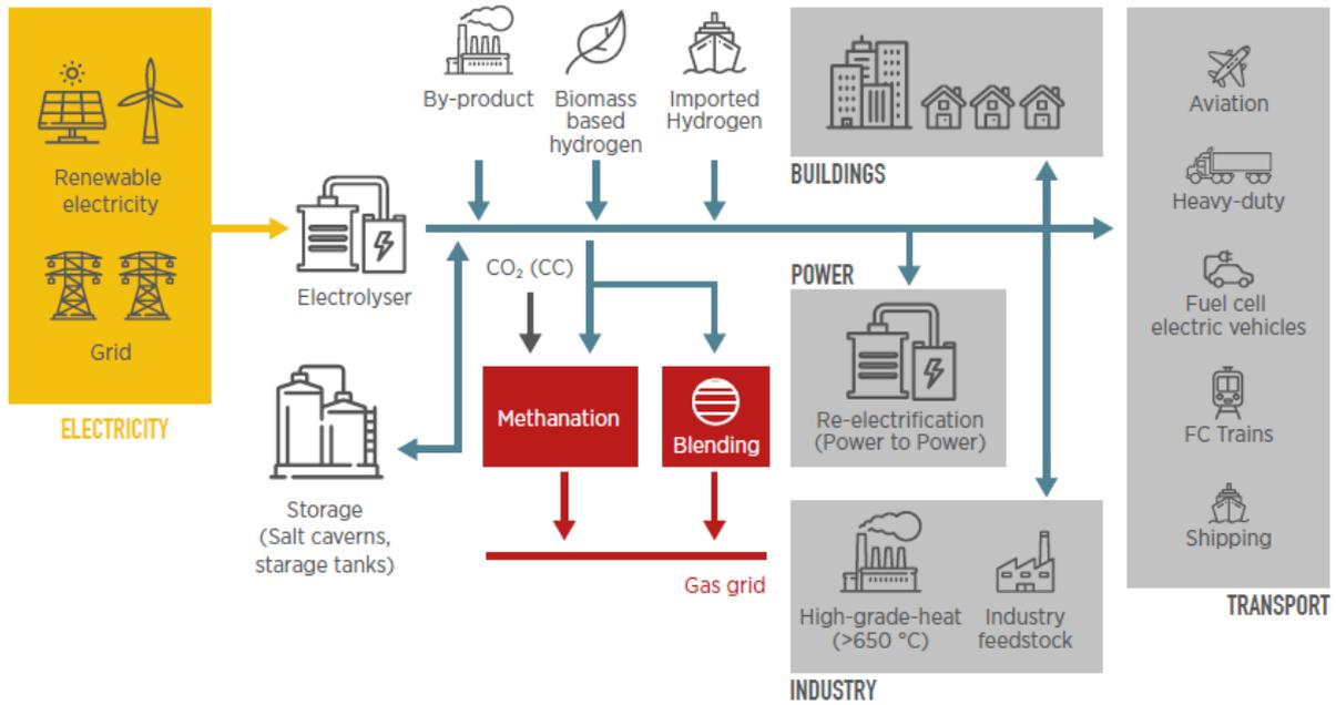
Figure 1-8: Integration of RES into end uses by means of hydrogen [17].
