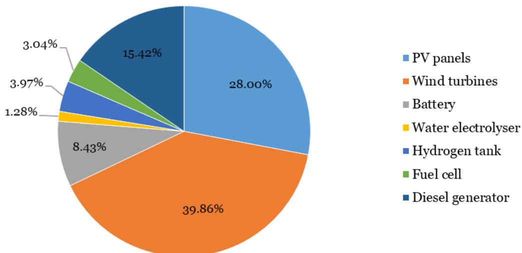
Figure 6-1: Relative contributions of each subsystem to the total GHG emissions of the Remote-2% scenario.
