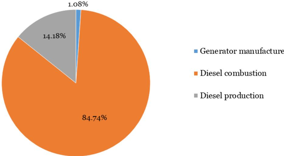
Figure 4-30: Relative contributions to the total GHG emissions of the diesel generator system (Diesel scenario).
