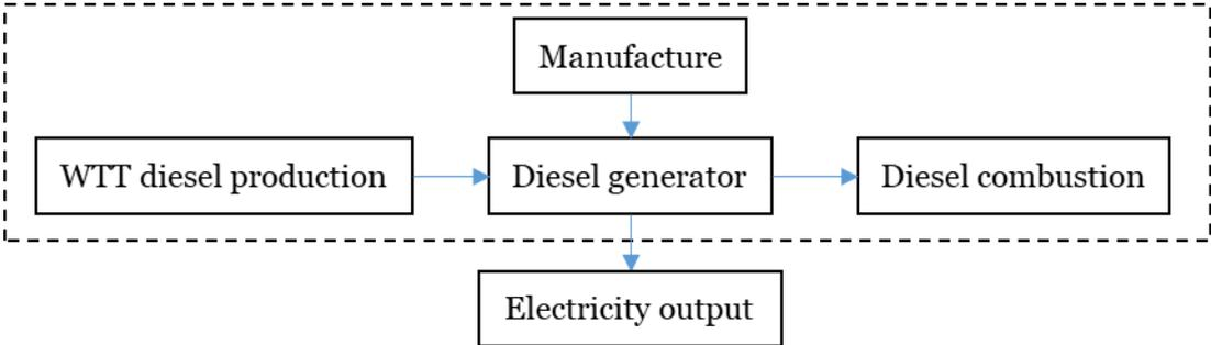
Figure 4-10: LCA boundaries assumed for the diesel generator system.
