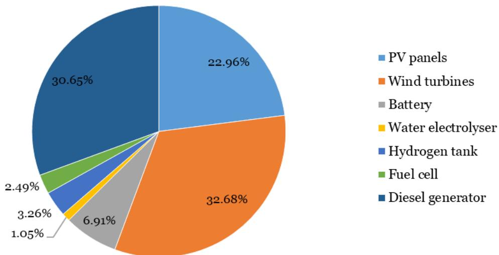
Figure 4-13: Relative contributions of each subsystem to the total GHG emissions of the Remote scenario.
