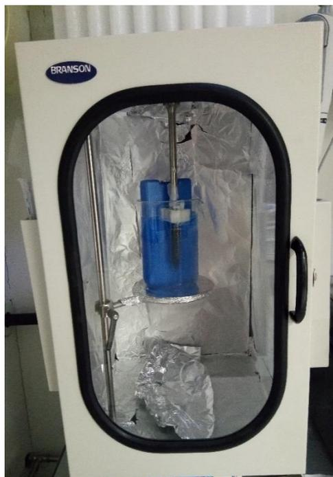
*Fig. 2.8– The dark blue polymeric solution (Clevios) inside the sonifier. The beaker contains water and ice (the blue element behind the solution), to refrigerate the system, due to the high temperature caused by cavitation.*
