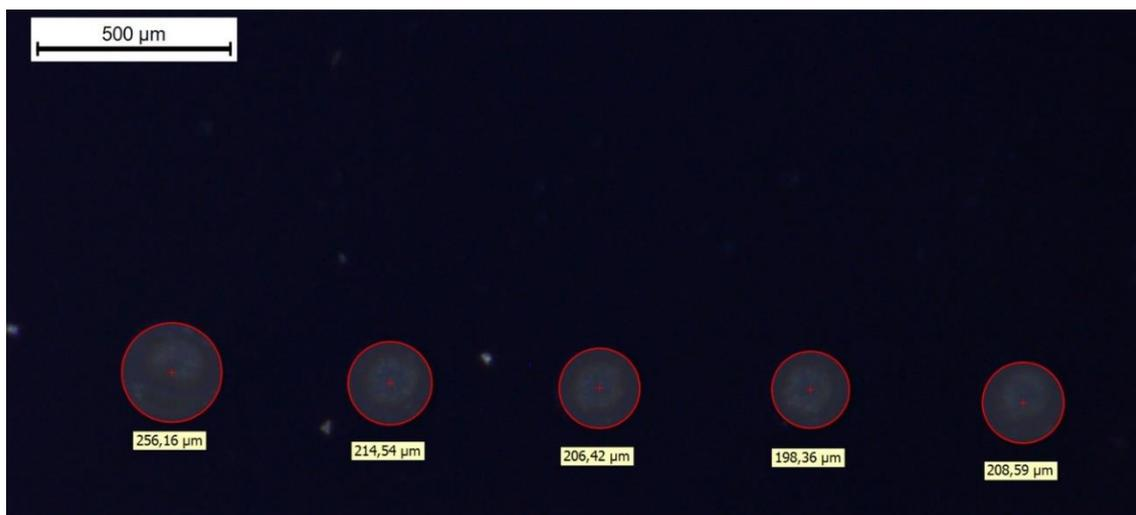
Fig. 3.10 – Droplets of *Clevios* on a silicon oxide substrate, generated by the same bipolar wave used for DI water.
