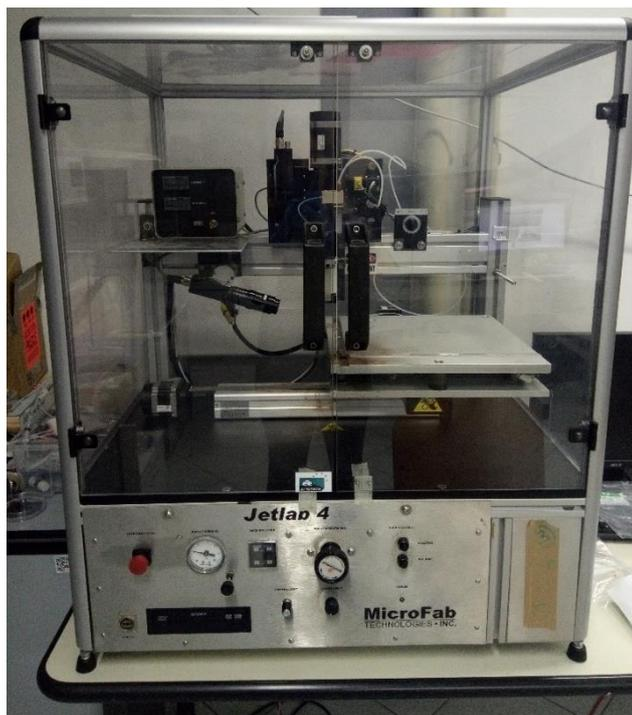
Fig. 2.14 – Microfab Jetlab 4 DOD ink-jet printer
