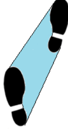
Figure 1.4: Schematic representation of a BoS in a double support phase. The area comprises both feet (black) and the area between them (light blue).
