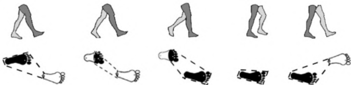
Figure 1.3: The base of support throughout the gait cycle, respectively at heel strike, foot flat, toe off and heel strike instants. The dark regions of the feet and the dashed lines represent the feet portions of contact and the perimeter of the base of support, [7].
