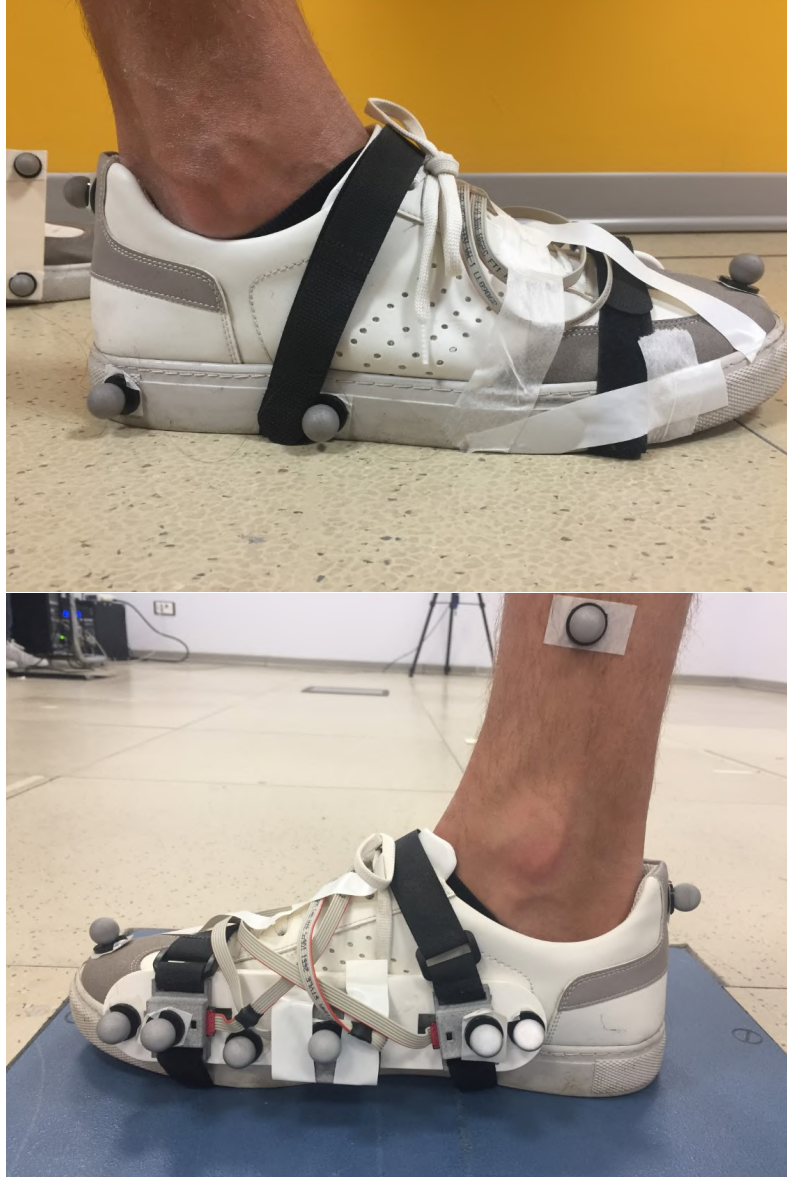
Figure 15.4: Right foot of the subject during the experimental session aiming at estimating the spatial gait parameters with the SP reference.
