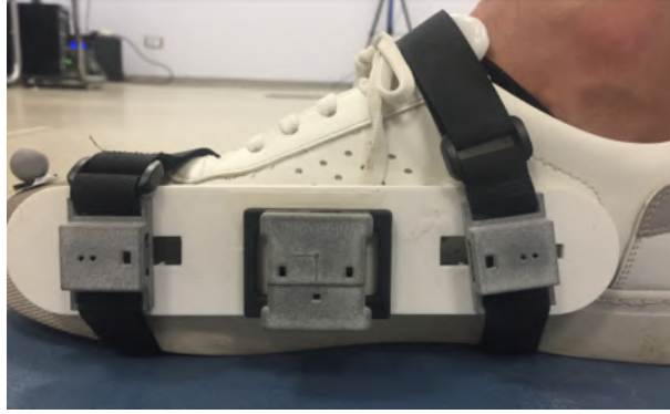
Figure 15.2: Set up of the MIMU and the two DSs attached on the same planar support.
