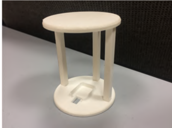
Figure 15.7: Object modelled for the estimation of the offset of the IR ToF sensors. The actual distance that they would measure is 0.05 m.
