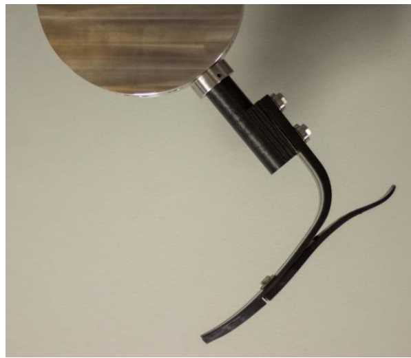
Figure 3.1.3 – Crescent-shaped support with the Vari-Flex® screwed on it. [51]
