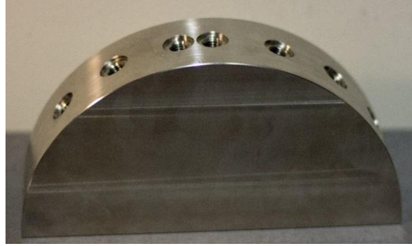
Figure 3.1.2 – Details of the crescent-shaped special support designed by L.Cavallaro et al. [51]
