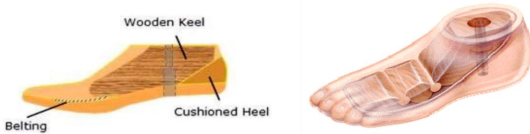
Figure 1.5.1 – Examples of rigid feet. On the left there is an example of SACH foot. On the right is represented a dynamic foot. [27]
