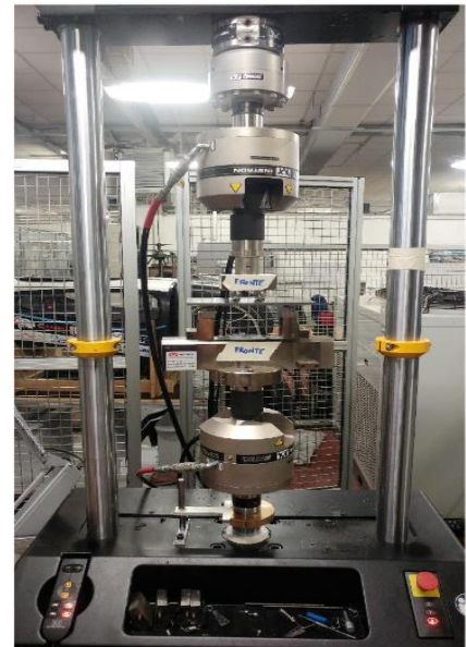
Figure 3.1.1 – Fatigue testing machine Instron 8801. [51]
