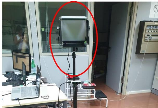
Figure 5.22: Experimental setup with one additional LED lamp: the LED lamp is behind the Intel RealSense D435
