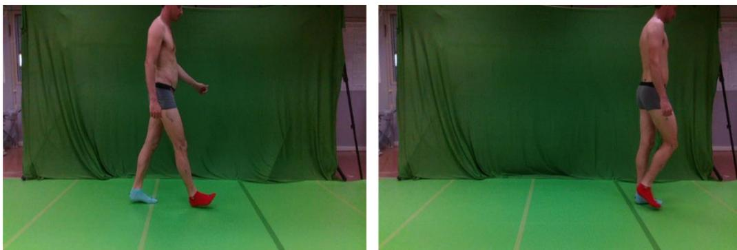
Figure 4.23: Variation of the two-dimensional images caused by the parallax effects due to the relative distance between the RGB-D camera and the participant. In particular, when the subject is close to the extremities of the FOV of the camera (b) there is a variation of shape and size of the body segments. This variation is absent when the subject is in the center of the FOV of the camera.
