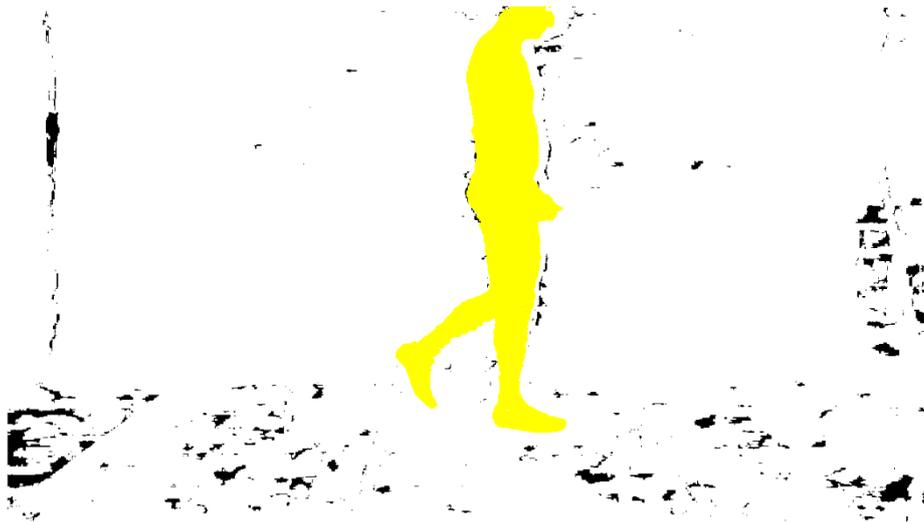
Figure 4.31: Segmented image (yellow surface) is overlapped on the depth image in order to selected only the subject
