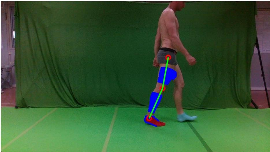
Figure 4.43: Extracted foreground thigh in situation 2. The blue surfaces represent the shank and the thigh, the blue line represents the foot, the green lines represent the LM-LE segment and the LE-GT segment. The first empty red dot is the LM the second empty red dot is the LE, and the higher empty red dot is the GT.
