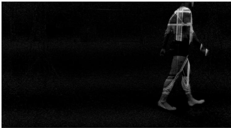
Figure 6.3: The difference image  $D$  obtained without the green background. The background is not homogeneous and for this reason, the difference image  $D$  is affected by the portion of the background which lies behind the subject.
