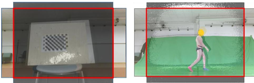
Figure 5.6: Identification of a common ROI in both RGB and depth images.
