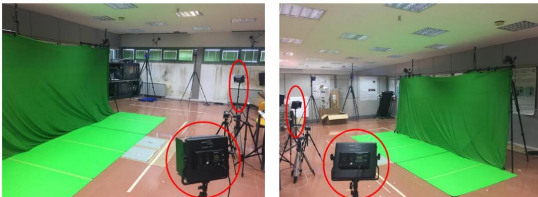
Figure 5.21: Experimental setup with two additional LED lamps: the LED lamps are on the left and right of the Intel RealSense D435.
