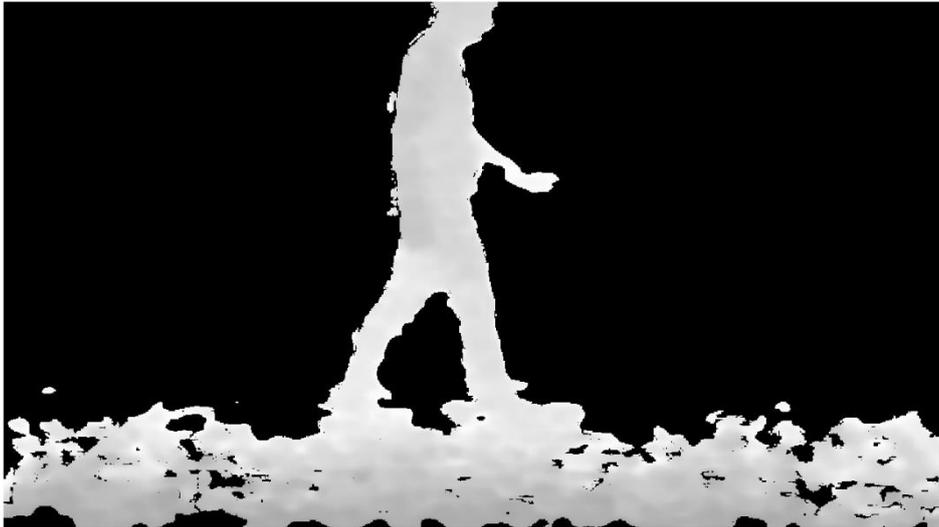
Figure 4.7: Depth image obtained after the removal of the depth values outside the depth values range.
