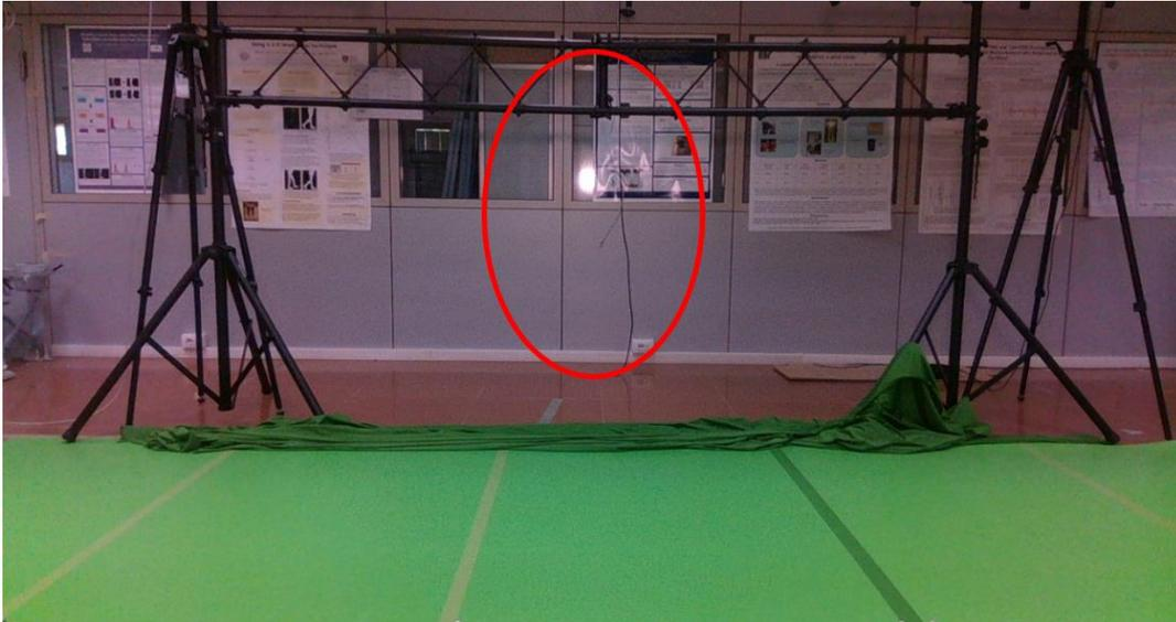
Figure 6.5: This image presents the experimental setup without the green background and with one additional LED lamp. It is possible to notice the light reflections on the background which increase the homogeneity of the background.
