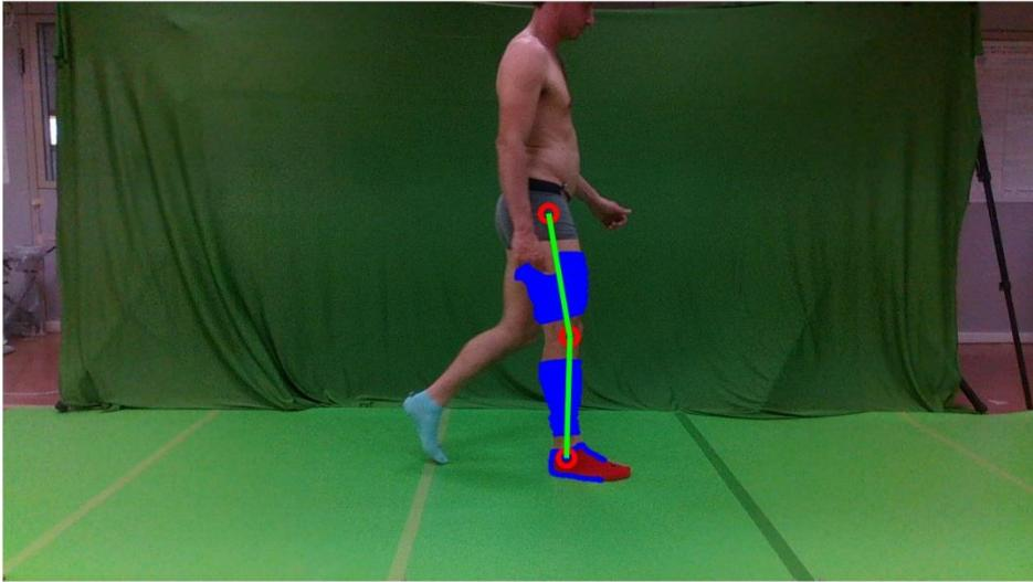
Figure 4.44: Extracted foreground thigh in situation 1. The blue surfaces represent the shank and the thigh, the blue line represents the foot, the green lines represent the LM-LE segment and the LE-GT segment. The first empty red dot is the LM the second empty red dot is the LE, and the higher empty red dot is the GT.
