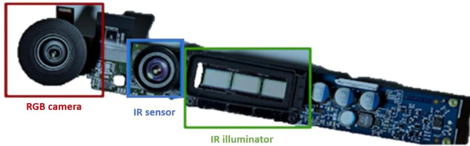
Figure 5.2: Sensors belonging Kinect 2 camera: RGB camera, IR sensor and IR illuminator
