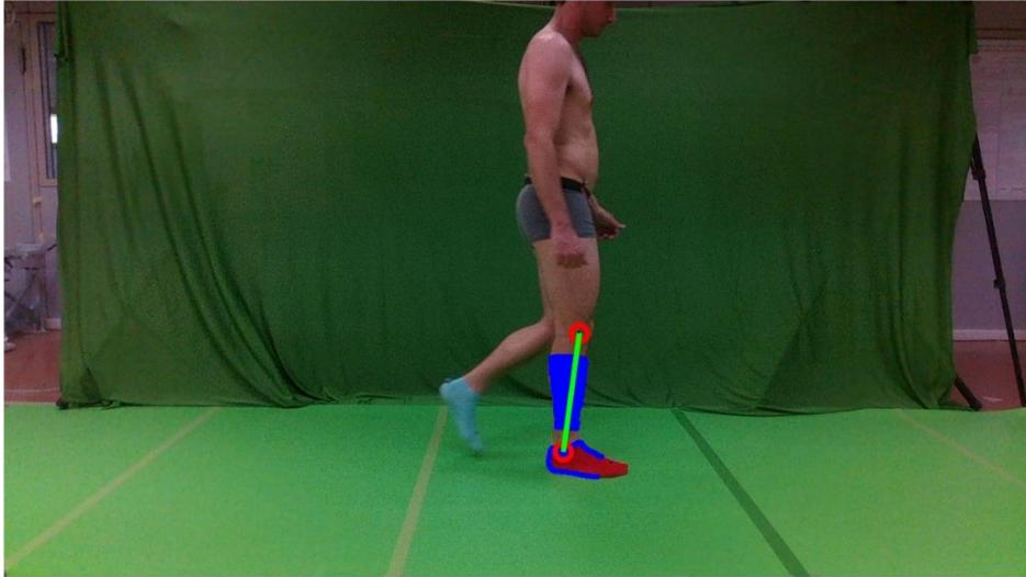
Figure 4.37: Extracted foreground shank. The blue surface represents the shank, the blue line represents the foot, the green line represents the LM-LE segment. The lowest empty red dot is the LM and the highest empty red dot is the LE.
