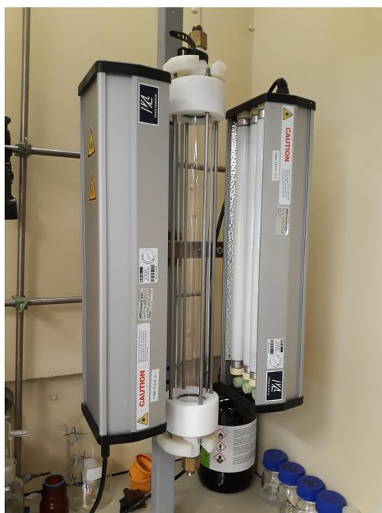
**Figure 2.4:** Quartz tube photoreactor.
