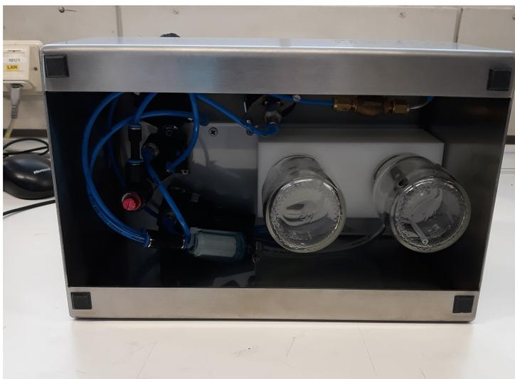
**Figure 2.3:** Bottom of the aerosol generator by PALAS.
