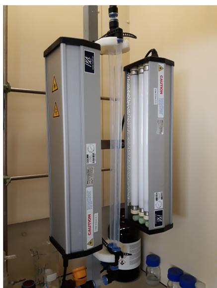
(a) 2-tubes photoreactor.
