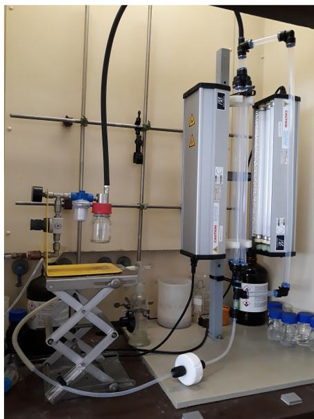
**Figure 1.2:** The whole employed setup: on the left the pneumatic atomizer connected to the 4-FEP tube photoreactor (on the right).
