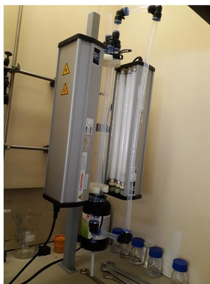
(b) 4-tubes photoreactor.
