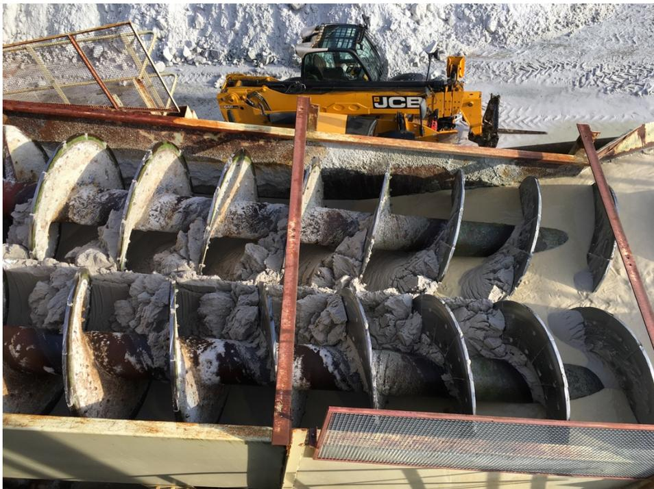
Figure I.4 Double Screw classifier
