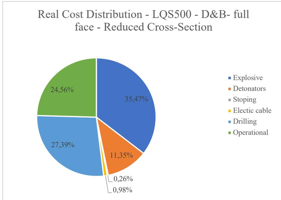
Figure 5.4 Percentage Distribution of the Costs - D&B - full face analysis, reduced cross-section
