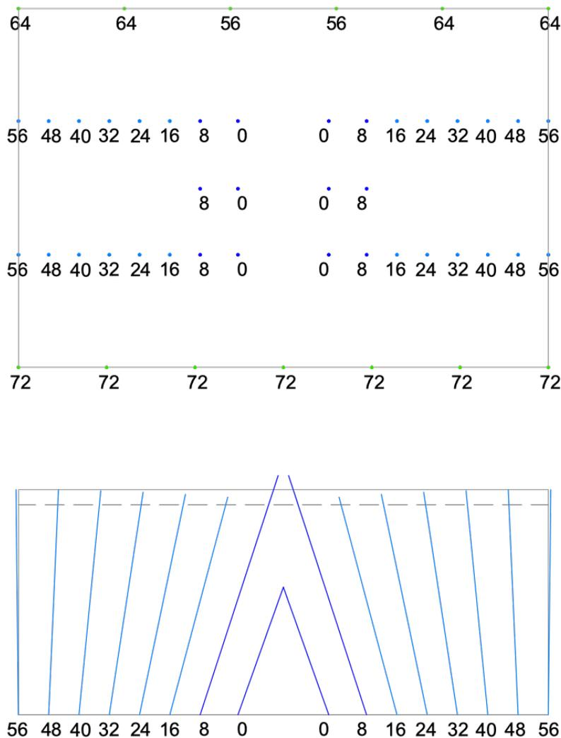
Figure IV.2 Blasting scheme for the production of LQS85
