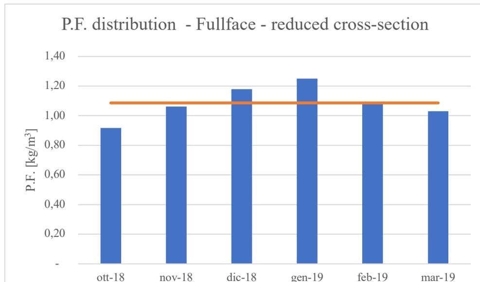
Figure IV.11 Distribution of the P.F.- D&B - full face - reduced cross-section
