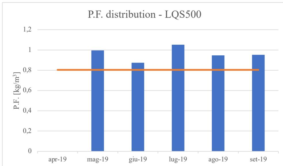
Figure IV.12 Distribution of the P.F.- D&B - full face - Usual cross-section
