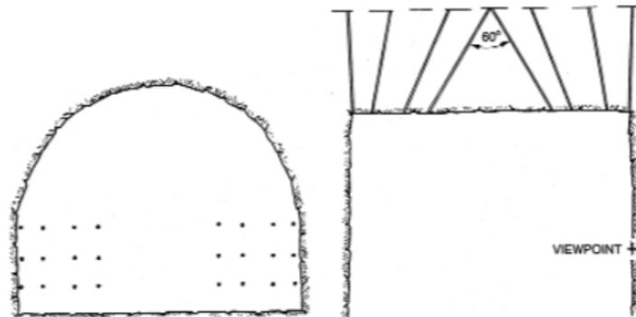
Figure IV.1 V-cut theoretical scheme
