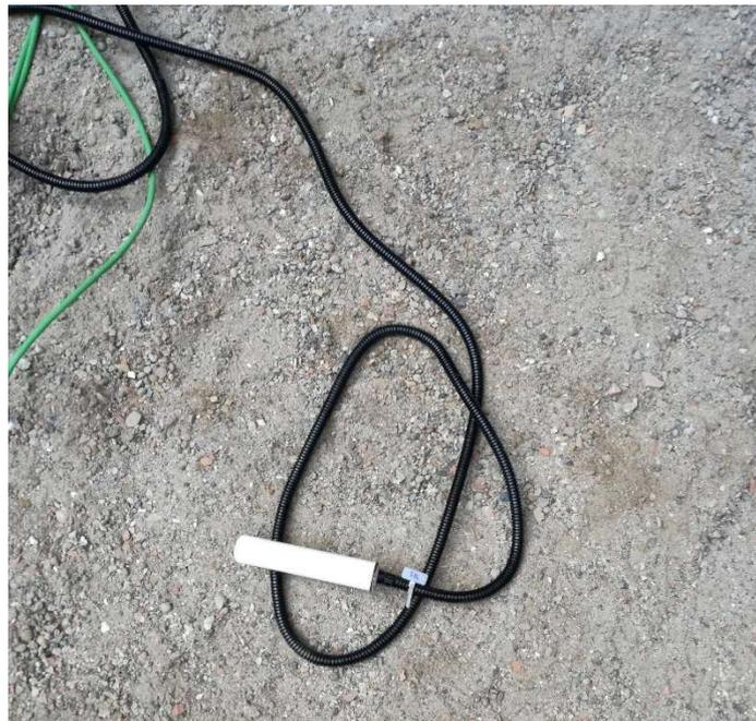
*Figura 46 – Sensore Sentek drill & drop probe*
