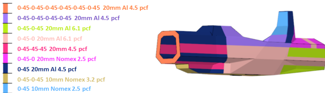
Figure 63. Final SC19 laminates configuration.
