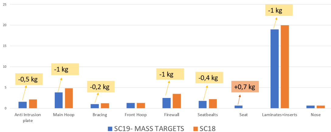
Graphic 5. Summary of weight saving prevision for the SC19 monocoque.
