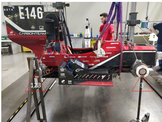
Graphic 6. Torsional stiffness test.
