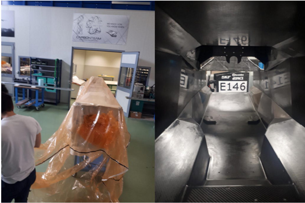
Figure 71. Left: vacuum bag preparation. Right: coupled cured molds.
