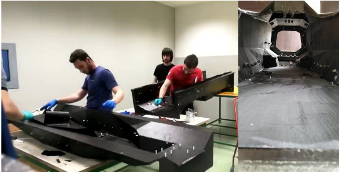
Figure 72. Left: lay up on the first layers on the two halves; note the presence of pins used for the positioning of the inserts. Right: outer skin cured with inserts.
