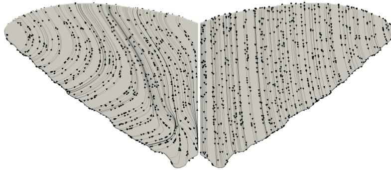
Figure 3.32.: Limiting streamlines (shear stress field) on the wing using the PANS turbulence model. On the left the dorsal (suction) side, on the right the ventral (pressure) side.
