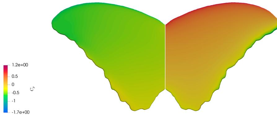
Figure B.38.: *Morpho deidamia*: pressure coefficient on the wing at  $16^\circ$  angle of attack. On the left the dorsal side, on the right the ventral side of the wing.
