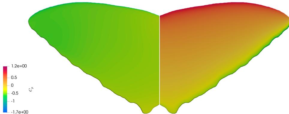
Figure B.30.: *Morpho cisseis*: pressure coefficient on the wing at  $20^\circ$  angle of attack.
