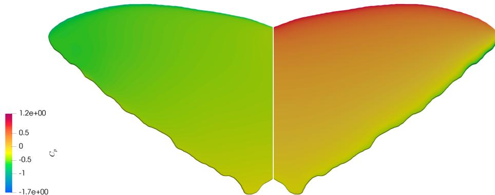
Figure B.28.: *Morpho cisseis*: pressure coefficient on the wing at  $16^\circ$  angle of attack.
