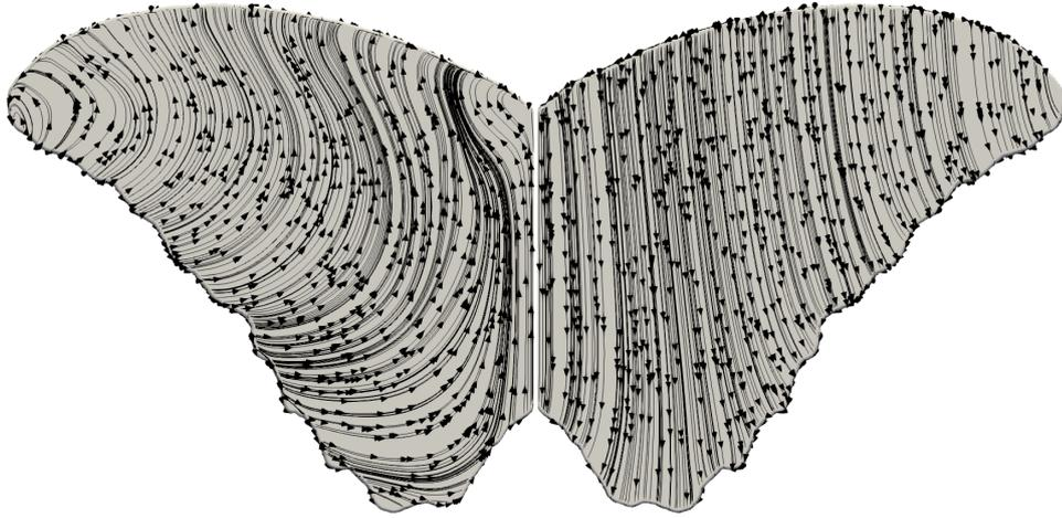
Figure B.56.: *Morpho deidamia*: velocity limiting streamlines on the wing at  $12^\circ$  angle of attack. On the left the dorsal side, on the right the ventral side of the wing.
