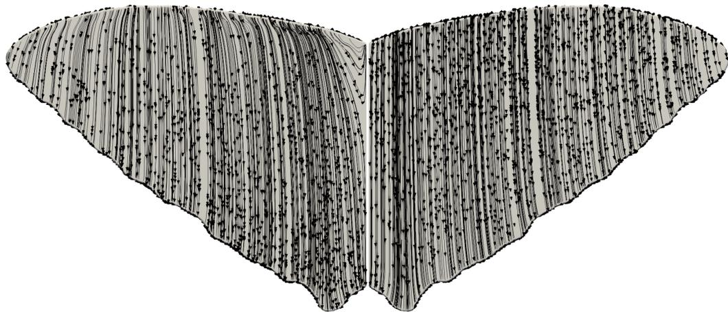
Figure B.42.: *Morpho cisseis*: velocity limiting streamlines on the wing at  $4^\circ$  angle of attack. On the left the dorsal side, on the right the ventral side of the wing.
