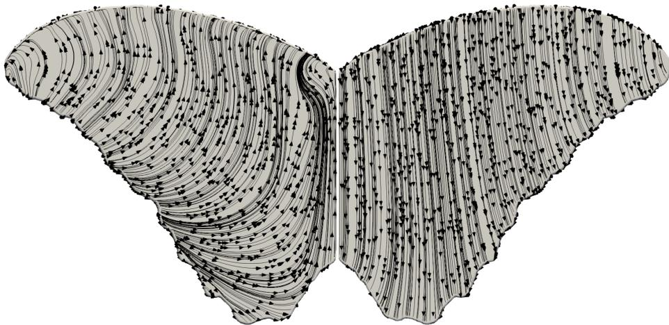
Figure B.55.: *Morpho deidamia*: velocity limiting streamlines on the wing at  $10^\circ$  angle of attack. On the left the dorsal side, on the right the ventral side of the wing.
