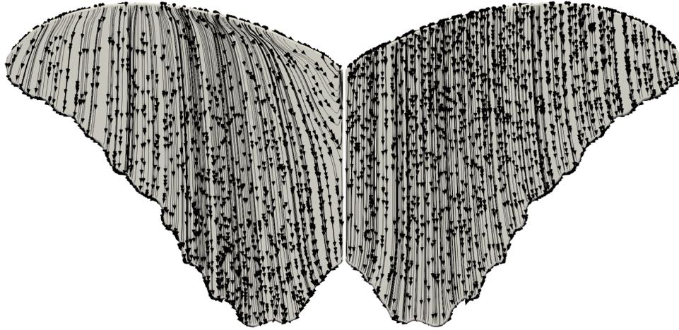
Figure B.52.: *Morpho deidamia*: velocity limiting streamlines on the wing at  $4^\circ$  angle of attack. On the left the dorsal side, on the right the ventral side of the wing.
