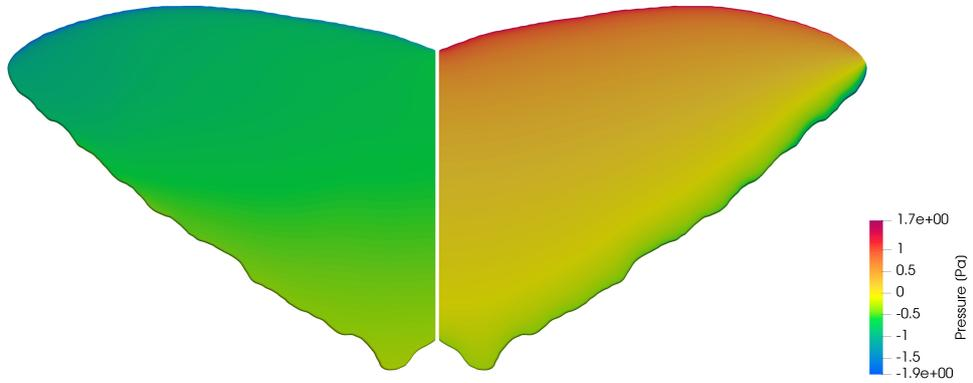
Figure 3.23.: Pressure field on the wing using the SST  $k - \omega$  model. On the left the dorsal (suction) side, on the right the ventral (pressure) side.
