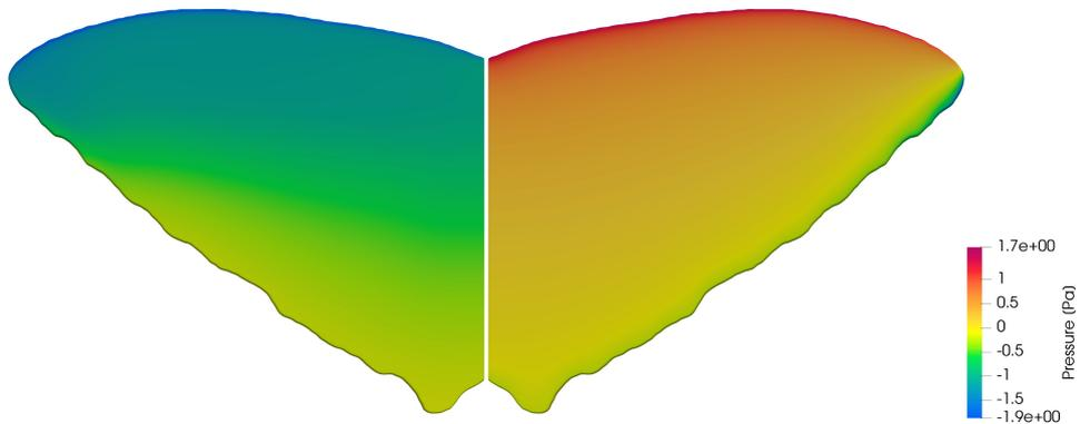
Figure 3.26.: Pressure field on the wing using the SST  $k - \omega$  turbulence model with  $\gamma - Re_\theta$  transition model;  $\nu_t/\nu=10$  inflow condition. On the left the dorsal (suction) side, on the right the ventral (pressure) side.
