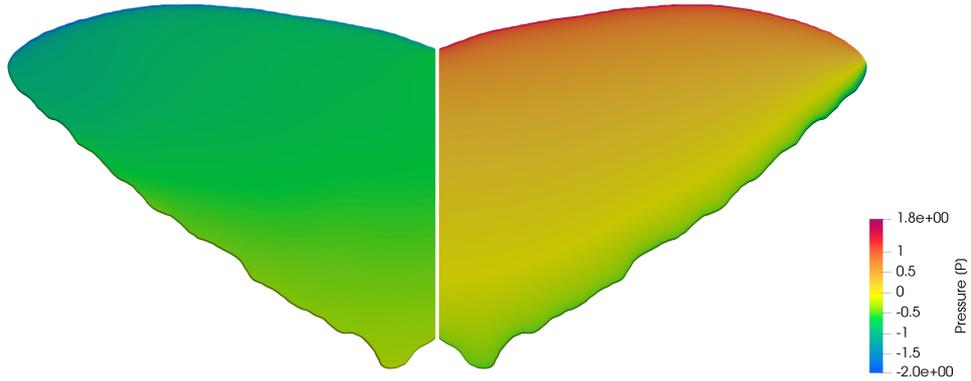
Figure 3.27.: Pressure field on the wing using the PANS turbulence model. On the left the dorsal (suction) side, on the right the ventral (pressure) side.
