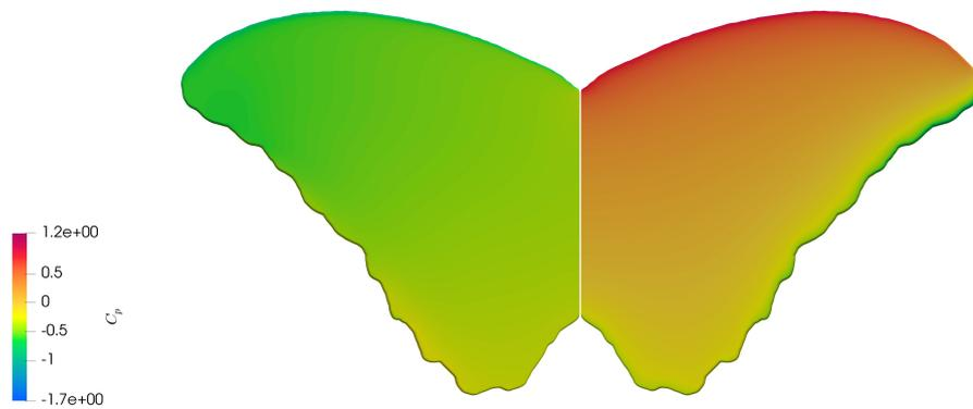
Figure B.39.: *Morpho deidamia*: pressure coefficient on the wing at  $18^\circ$  angle of attack. On the left the dorsal side, on the right the ventral side of the wing.
