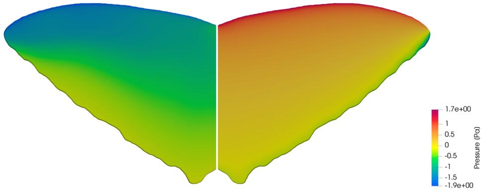
Figure 3.24.: Pressure field on the wing using the Spalart-Allmaras model. On the left the dorsal (suction) side, on the right the ventral (pressure) side.
