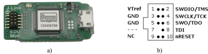
**Figure 3.25:** a) J-Link EDU Mini SEGGER®, b) Connection of the J-Link EDU Mini followed to implement the electronic interconnection to JTAG port [48].
