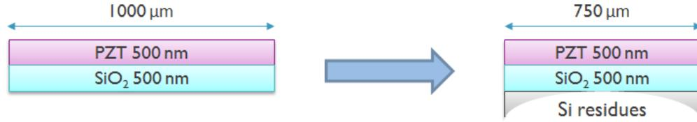
Figure 5.18: Graph with the desirable membrane (left) and with the obtained one after Bosch process (right). The radius membrane is reduced, and the bottom part is bended. The electrodes are removed for the sake of clarity.
