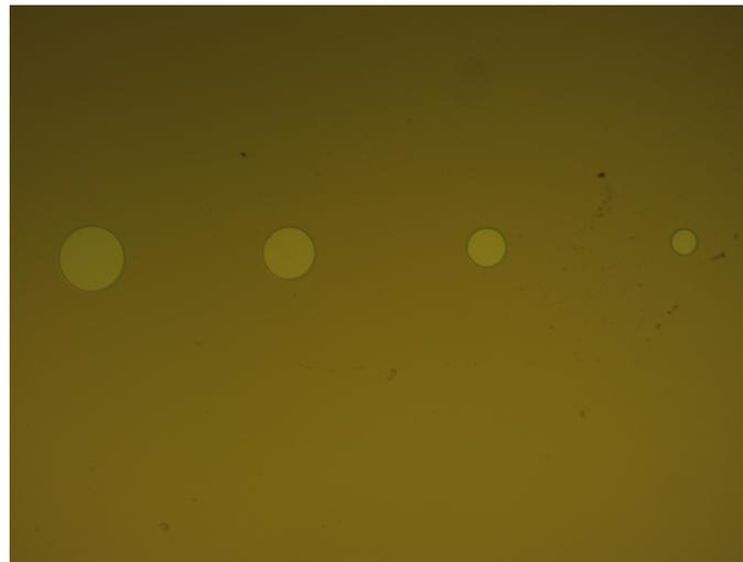
(b) Small features, 200  $\mu\text{m}$ , 160  $\mu\text{m}$ , 120  $\mu\text{m}$  and 80  $\mu\text{m}$  from left to right.
