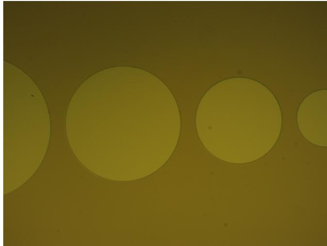
(a) Big features, 1000  $\mu\text{m}$ , 800  $\mu\text{m}$ , 600  $\mu\text{m}$  and 400  $\mu\text{m}$  from left to right.
