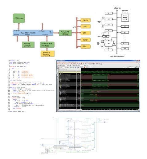
IPs microarchitecture, RTL design, UVM based standalone functional verification and synthesis have been carried out based on system specifications for enhancing the stability and security of the interconnect of new microprocessors. All the design is fully configurable to be easily integrated into other systems and synthesizable with the required timing constraints of the first targeted SoC.
