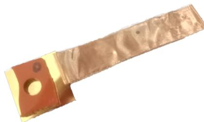
**Figure 1.8** – Gold sample with silicone gasket and copper tape.
