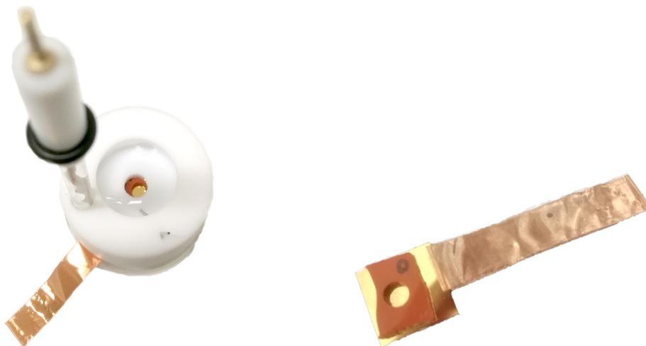
**Figure 1.7** – Electrochemical cell mounted with the gold working electrode (on the bot-
