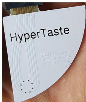
Figure 5.3. Sensor array based on Au/ENIG electrodes.
