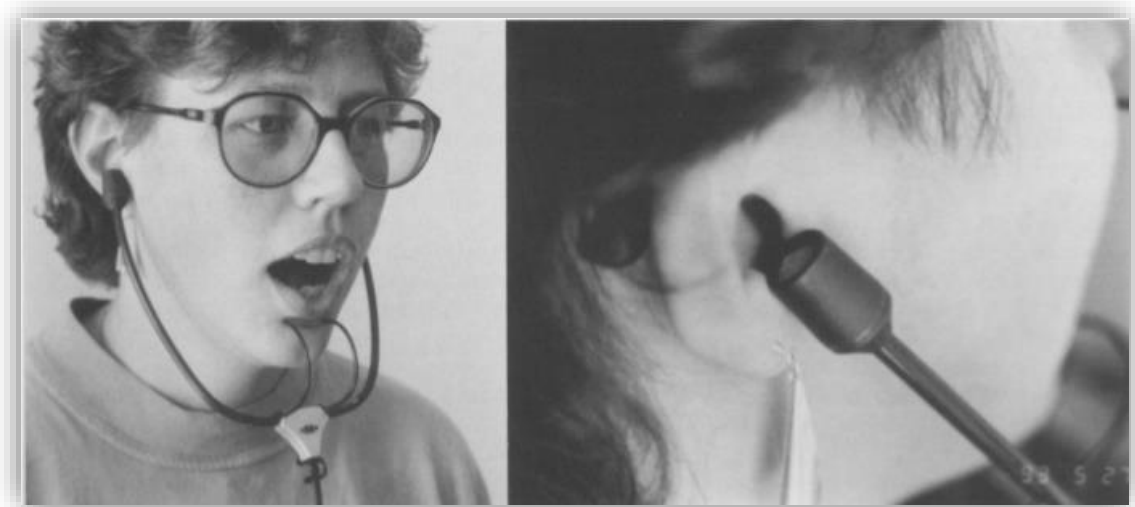
Figure 15 Example of how binaural microphones were worn in the experiment conducted by Ternstrom
