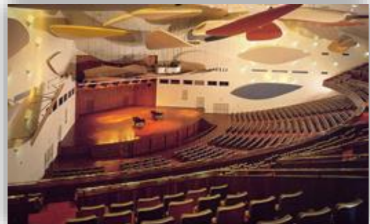
Figure 24 Lecture hall (Caracas). Distinctive feature of the room: "flying saucers". Fan-shaped with a curved roof and a rear wall with its center of curvature in the back of the stage. To solve the problems of echo and lack of uniformity in sound distribution, reflective panels have been added to cover a surface equal to 70% of the ceiling. Thanks to the sculptor Alexander Calder these are not just rectangular panels, but "flying saucers"
