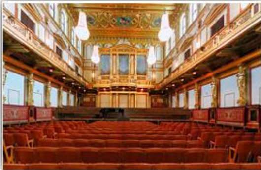
Figure 23 Grosser Musik Vereinsaal (Vienna). The side walls are irregular due to 40 windows, 20 doors above the balconies and 32 female statues below. Thanks to the poor width and the interrupted surfaces, the immediate reflected sound reaches each place.
