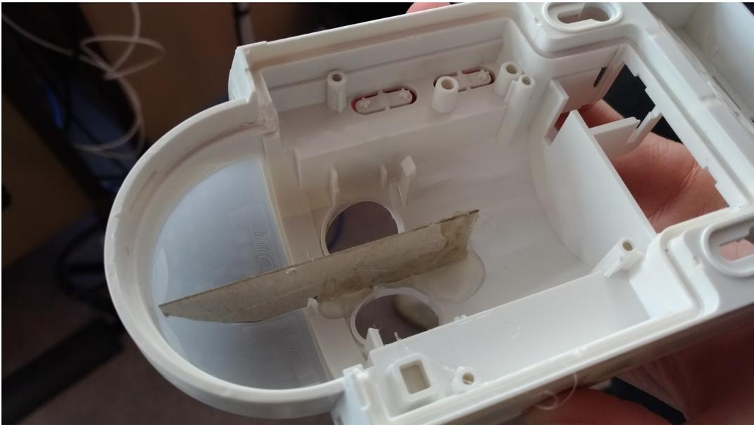
FIGURE 6.1: Applied mask in order to better separate the two detection zones.
